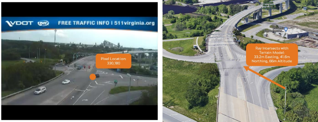
Figure 9. A pixel location shown in the camera view at the left is projected through the ray shown at the right until it intersects the terrain at the location shown. The right image is a screenshot of Google Earth in the area around the traffic camera. The origin of the ray is the location of the traffic camera.
