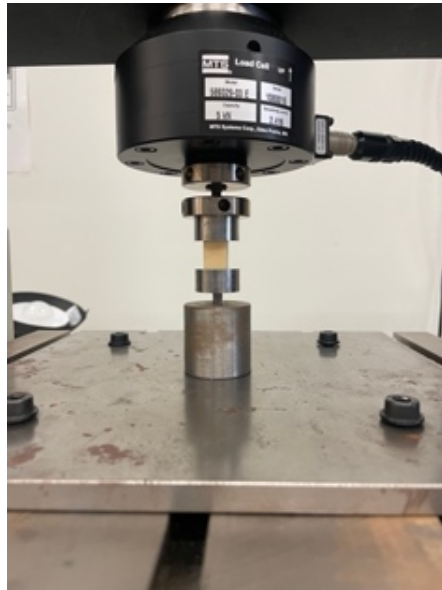
Figure 15: A standard platen compression testing setup for a bone specimen.
