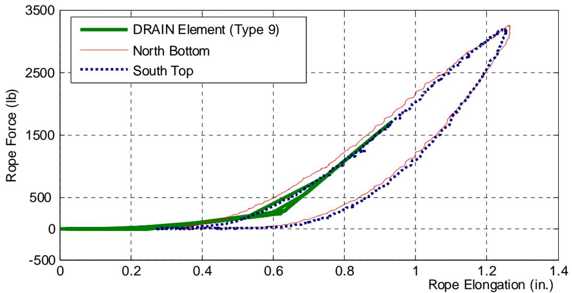
Figure 5. 1: DRAIN Rope Element Response vs. 0.25-in. Rope Response
