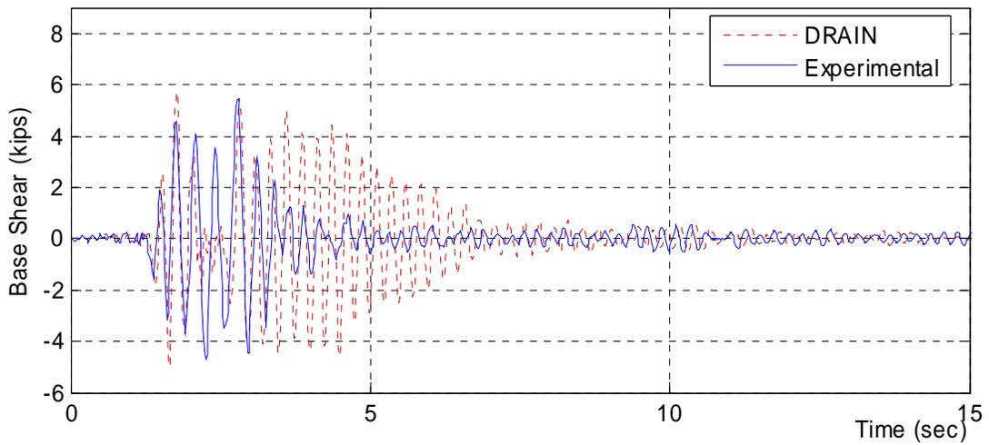
Figure 5. 35: Experimental Base Shear: NR-1-180
