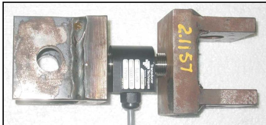
Figure 5. 23: Photographs of Load-Cell Fixtures Attached to the Load Cell
