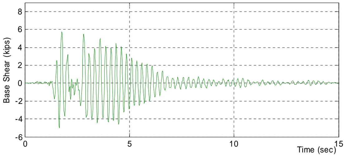
Figure 5. 7: DRAIN Base Shear: NR-1-180
