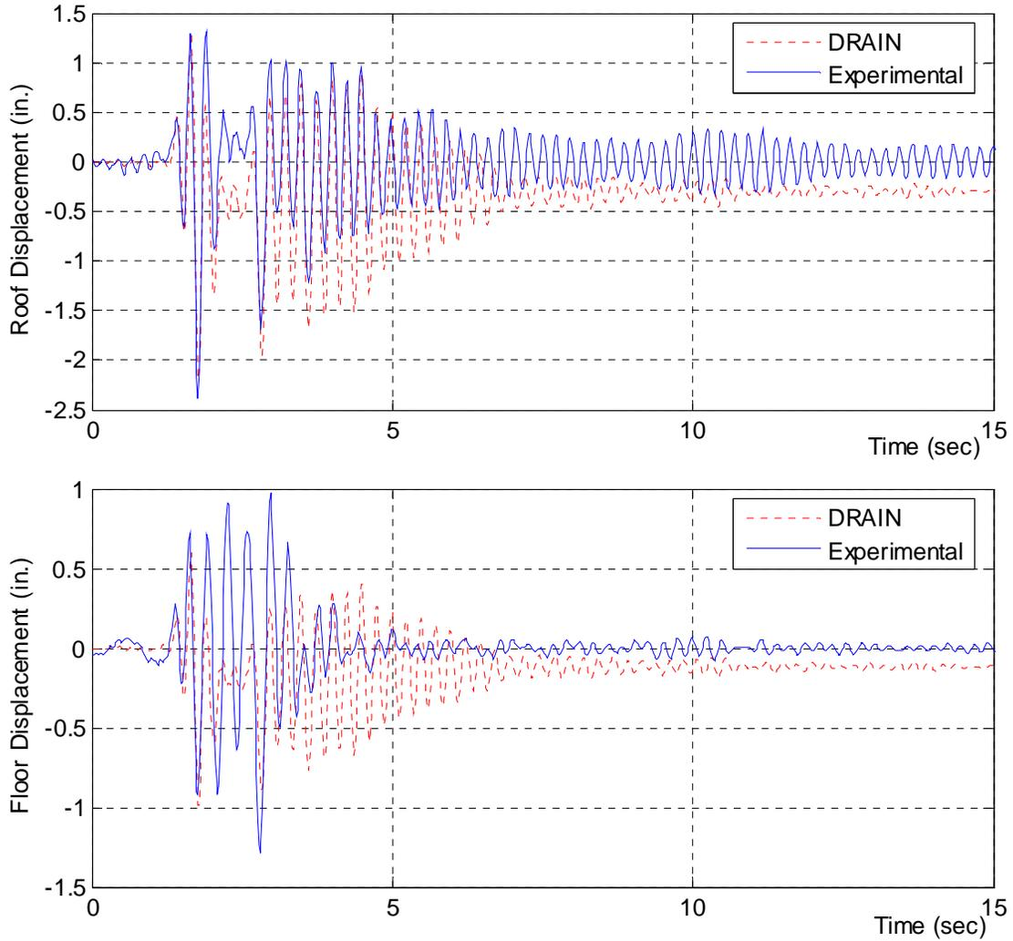
Figure 5. 33: Experimental Roof and Floor Displacements: NR-1-180
