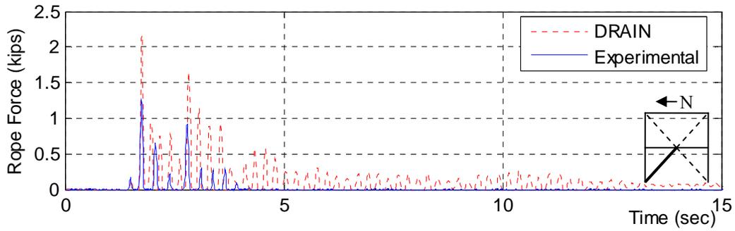
Figure 5. 46: Experimental Rope Force: North Bottom
