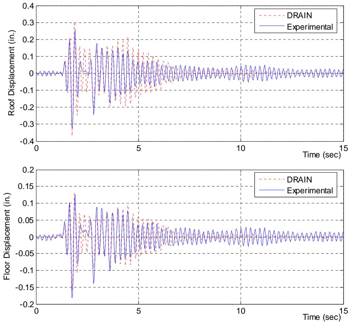
Figure 5. 30: Experimental Roof and Floor Displacements: NR-1-30
