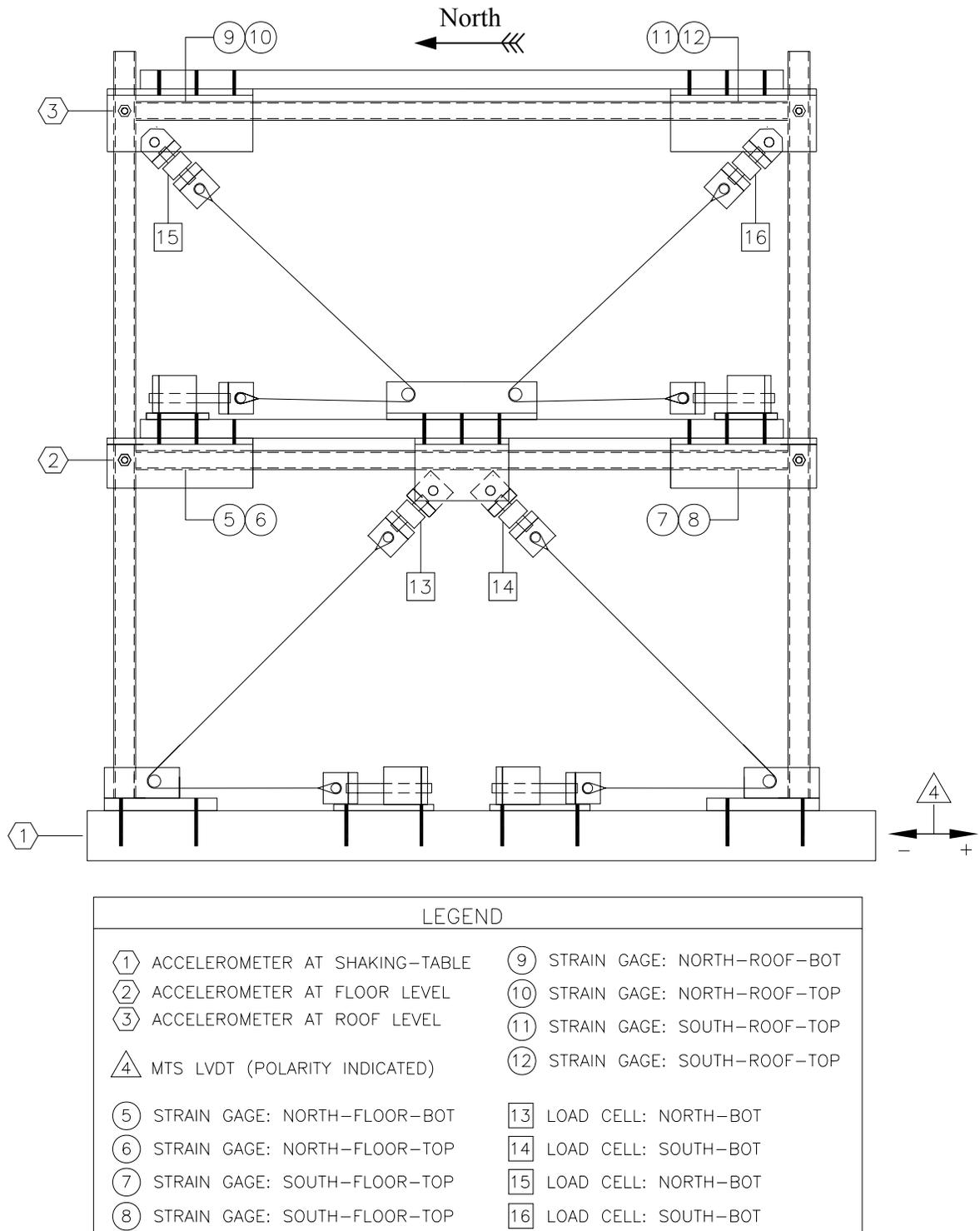
Figure 5. 16: Instrumentation Diagram for Northridge Shaking-Table Tests
