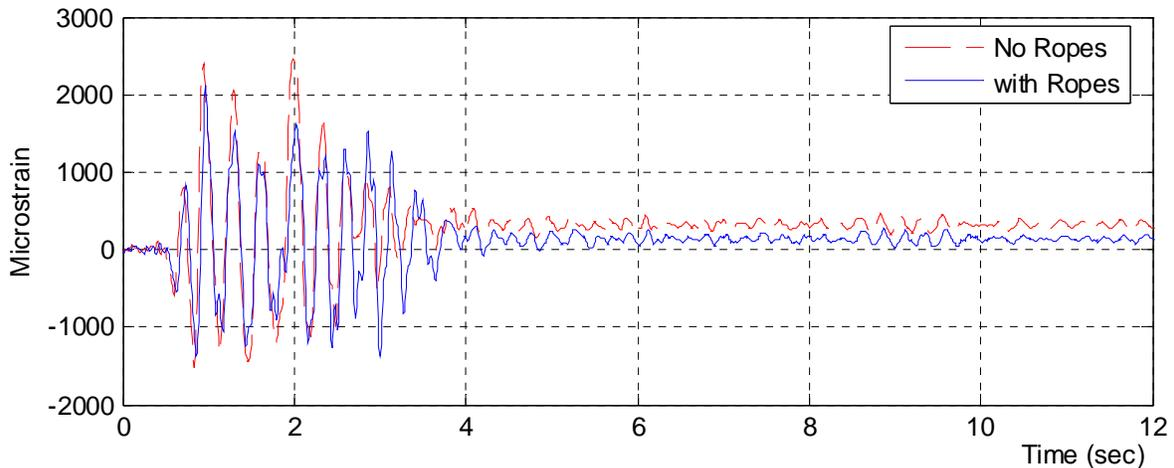
Figure 5. 54: Strain Comparison at North-Roof-Bottom: NR-1-180 and NR-2-180
