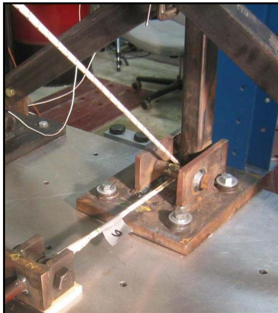
Figure 5. 27: Photograph of Rope Support at the Shaking Table Level
