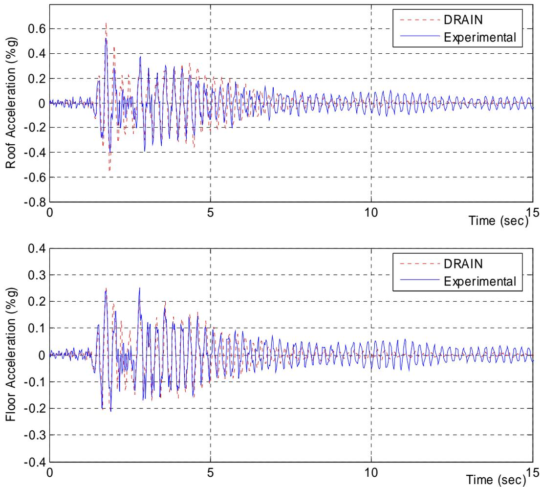
Figure 5. 31: Experimental Roof and Floor Acceleration: NR-1-30
