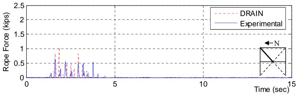
Figure 5. 48: Experimental Rope Force: North Top
