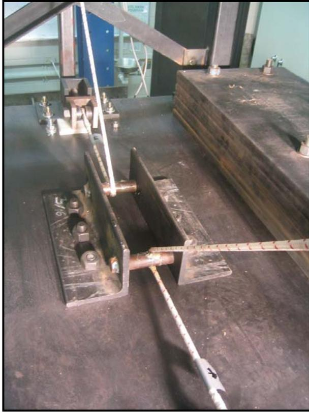
Figure 5. 26: Photograph of Rope Support at the Floor Diaphragm
