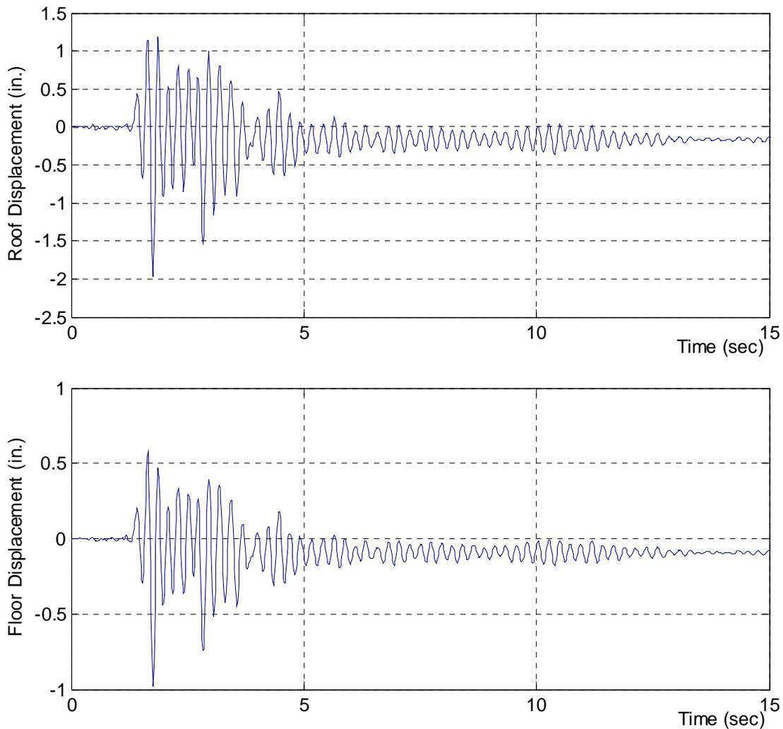
Figure 5. 12: DRAIN Roof and Floor Displacements: NR-2-180
