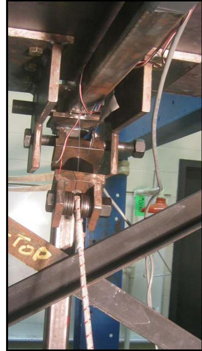
Figure 5. 24: Photograph of Load Cell Attachment at the Roof Diaphragm
