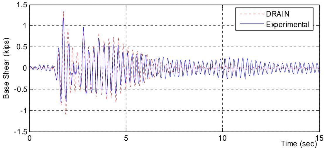
Figure 5. 32: Experimental Base Shear: NR-1-30
