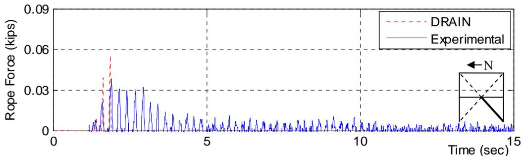
Figure 5. 40: Experimental Rope Force: Bottom South
