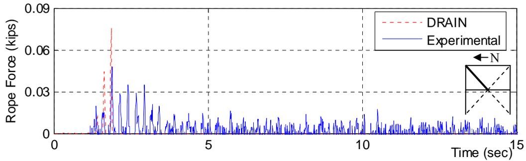
Figure 5. 42: Experimental Rope Force: Top North
