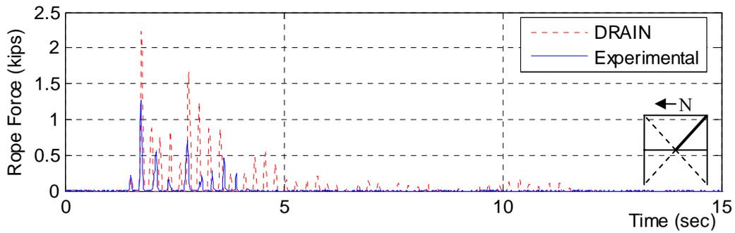
Figure 5. 49: Experimental Rope Force: South Top
