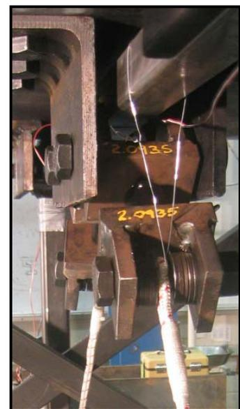
Figure 5. 25: Photographs of Load-Cell Attachment at the Floor Diaphragm
