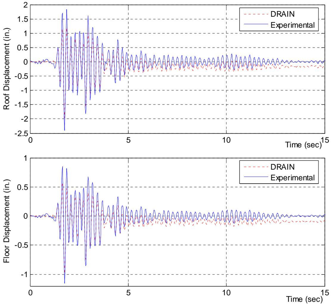
Figure 5. 43: Experimental Roof and Floor Displacements: NR-2-180
