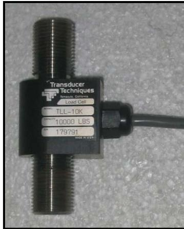
Figure 5. 17: Photograph of 10,000-lb Tension Load Cells
