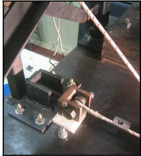
Figure 5. 28: Photographs of Adjustment Fixture at the Floor Diaphragm
