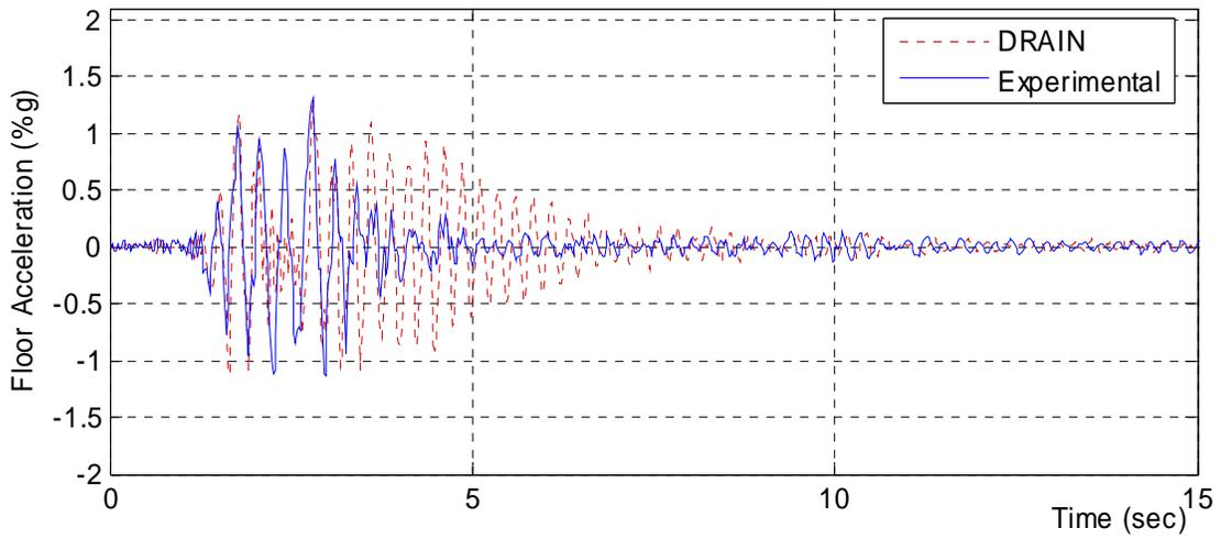
Figure 5. 34: Experimental Roof and Floor Accelerations: NR-1-180
