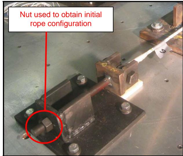
Figure 5. 29: Photographs of Adjustment Fixture at the Shaking Table
