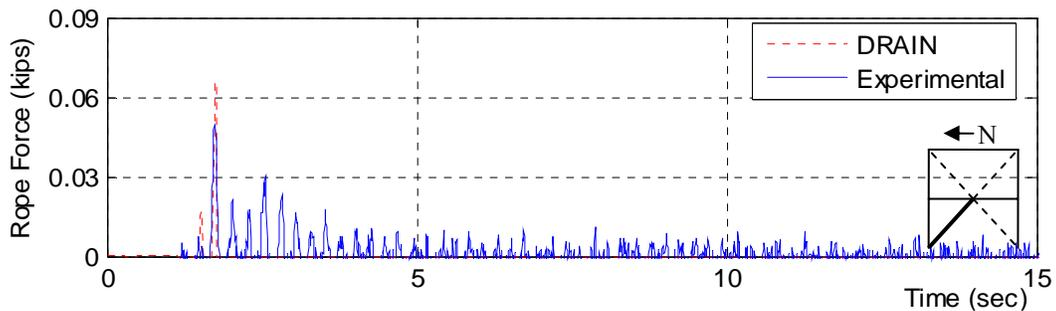
Figure 5. 39: Experimental Rope Force: Bottom North
