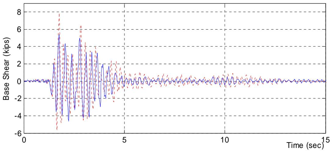
Figure 5. 45: Experimental Base Shear: NR-2-180
