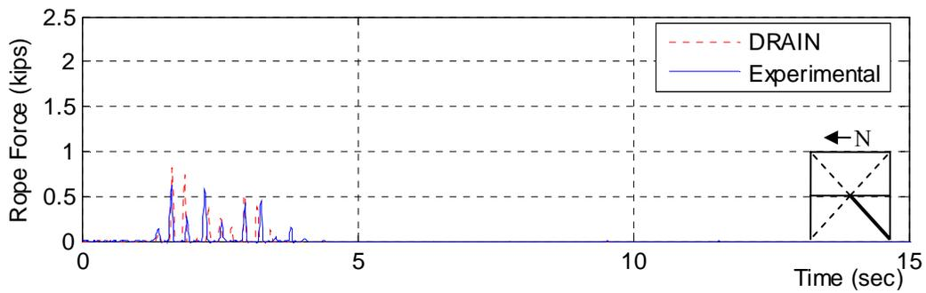
Figure 5. 47: Experimental Rope Force: South Bottom
