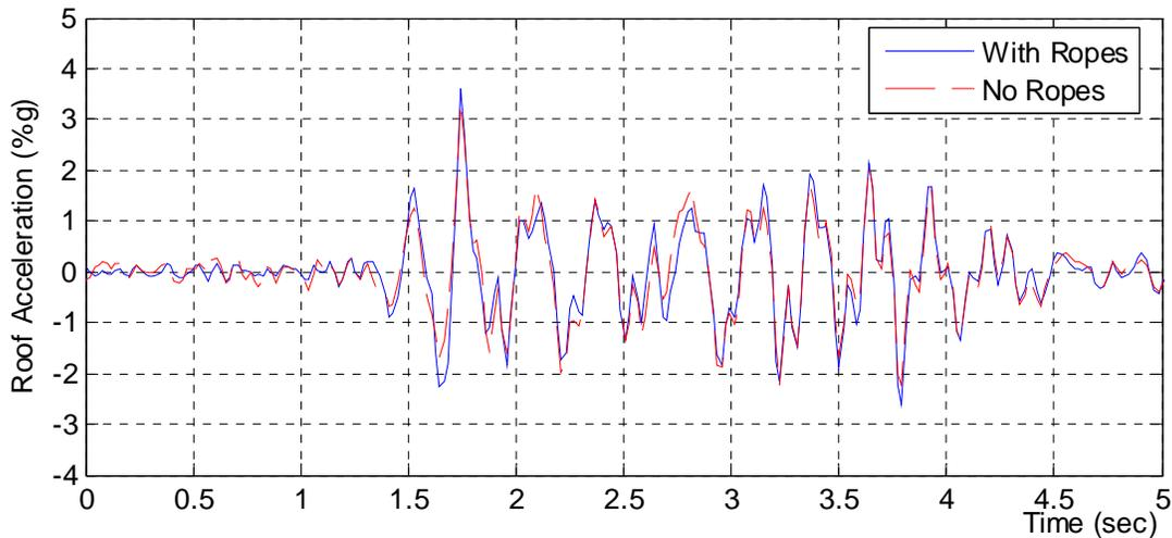
Figure 5. 57: Comparison of Roof Acceleration between 0 and 5 sec: NR-1-180 and NR-2-180
