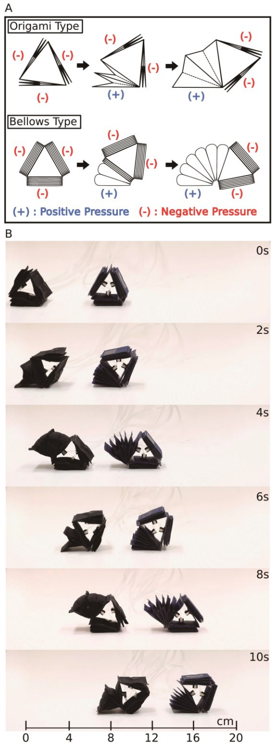
Figure 2.15. (A), Diagrams of the two methods of constructing the revolving robot. (B), Photos showing the two rolling robots in operation.
