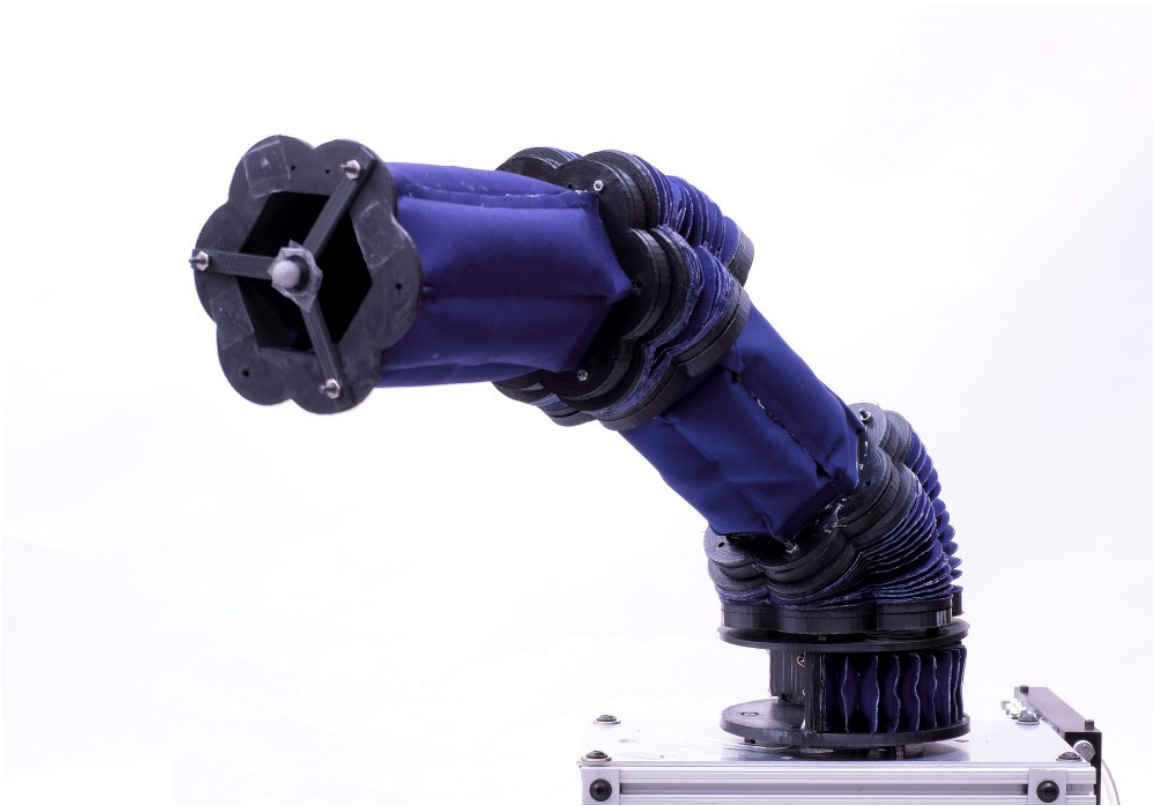
Figure 3.1. A proposed soft/rigid hybrid pneumatic robot in this paper.
