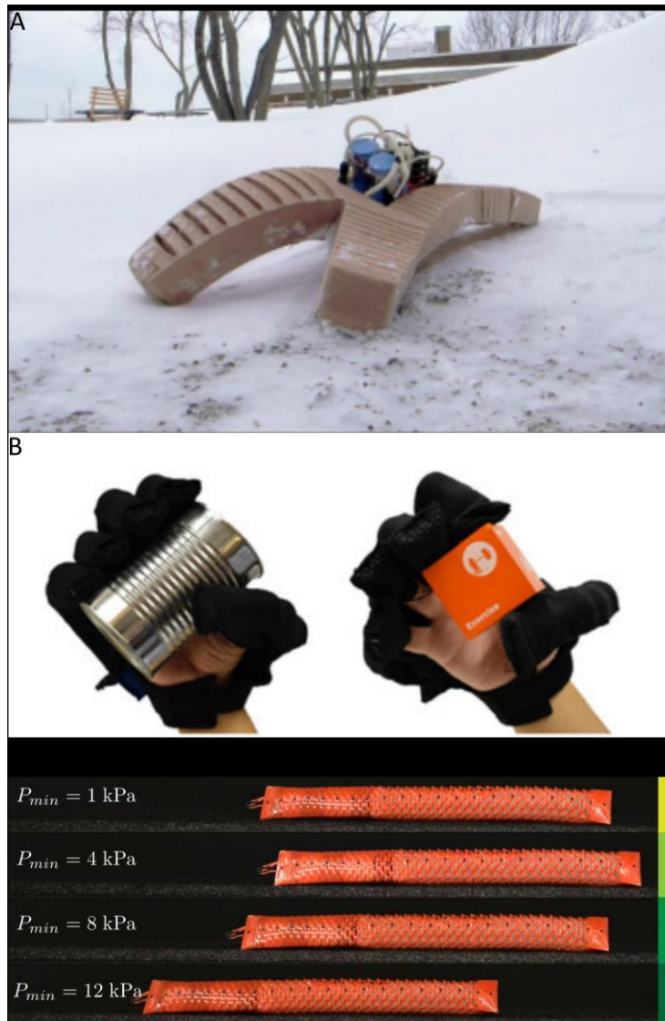
Figure 1.1. (A) A untethered soft robot [3]; (B) A fabric-based soft robotic glove for assistance and rehabilitation [4]; (C) A bioinspired actuator with kirigami skins [5].
