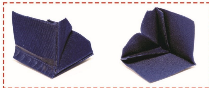
Figure 2.7. (A-C), Examples of airtight corners. (D), Example of a corner that is not airtight.
