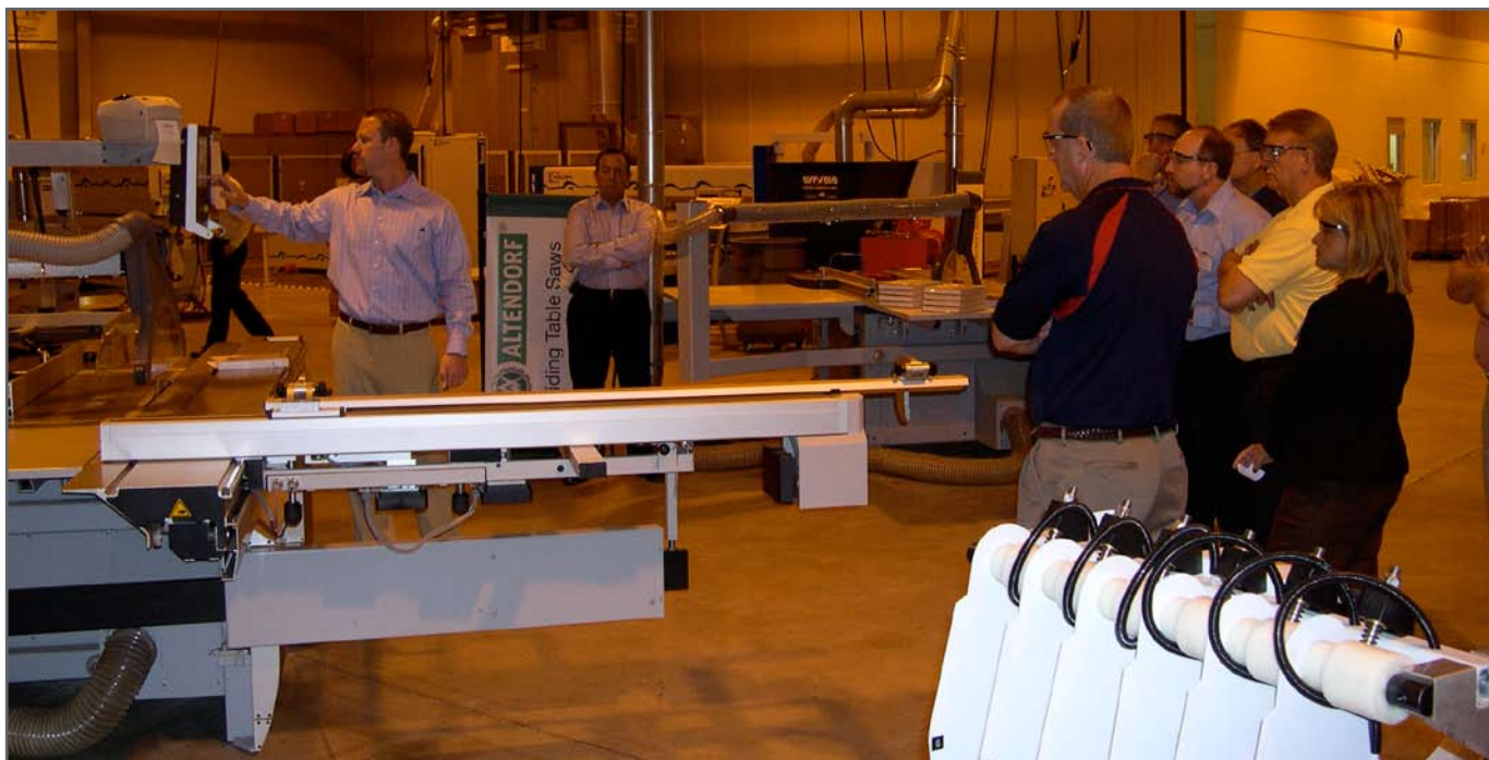
Chris Dolbow of Stiles demonstrates the new Altendorf Sliding Table Saw – the F45 ELMO. This has to be the sleekest, most sophisticated table saw in the marketplace with its nearly hands-off operation.
