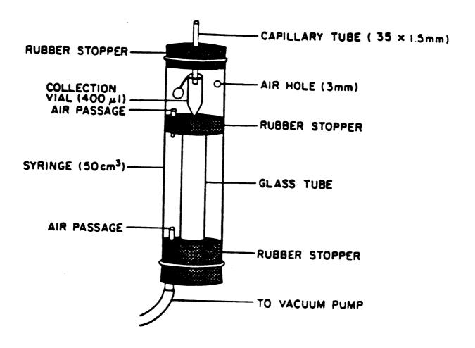
Figure 1. Diagrammatic representation of device used to obtain milk samples for somatic cell count determination.
