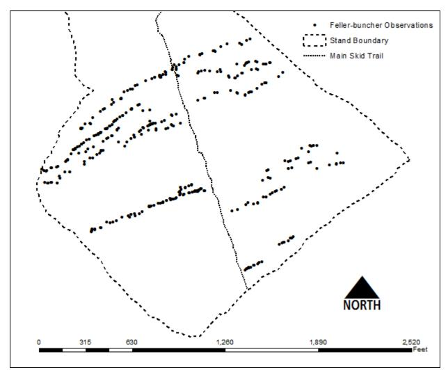
Figure 3.1. Logged GPS waypoints of feller-buncher cycle locations on case study site located in the Virginia Coastal Plain region
