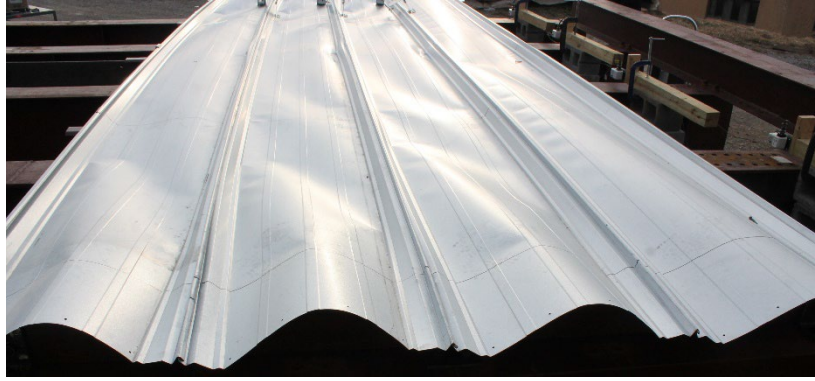
Figure 6-15 Typical deformed shape after panel buckling (from Specimen 7)
