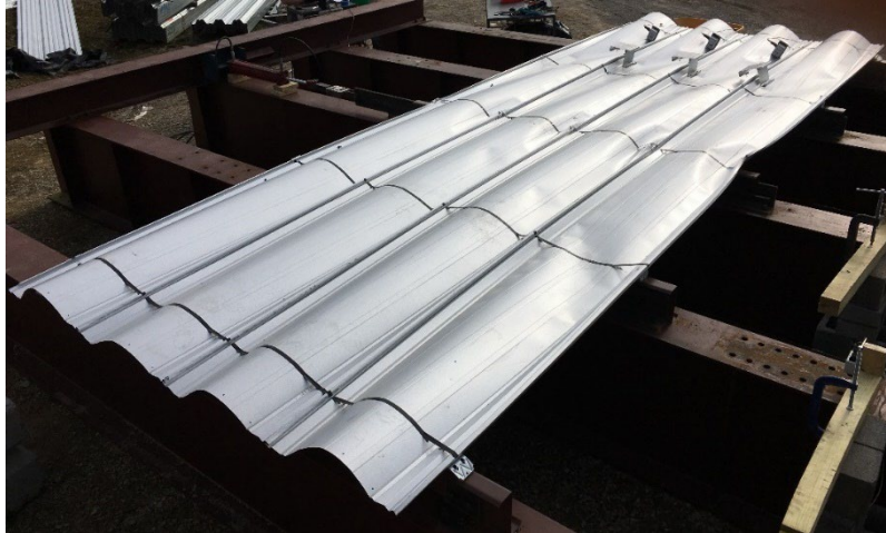
Figure B-3 Deformed shape of Specimen 1
