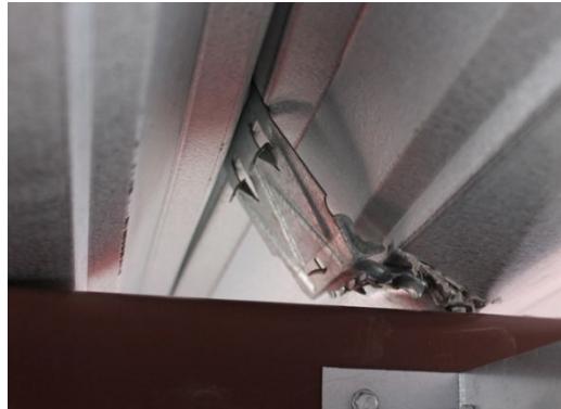
Figure 6-17 Tearing of clip material at the bottom (from Specimen 7)
