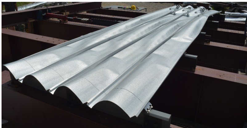
Figure B-23 Deformed shape of Specimen 6
