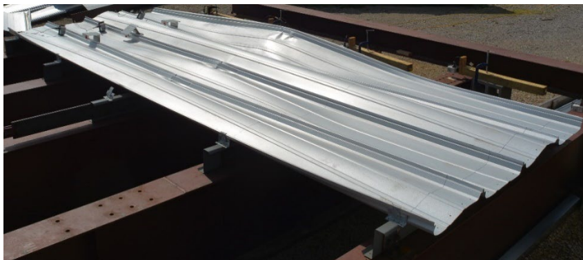
Figure B-11 Deformed shape of Specimen 3
