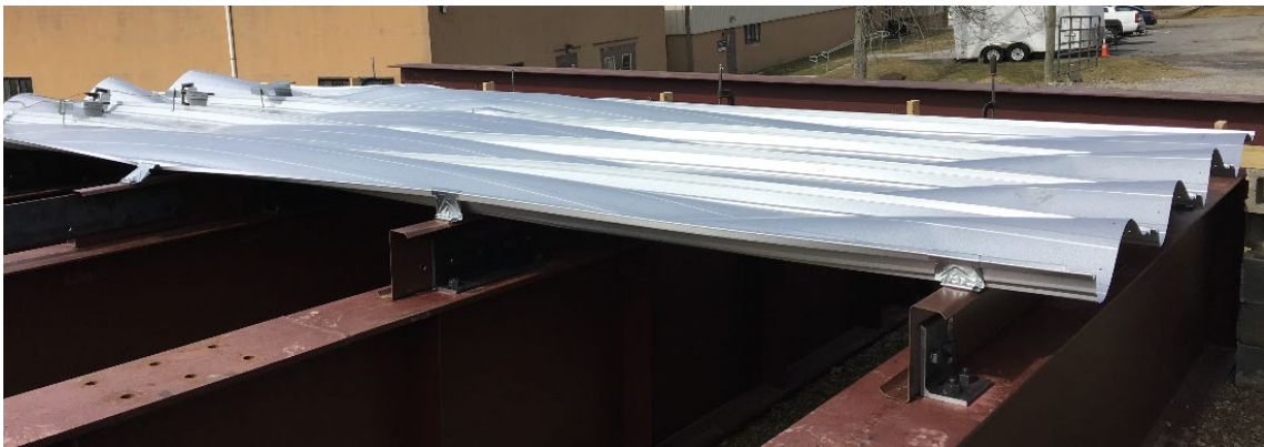
Figure B-7 Deformed shape of Specimen 2
