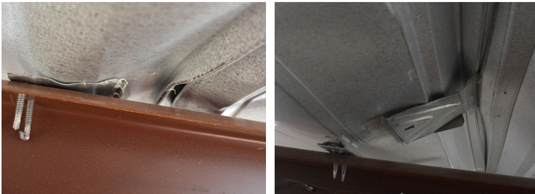
Figure 6-16 Mechanical detachment of clips from top (left) and bottom (right) (from Specimen 8)
