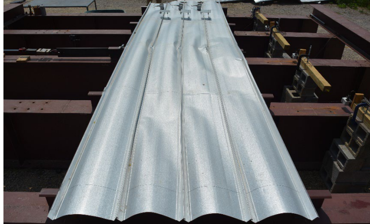
Figure B-15 Deformed shape of Specimen 4
