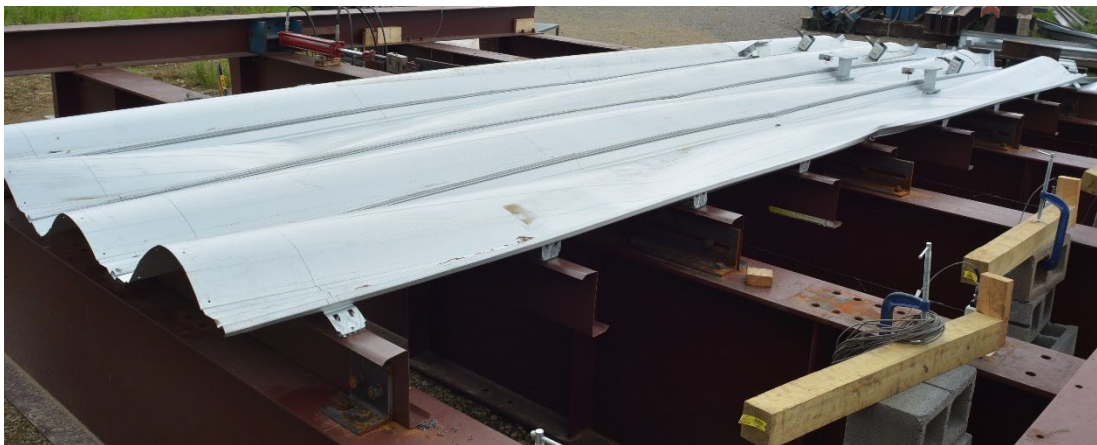
Figure B-43 Deformed shape of Specimen 11
