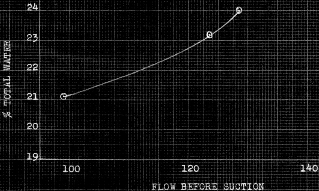
Flow - Before and After Curves of Line Putty-Cement Sand Mortar Used in Proposal V
