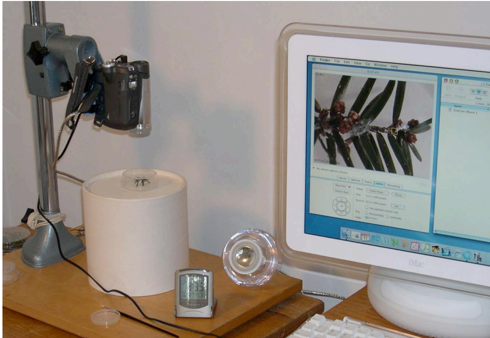
Figure 4.1. Experimental arena for the video studies. Each assay consisted of a 5 x 2.5 cm polystyrene Petri dish lined with moistened filter paper, and held 10 cm of branch clippings of eastern hemlock, T. canadensis , infested with A. tsugae . A digital video camera, mounted on a camera stand 5-10 cm above the assay was used for video capture. All intermittent video capture was controlled using EvoCam 3.5 software and video segments were visualized and stored on an Apple iMac G4 computer.
