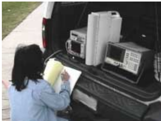
Figure C.2: Photo of TX and RX LMDS Radio Module field testing.
