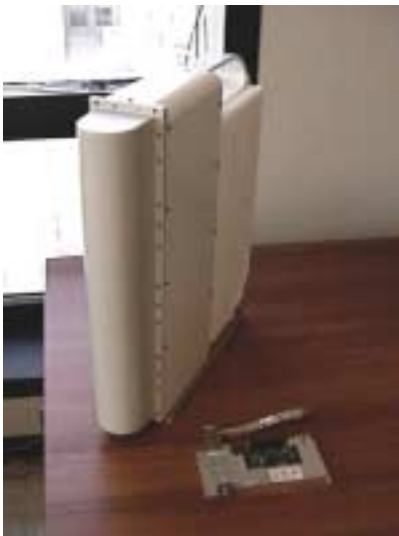
Figure C.6: Photo of RX LMDS Radio Module.
