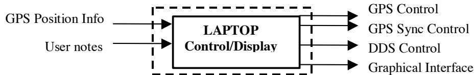
Figure A.1: TX Host Module interface diagram
