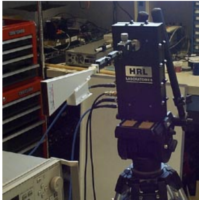
Figure 25: The transmitter horn antenna.
