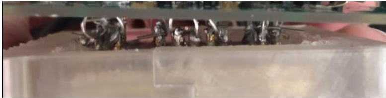
Figure 52: The additional leads to connect the \text{Si}_3\text{N}_4 switching cell to the interface board.
