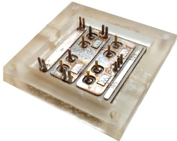
Figure 47 : a) 3D rendering of the switching cell with housing, and b) cross-section view showing the two-step encapsulation.
