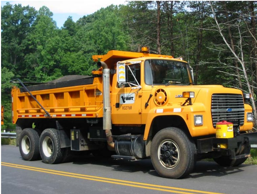
Figure 3.7: VDOT Dump Truck used for Live Load Testing
