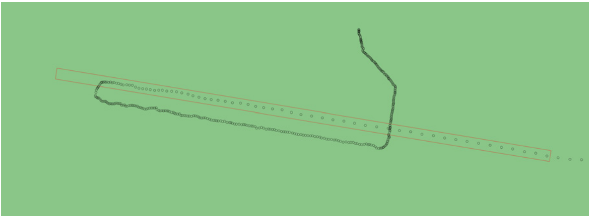
Figure 3.6: Illustration of a Runway Polygon and Arrival Track Points for an Arrival at San Diego International Airport
