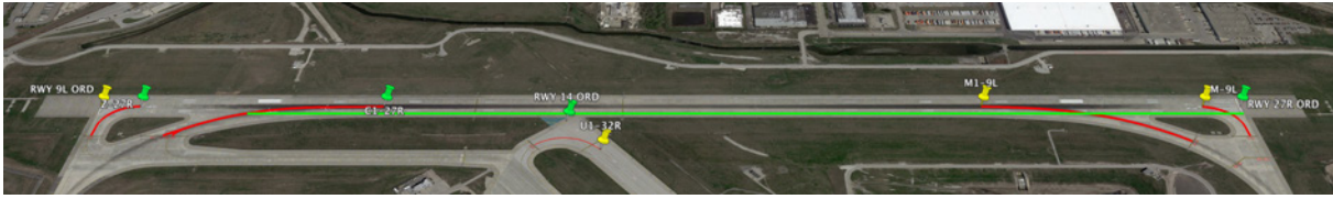
Figure 3.10: Image of Straight-Line Distance from Runway Threshold to Intersection of Taxiway Centerline and Runway Edge at Chicago O’Hare International Airport Runway 9R-27L. Source: Google Earth
