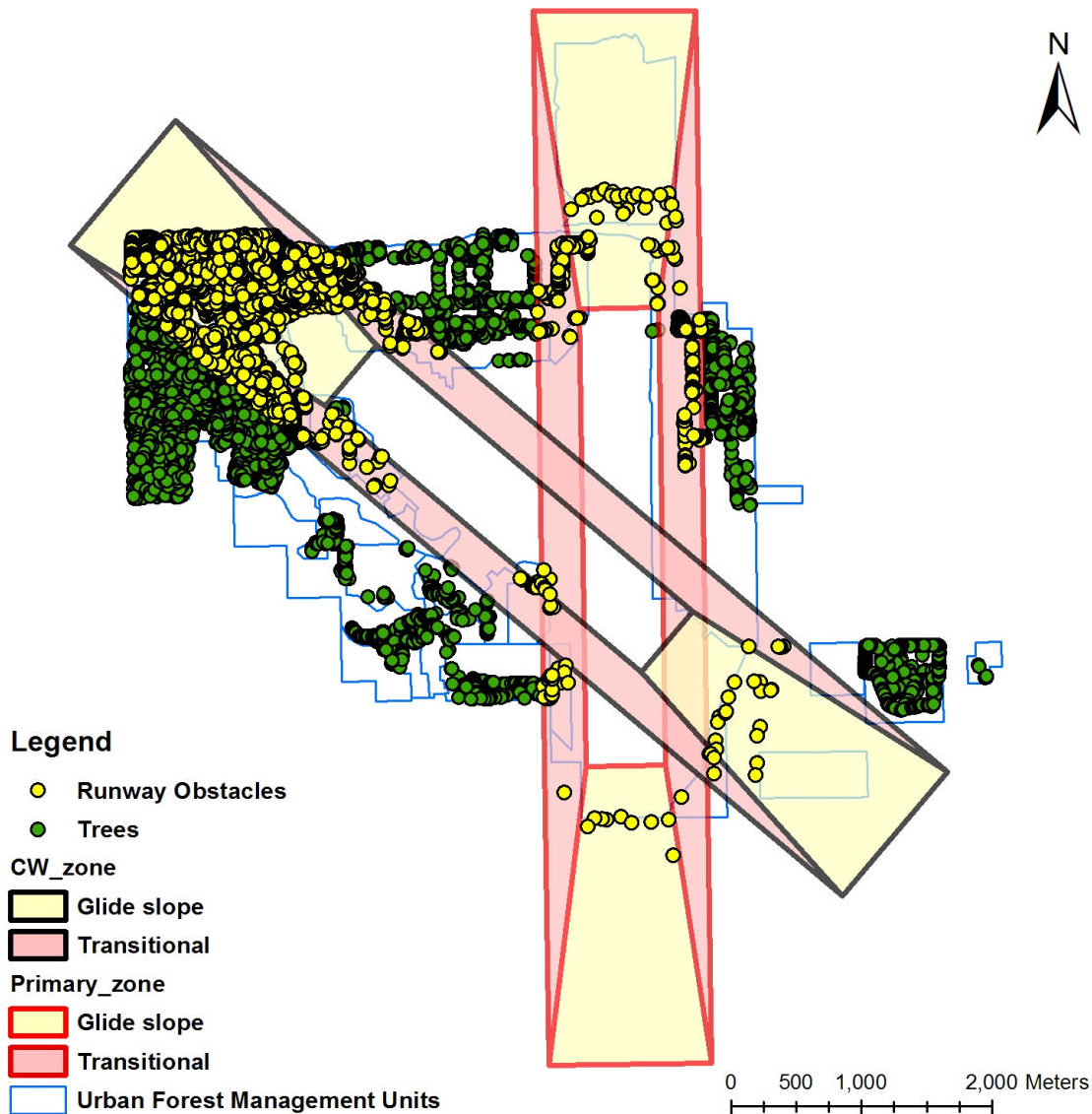
Figure 12: Trees within the glide slope and transitional zones around the runways were identified as possible runway obstacles and were measured first during the inventory.
