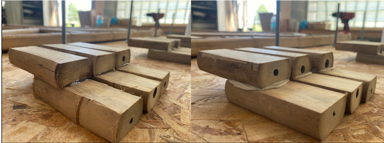
Figure 28. Test specimens for adhesive shear test. (left) 2-part epoxy samples. (right) Expanding construction adhesive samples. (not featured) PVA wood glue samples.
