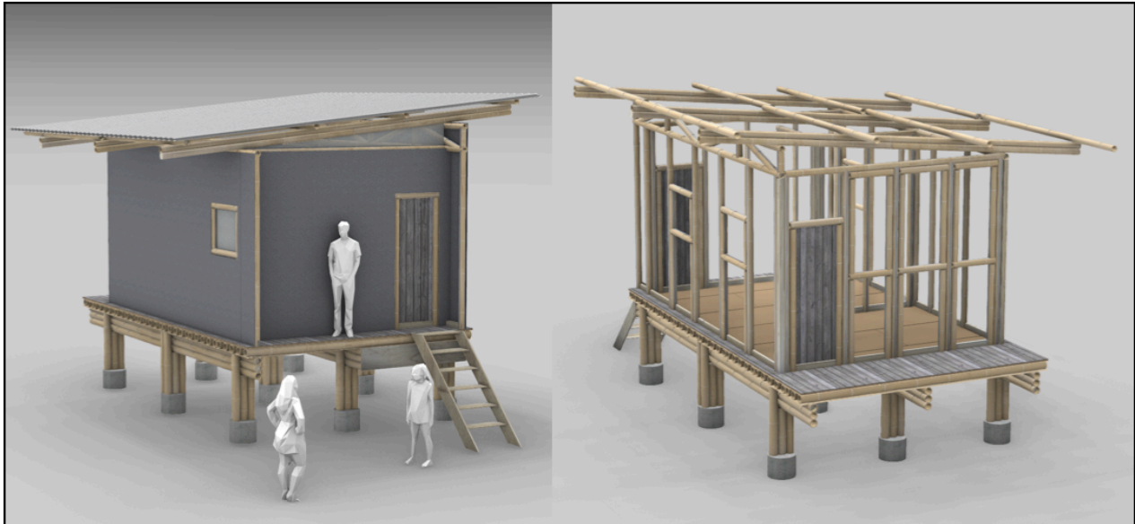
Figure 30. Case Study House Design. (shown both with and without the fiber cement board sheathing)
