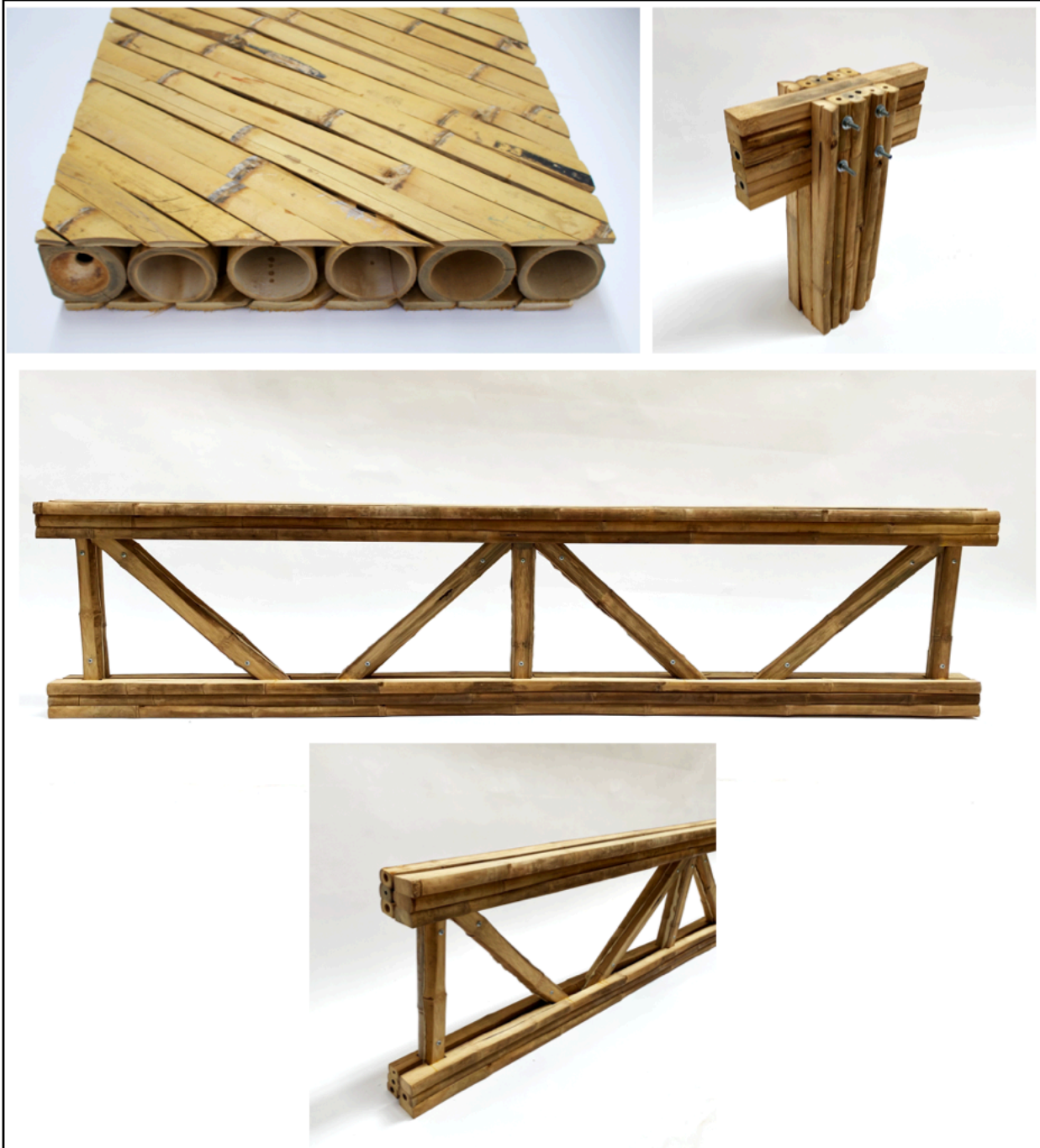
Figure 24. Prototypes from RDF. (top left) G. angustifolia 2' x6' panel. (top right) Column to beam connection. (middle) Dendrocalamus strictus truss. (bottom) Truss side view showing the two halves.
