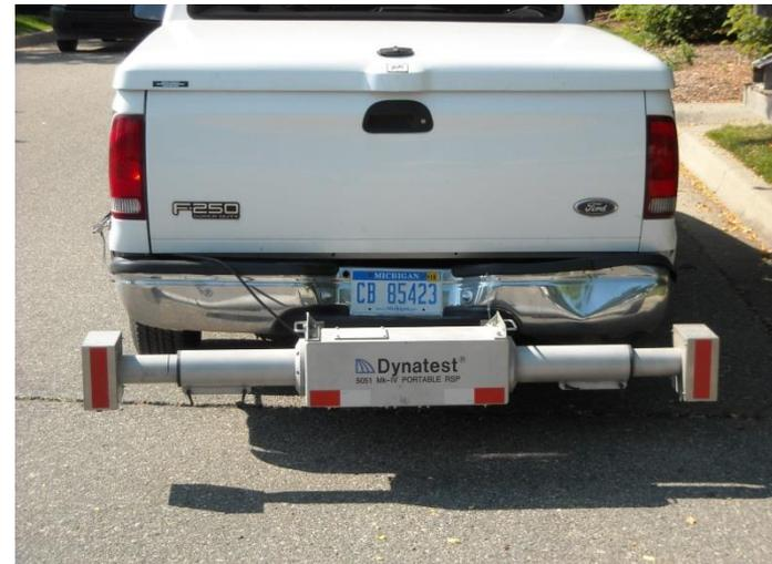
Sensor Spacing = Distance between left and right wheel path sensors
