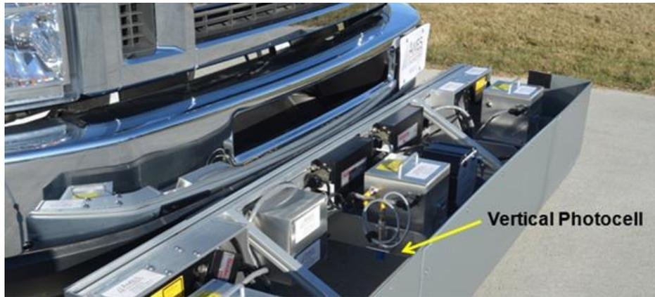
Vertical: Triggers off reflective tape placed on the pavement
