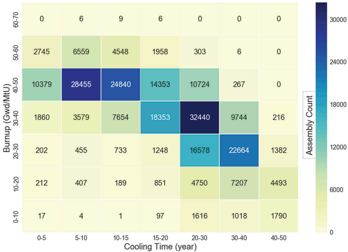
Figure 8.1 Inventory of SNF discharged from U.S. commercial reactors through June 2013, from UDB (Unified Database), binned by burnup and cooling time. Cooling time was calculated on July 1, 2016 [7]
