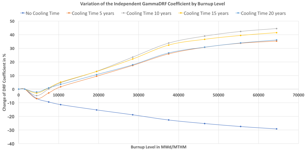
Figure G.7 Sensitivity of the Photon Source DRF Coefficient to Burnup and Cooling Time - 1
