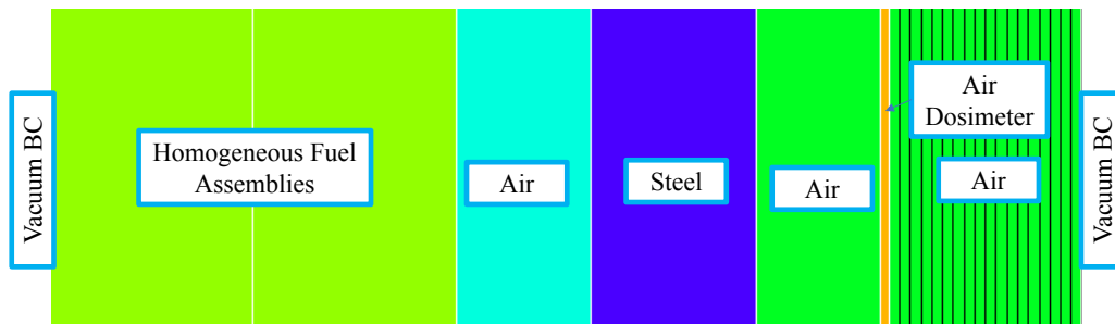
Figure H.1 PENTRAN TM 1D Photon Importance Model
