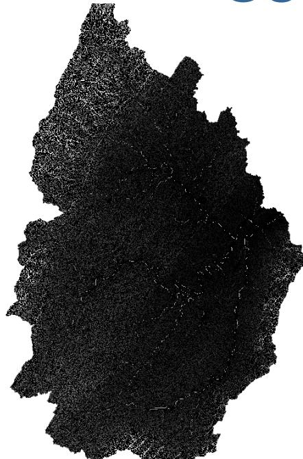
A map showing flow accumulation values, where darker shades indicate higher accumulation areas, typically along stream networks.
