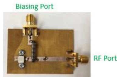
Figure 3.6 Board for characterizing of varactor
