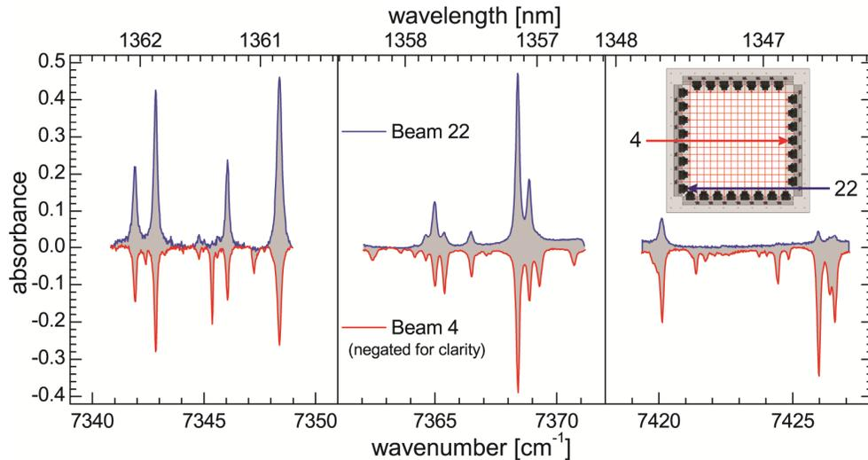
Fig. 4. Absorption spectra measured during a single scan of the TDM 3-FDML laser operating at 50.24337 kHz (~20 microseconds). Each panel shows the spectra measured by one of the three FDML lasers.
