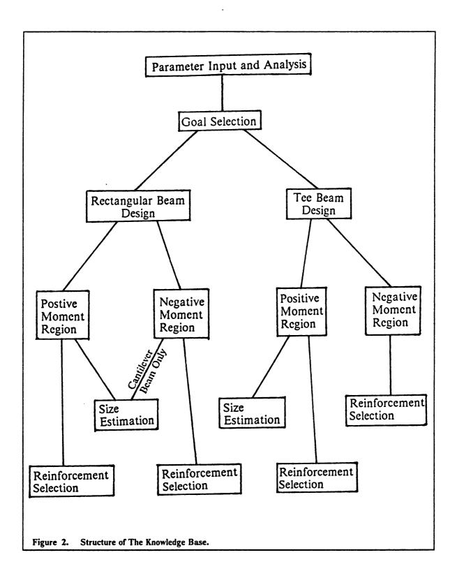
the goal is either to design a rectangular or a tee beam. A goal menu is provided for the user to choose a goal if he knows which one to choose. If not, four rules are provided so that BEAMDES will be able to determine the goal by itself. If the beam is a cantilever then it is designed as a rectangular section. For other boundary conditions, if the slab is reinforced concrete and cast monolithically with the beam then the beam is designed as a tee beam, otherwise, a rectangular beam is designed.
