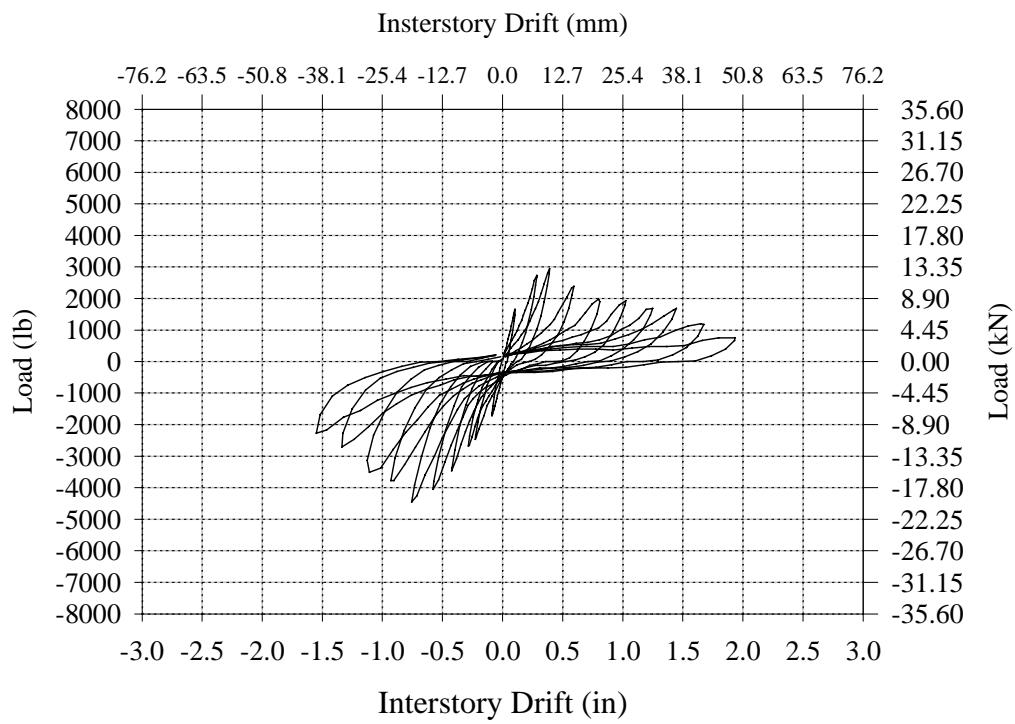
**Figure B.23 – Stabilized Hysteresis Curve for Wall CC-1.**
