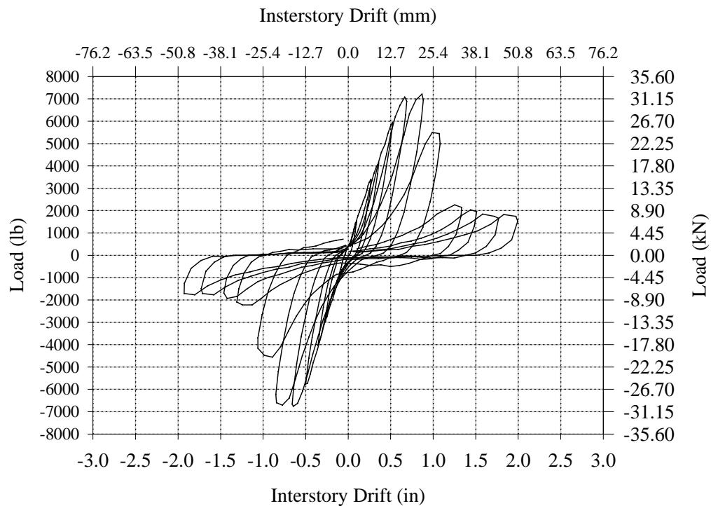
**Figure B.42 – Initial Hysteresis Curve for Wall EC-2.**
