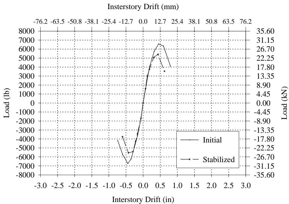
**Figure B.32 – Cyclic Envelope Curve for Wall DC-1.**
