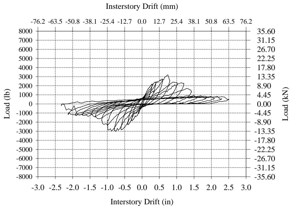
**Figure B.2 – Initial Hysteresis Curve for Wall AC-1.**
