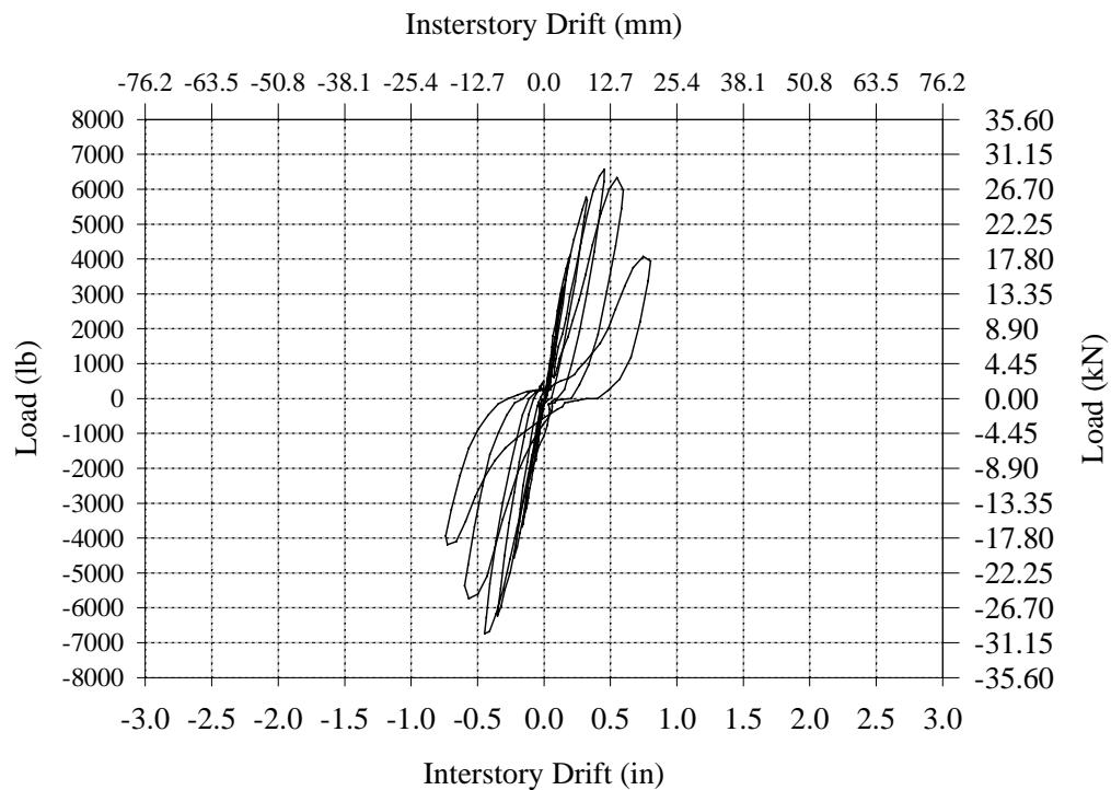
**Figure B.30 – Initial Hysteresis Curve for Wall DC-1.**
