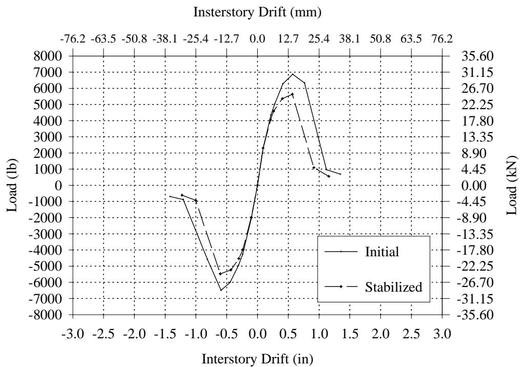
**Figure B.36 – Cyclic Envelope Curve for Wall DC-2.**
