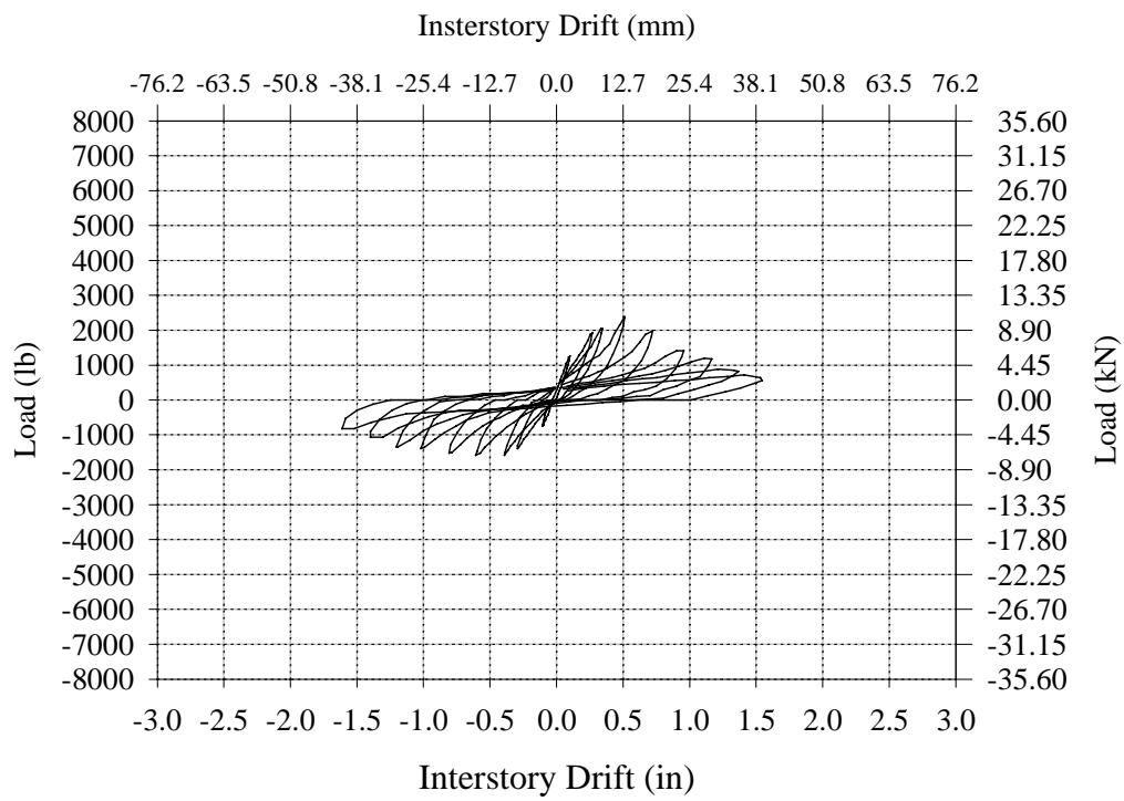
**Figure B.11 – Stabilized Hysteresis Curve for Wall AC-3.**
