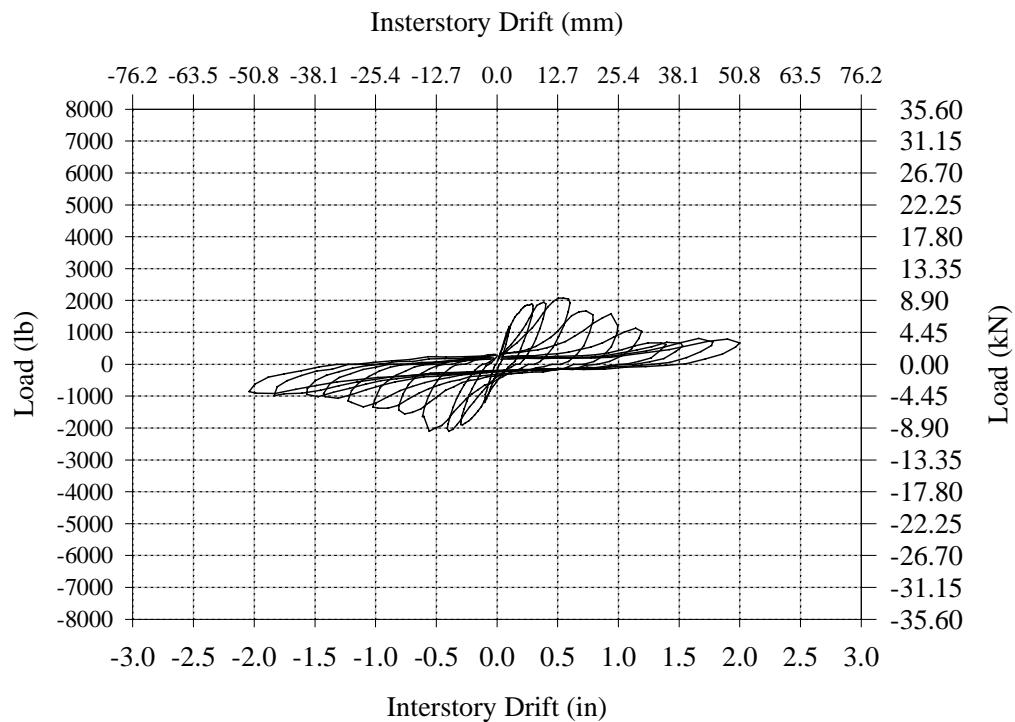
**Figure B.6 – Initial Hysteresis Curve for Wall AC-2.**
