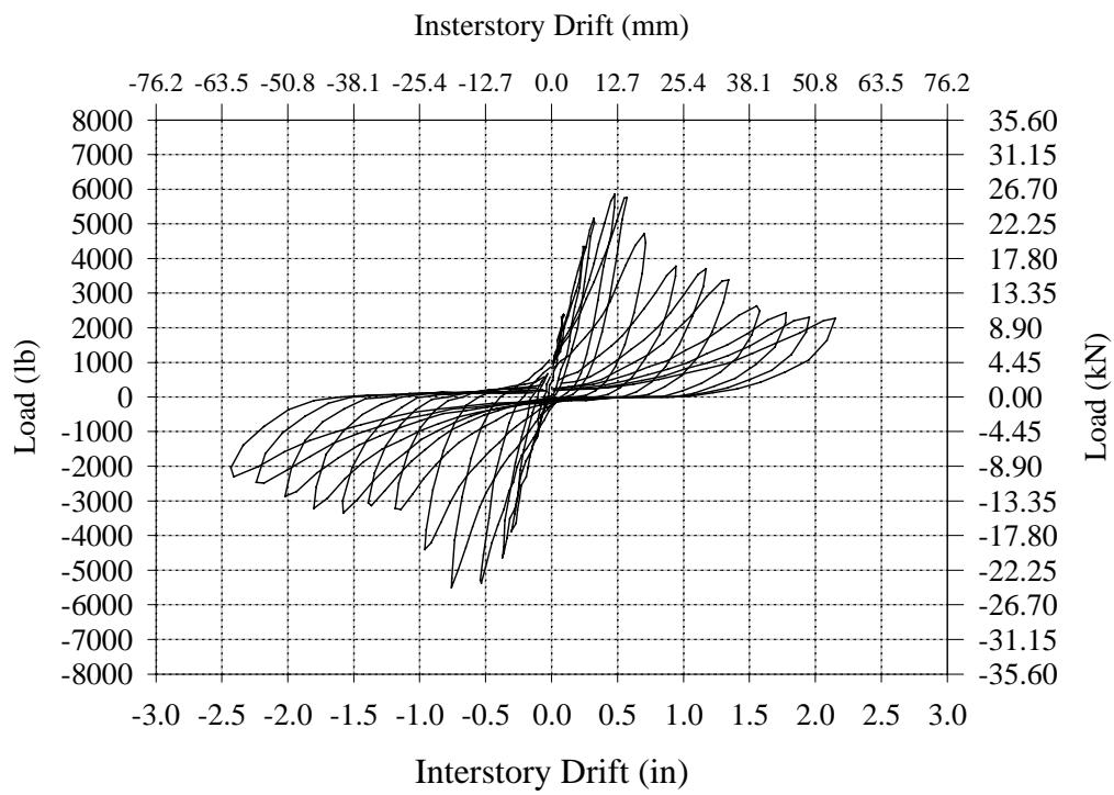
**Figure B.39 – Stabilized Hysteresis Curve for Wall EC-1.**
