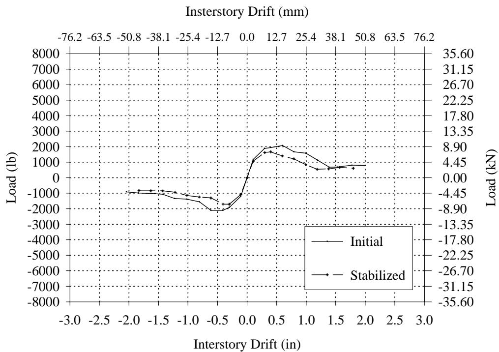
**Figure B.8 – Cyclic Envelope Curve for Wall AC-2.**
