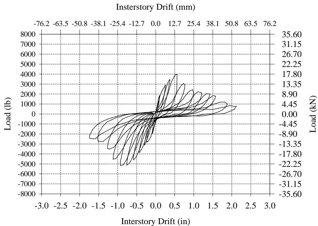
**Figure B.22 – Initial Hysteresis Curve for Wall CC-1.**
