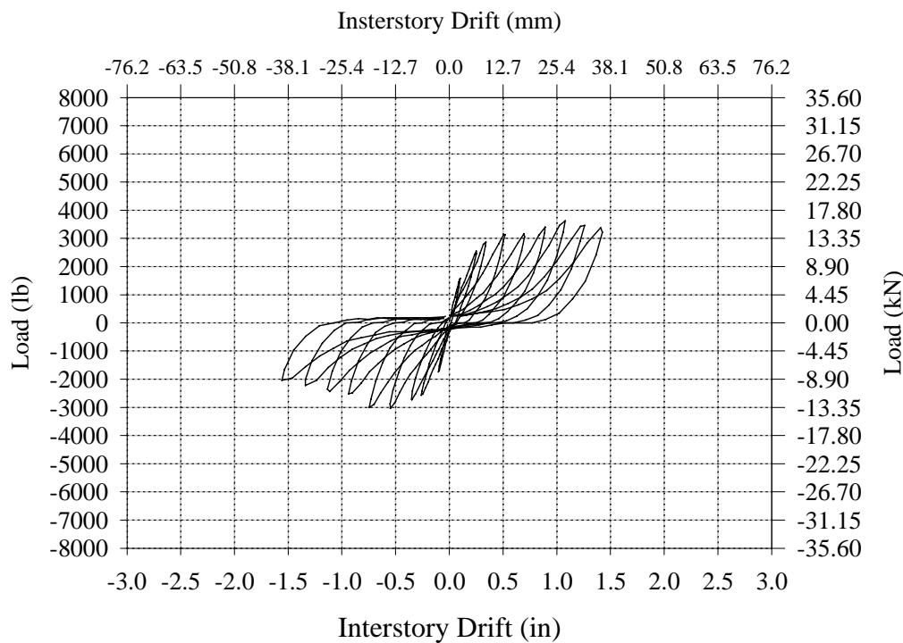
**Figure B.27 – Stabilized Hysteresis Curve for Wall CC-2.**
