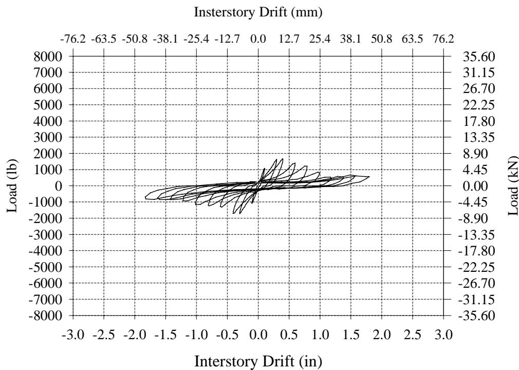
**Figure B.7 – Stabilized Hysteresis Curve for Wall AC-2.**
