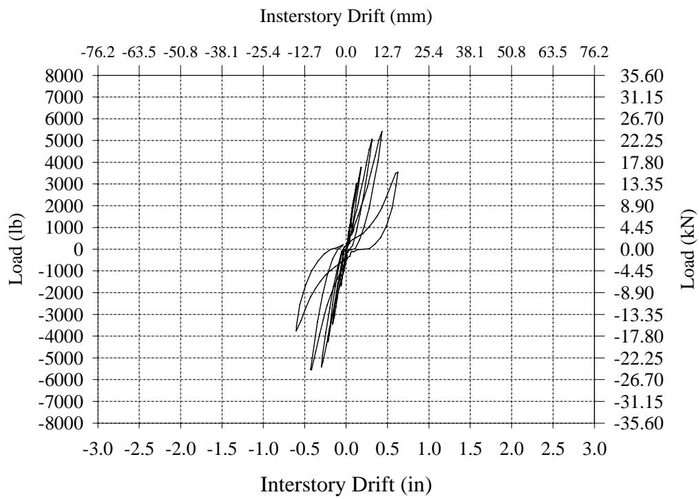
**Figure B.31 – Stabilized Hysteresis Curve for Wall DC-1.**
