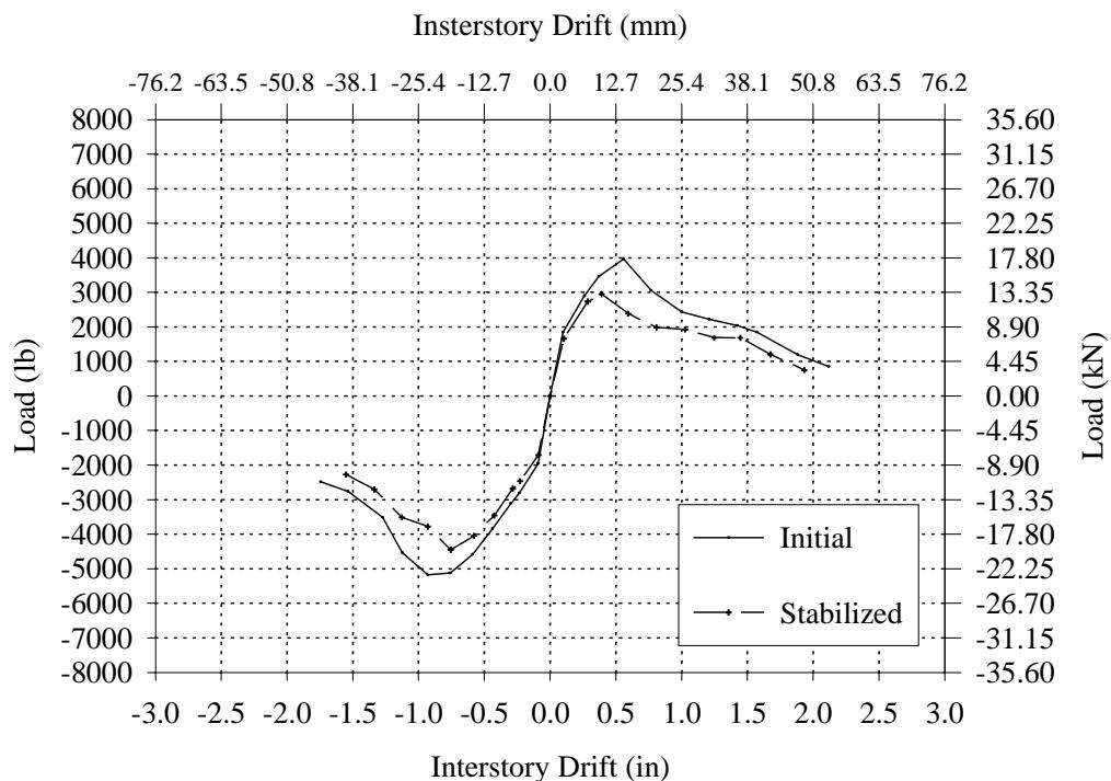
**Figure B.24 – Cyclic Envelope Curve for Wall CC-1.**
