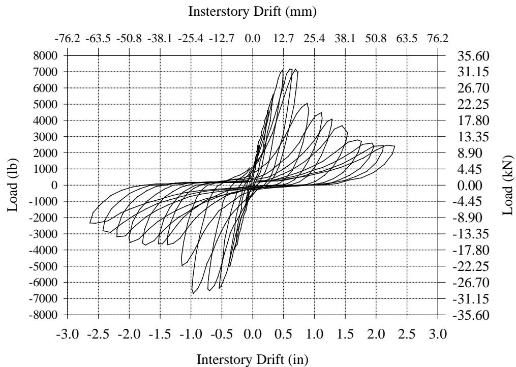
**Figure B.38 – Initial Hysteresis Curve for Wall EC-1.**
