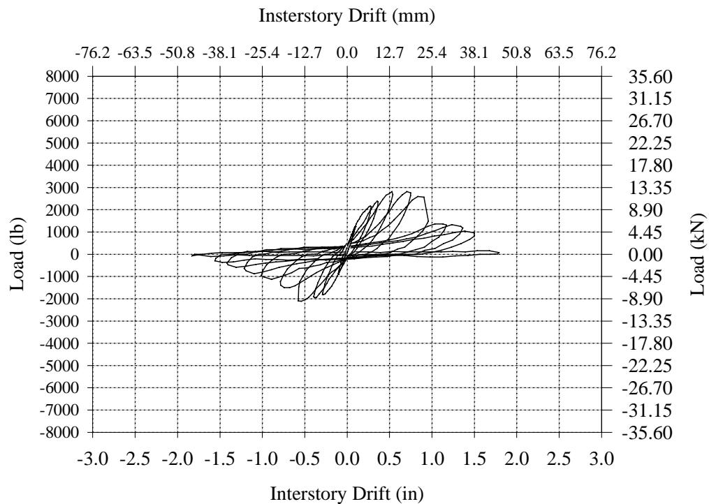
**Figure B.14 – Initial Hysteresis Curve for Wall BC-1.**
