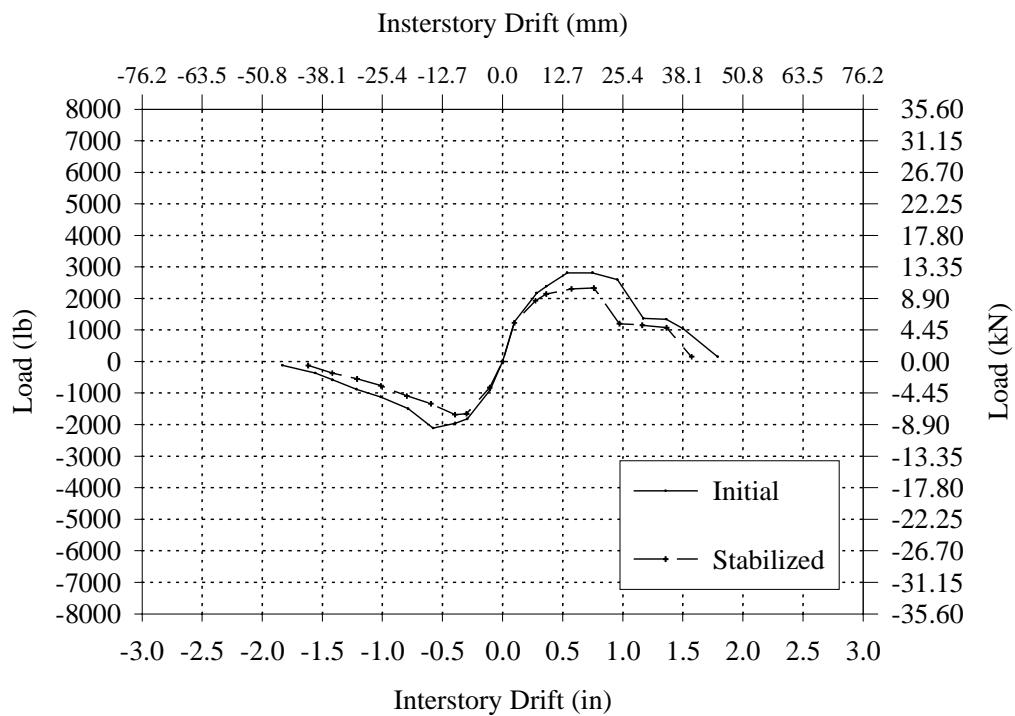
**Figure B.16 – Cyclic Envelope Curve for Wall BC-1.**
