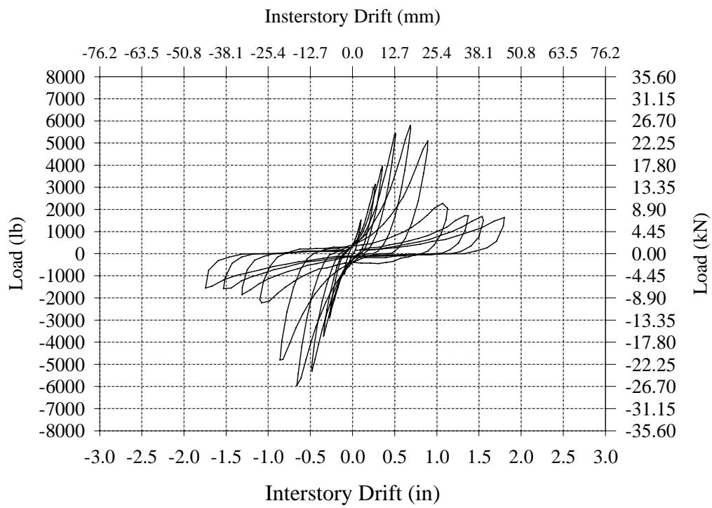
**Figure B.43 – Stabilized Hysteresis Curve for Wall EC-2.**
