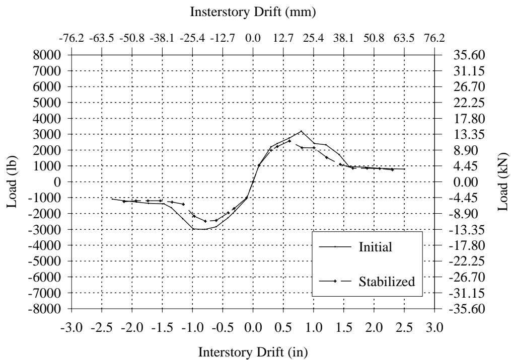
**Figure B.4 – Cyclic Envelope Curve for Wall AC-1.**
