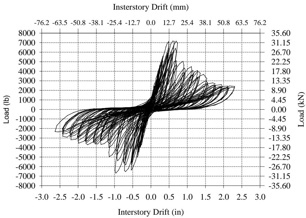
**Figure B.37 – Total Hysteresis Curve for Wall EC-1.**
