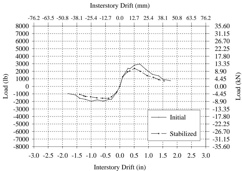
**Figure B.12 – Cyclic Envelope Curve for Wall AC-3.**
