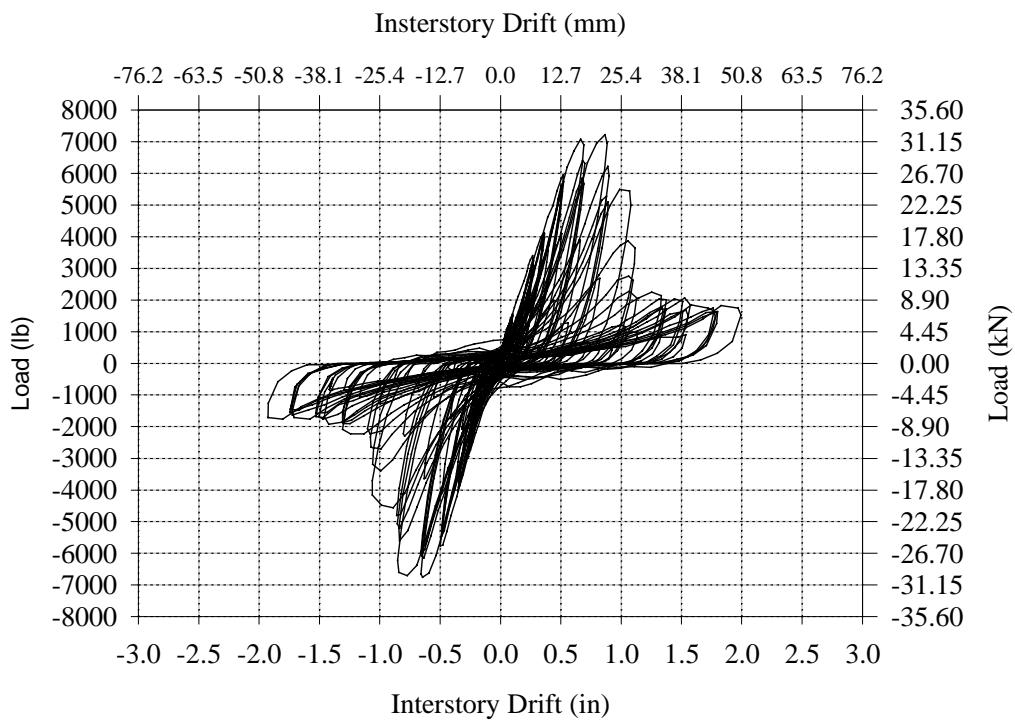
**Figure B.41 – Total Hysteresis Curve for Wall EC-2.**
