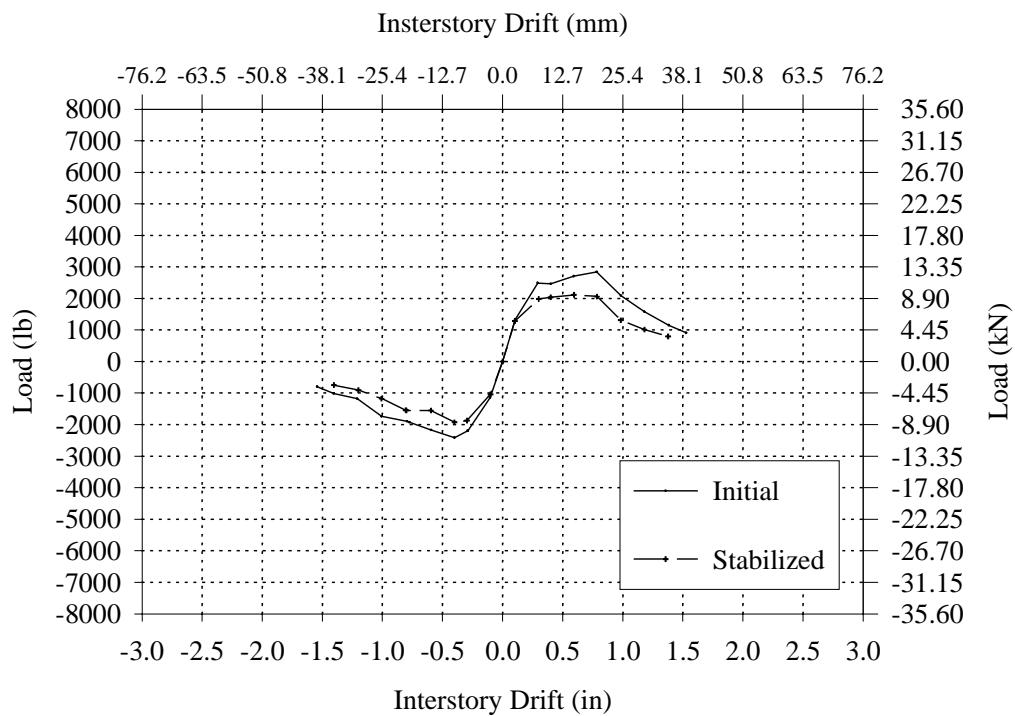
**Figure B.20 – Cyclic Envelope Curve for Wall BC-2.**
