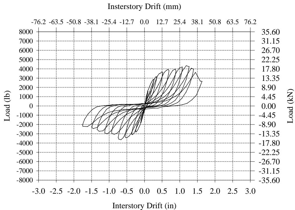
**Figure B.26 – Initial Hysteresis Curve for Wall CC-2.**
