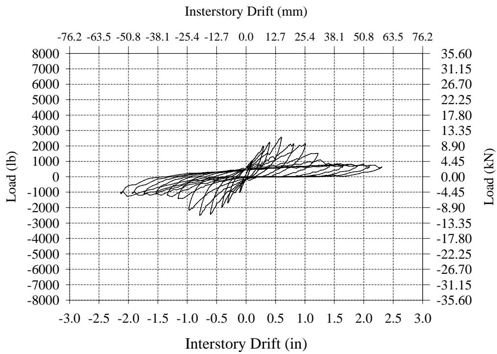
**Figure B.3 – Stabilized Hysteresis Curve for Wall AC-1.**
