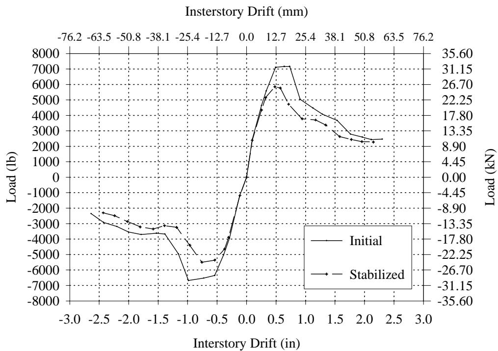
**Figure B.40 – Cyclic Envelope Curve for Wall EC-1.**
