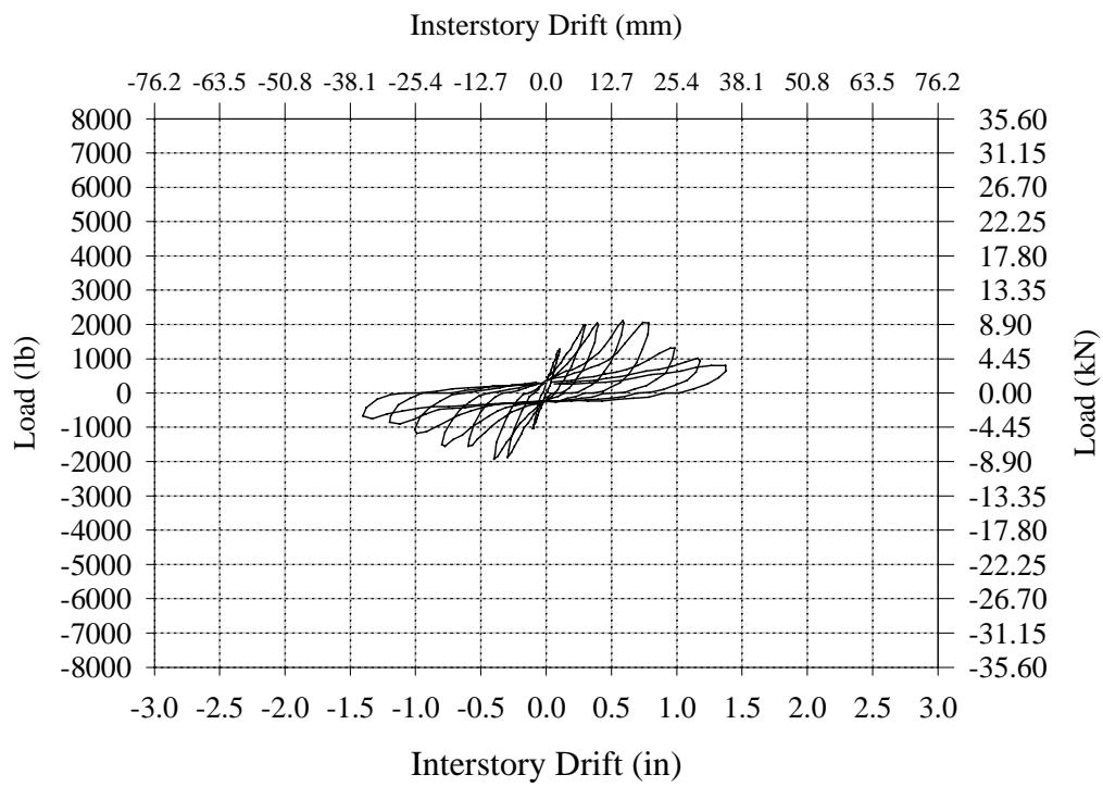
**Figure B.19 – Stabilized Hysteresis Curve for Wall BC-2.**
