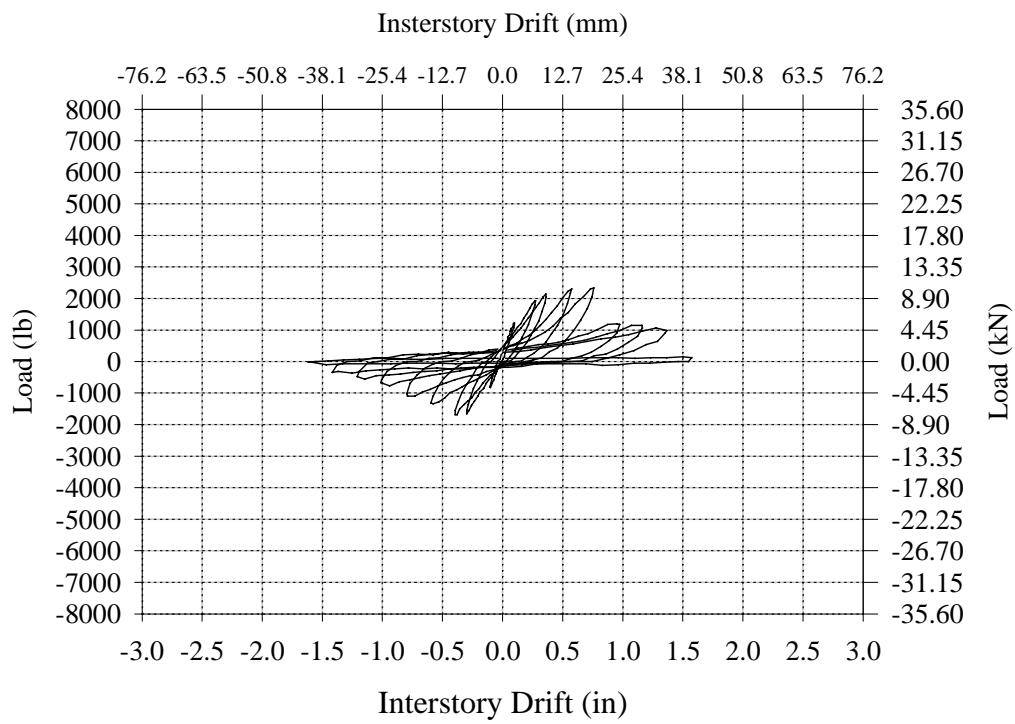
**Figure B.15 – Stabilized Hysteresis Curve for Wall BC-1.**
