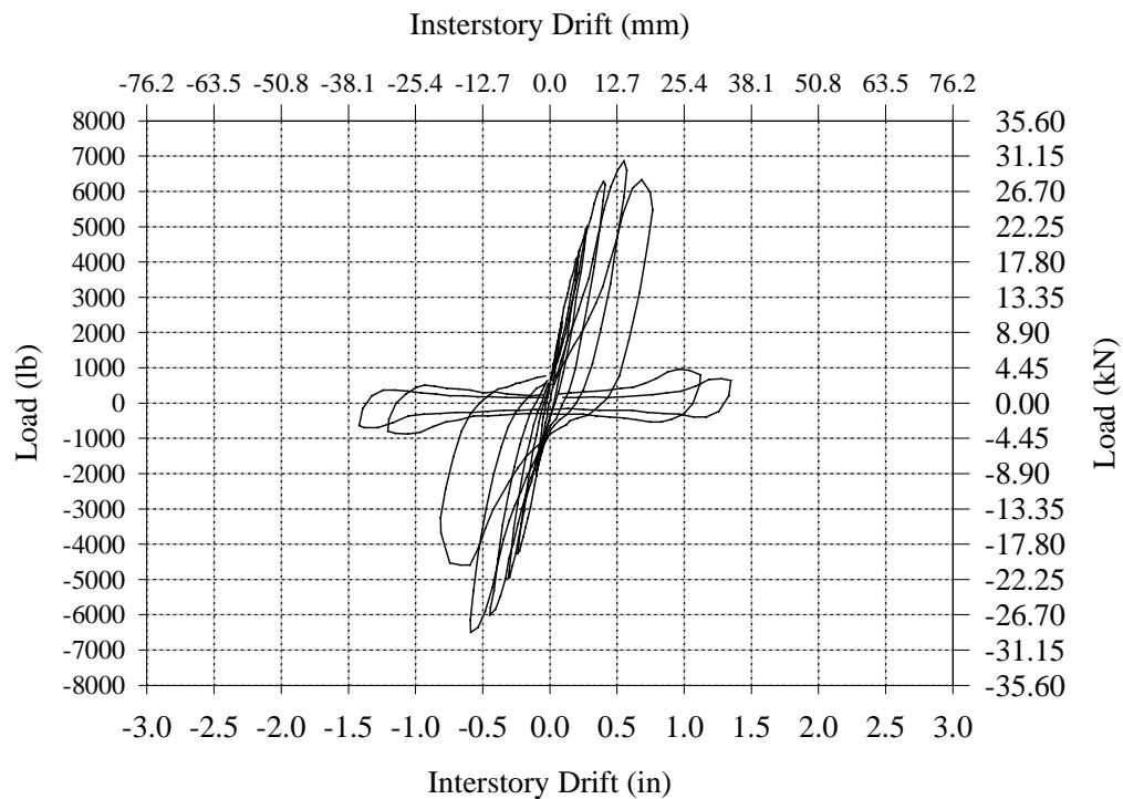
**Figure B.34 – Initial Hysteresis Curve for Wall DC-2.**
