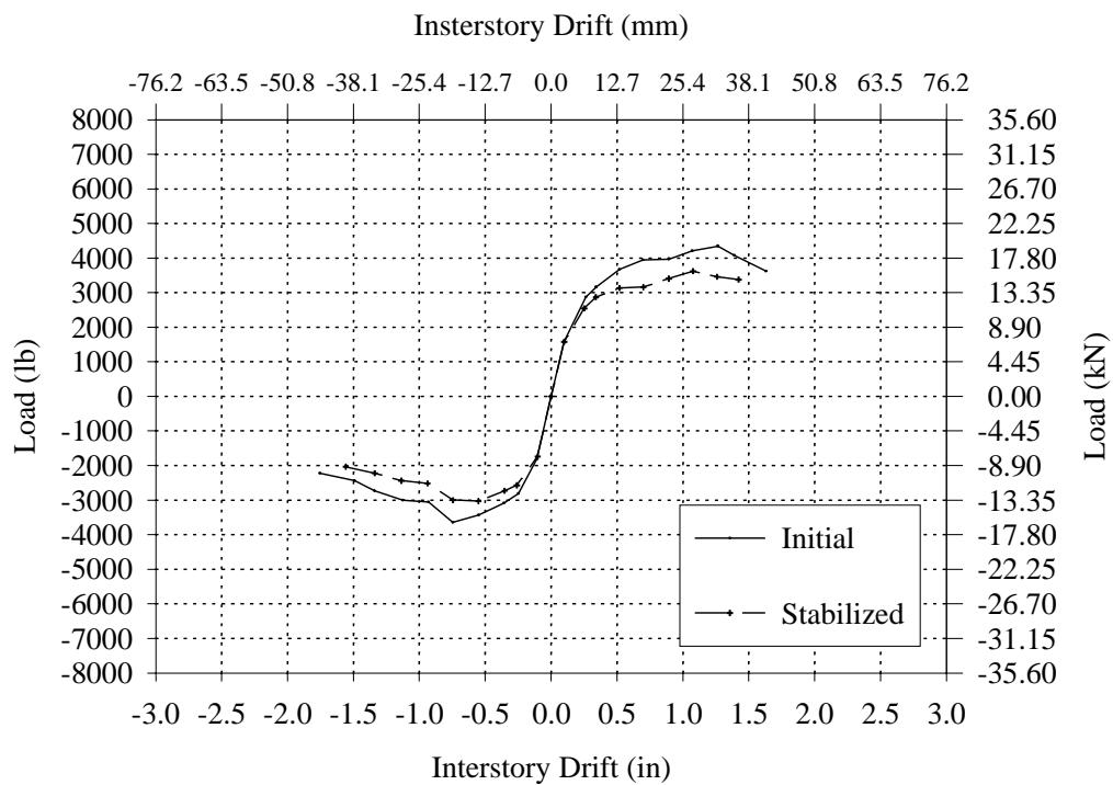
**Figure B.28 – Cyclic Envelope Curve for Wall CC-2.**
