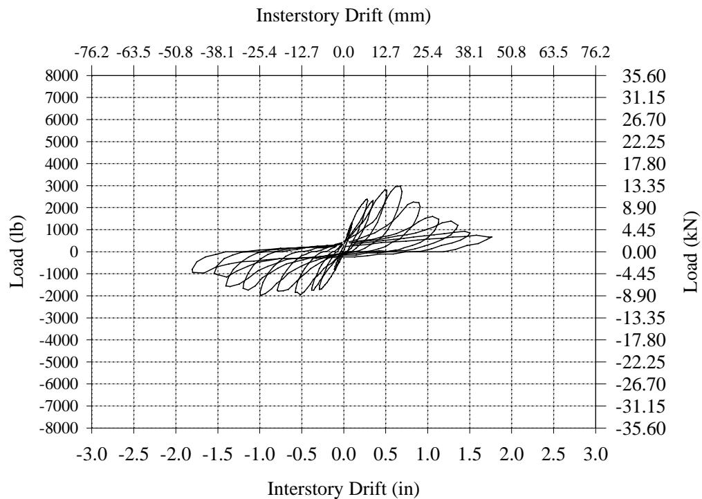
**Figure B.10 – Initial Hysteresis Curve for Wall AC-3.**
