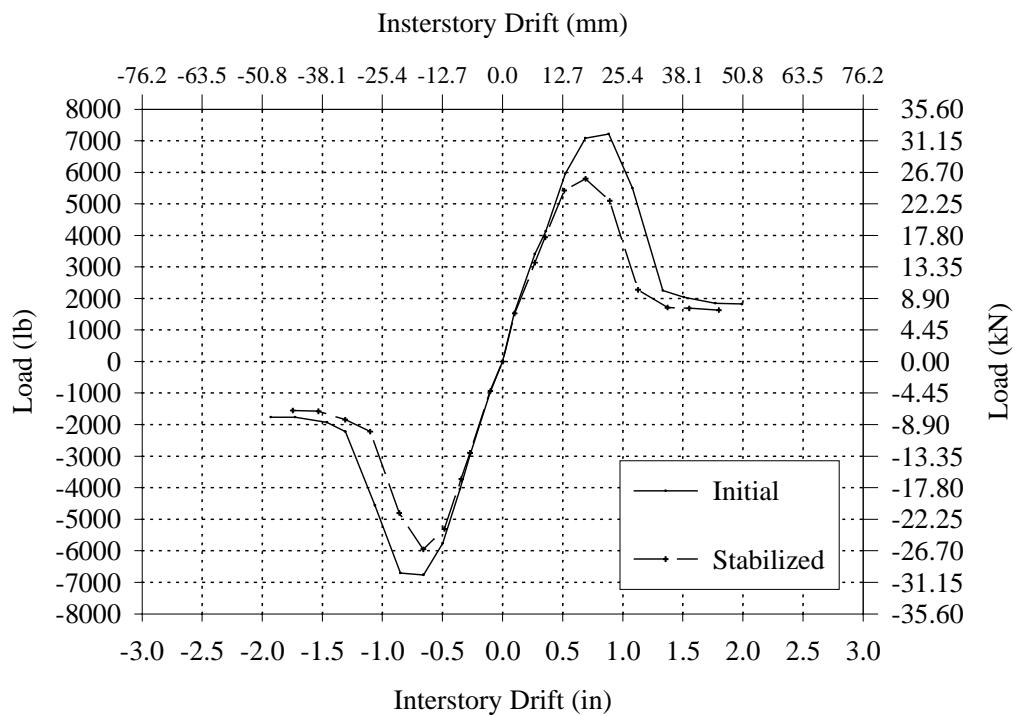
**Figure B.44 – Cyclic Envelope Curve for Wall EC-2.**
