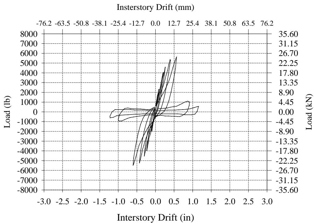
**Figure B.35 – Stabilized Hysteresis Curve for Wall DC-2.**
