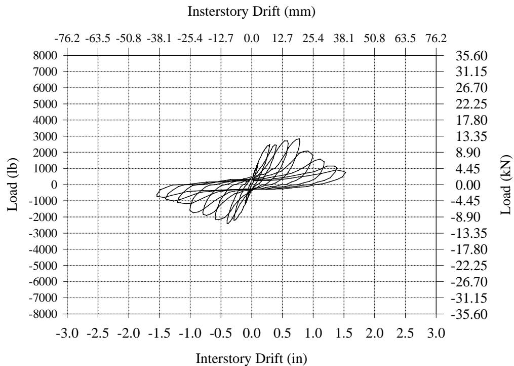
**Figure B.18 – Initial Hysteresis Curve for Wall BC-2.**
