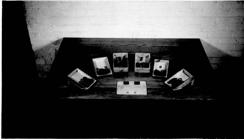
FIGURE 1. Work Place Arranged For Symmetrical Motion Path. Bins From Left To Right Are: Plain Washers, Lock Washers, Bolts, Bolts, Lock Washers, And Plain Washers.
