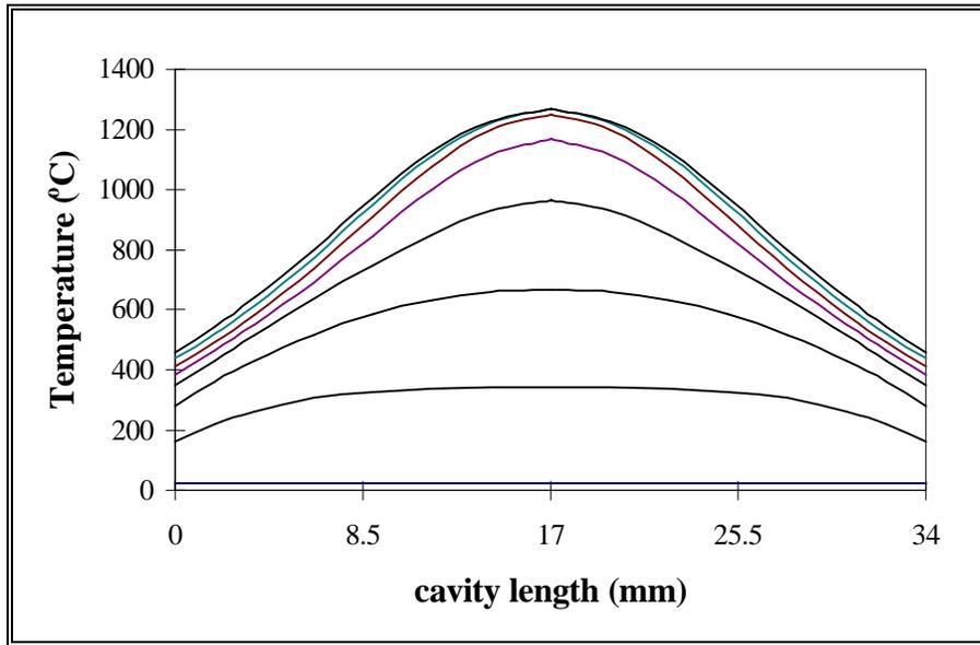
**Figure 4.8 Transient Temperature Distribution along a 4.67 mm Mullite Rod with an Absorbed Power of 50 W at 10 sec Intervals**
