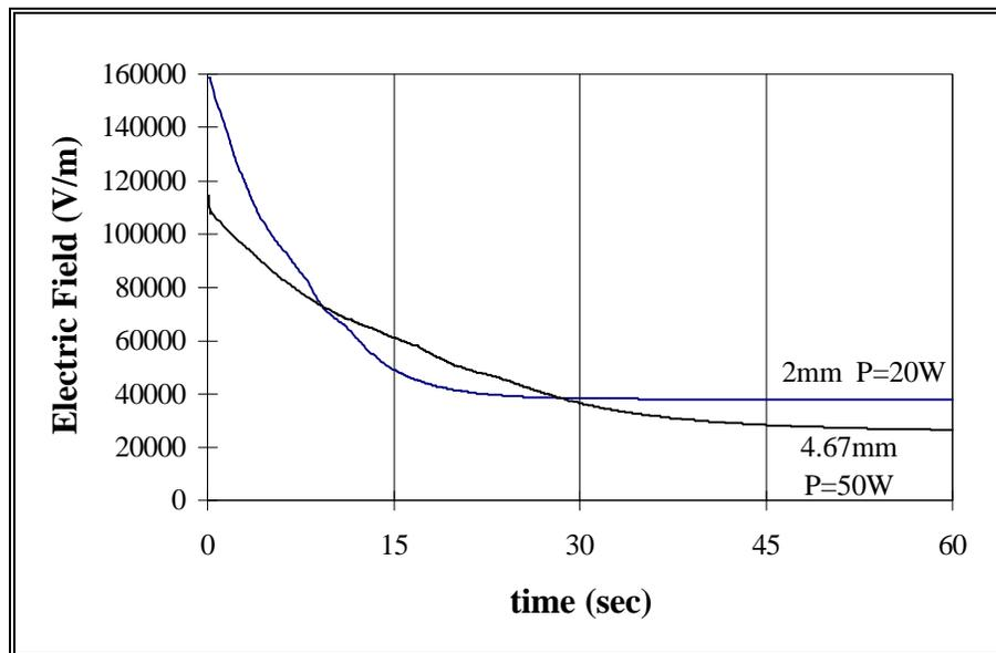
**Figure 4.10 Electromagnetic Fields Required to Hold the Absorbed Power Constant at 20W and 50W for a 2mm and 4.67mm Diameter Mullite Rod Respectively**
