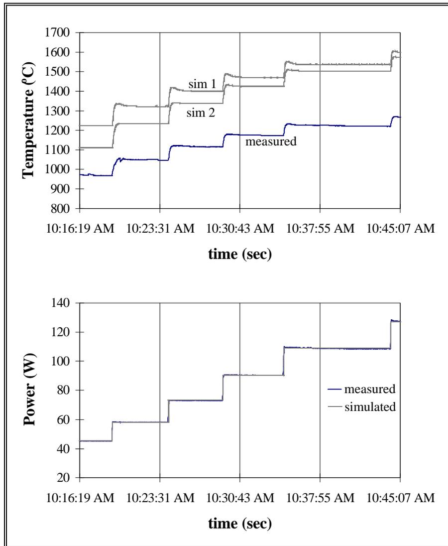
**Figure 4.13 Comparison of Actual Temperature Measurements with Simulated Data for the 4.67mm Diameter Case**
