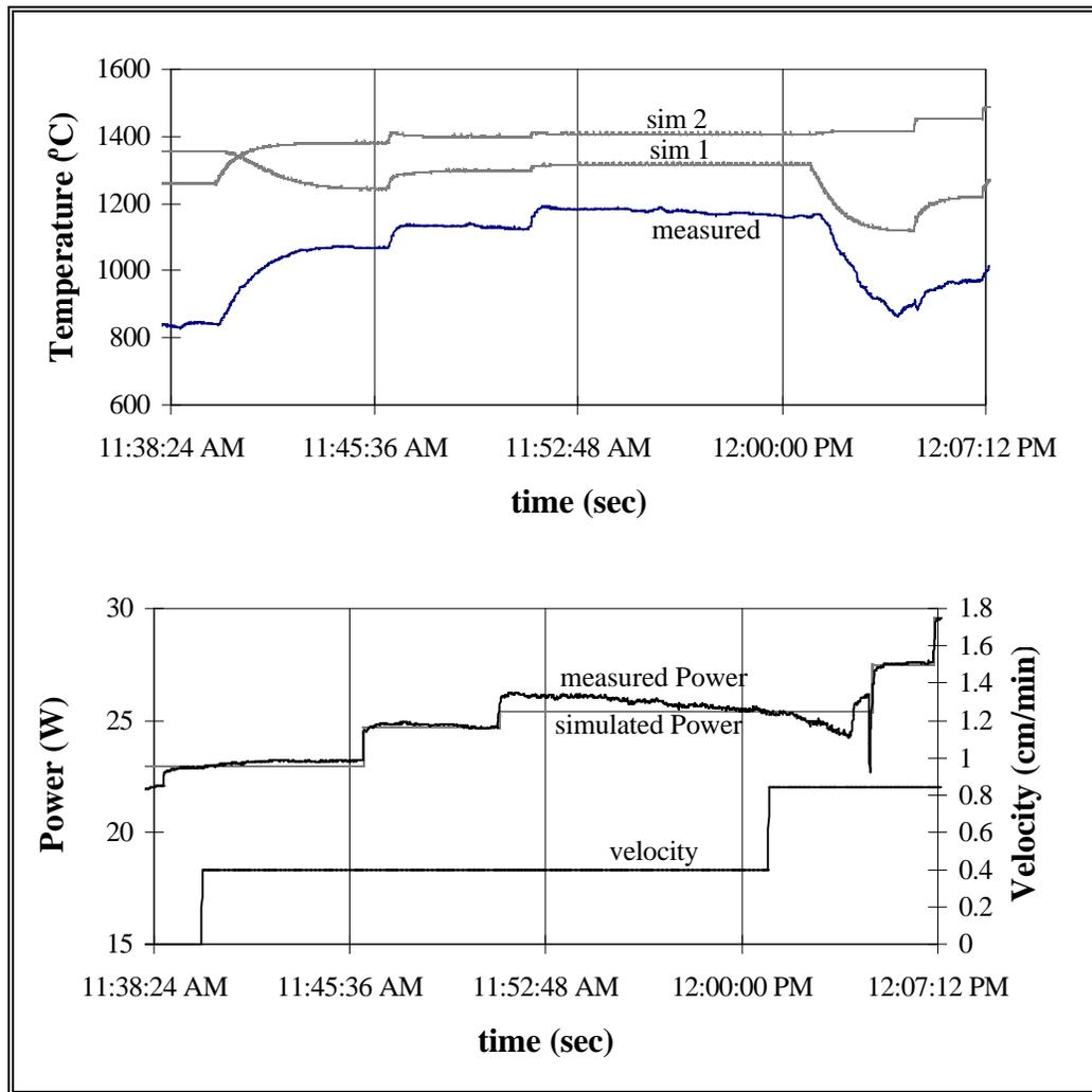
**Figure 4.12 Comparison of Actual Temperature Measurements with Simulated Data for the 2mm Diameter Case**
