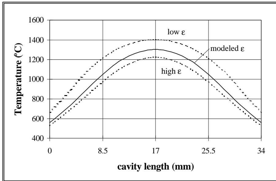
**Figure 4.11 Temperature Distribution of 4.67mm Mullite Rod at an Absorbed Power of 55 W with Different Emissivities**
