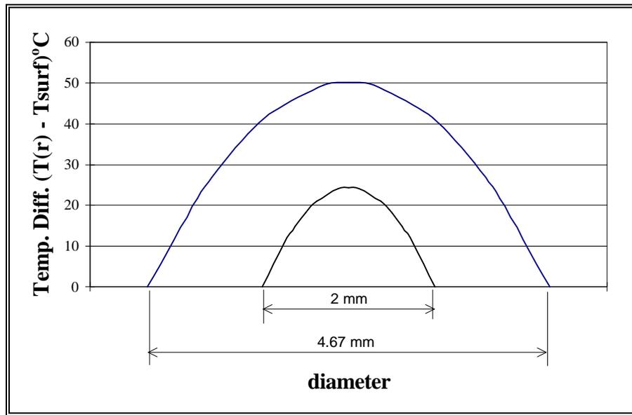
**Figure 4.3 Radial Temperature Distribution along a 2mm and 4.67mm Rod at Center**
