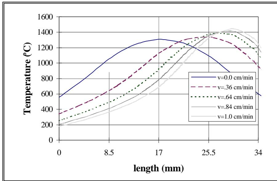
**Figure 4.6 Steady State Temperature Distribution along a 4.67 mm Diameter Rod for Various Velocities and an Absorbed Power of 55 W**
