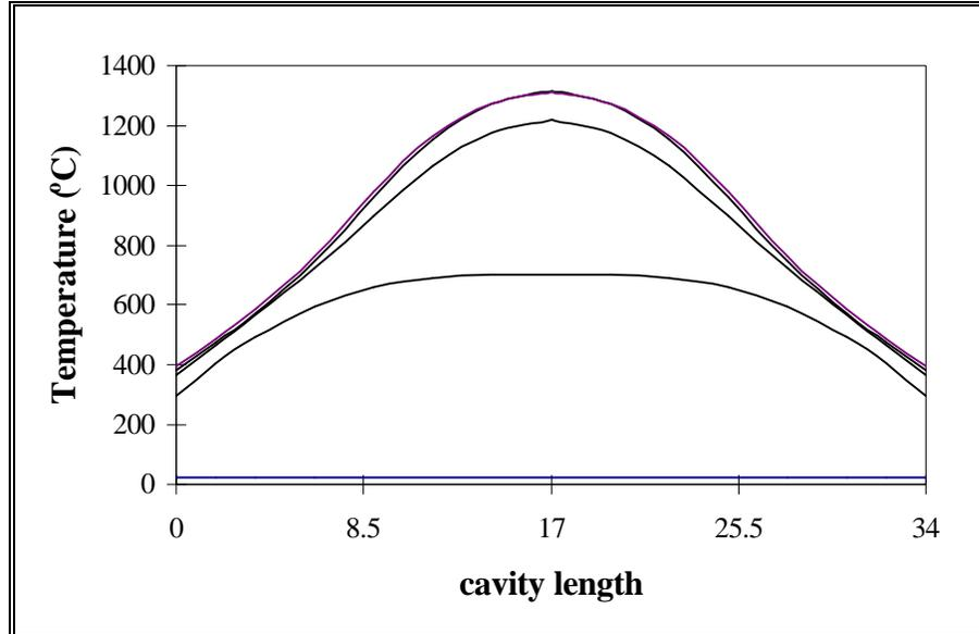
**Figure 4.7 Transient Temperature Distribution over a 2mm Mullite Rod with an Absorbed Power of 20 W at 10 sec Intervals**
