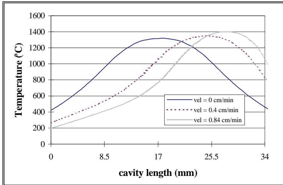
**Figure 4.5 Steady State Temperature Distribution along a 2mm Diameter Rod for Various Velocities and an Absorbed Power of 20W**
