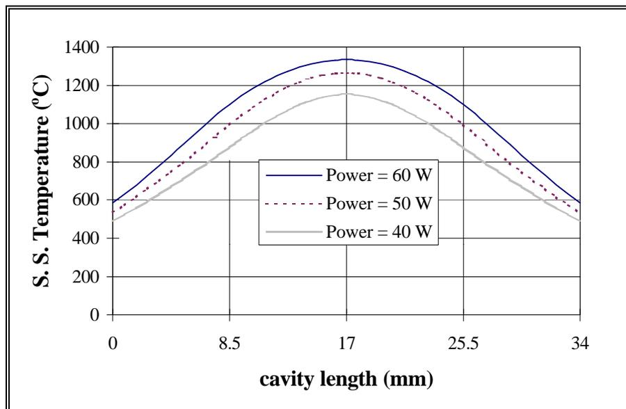
**Figure 4.2 Steady State Surface Temperature Distribution along a 4.67 mm Diameter Mullite Rod at Different Absorbed Powers with Respect to the Length of the Rod in the Cavity**
