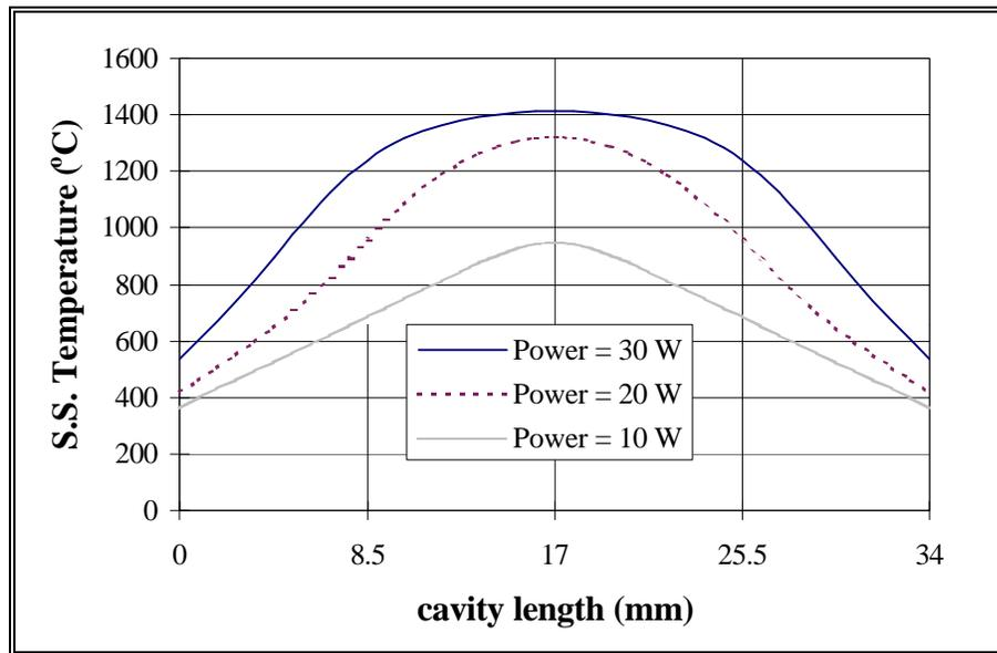
**Figure 4.1 Steady State Surface Temperature Distribution along a 2 mm Diameter Mullite Rod at Different Absorbed Powers with Respect to the Length of the Rod in the Cavity**
