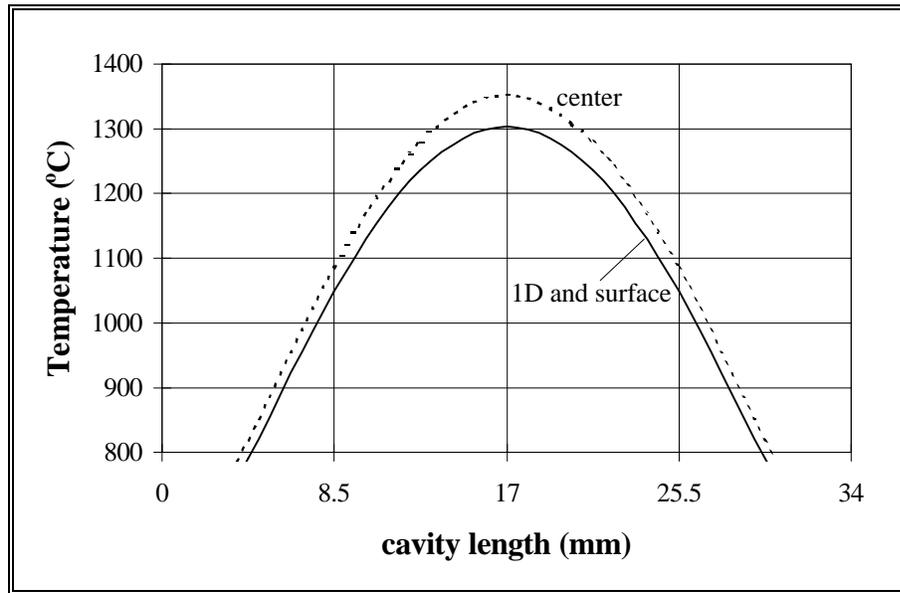
**Figure 4.4 Temperature Distribution Comparison of 1-D and 2-D models using a 4.67mm Diameter Mullite Rod**
