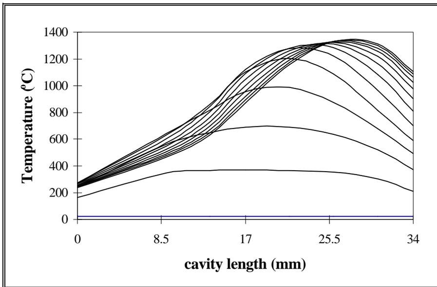
**Figure 4.9 Temperature Distribution along a 4.67 mm Mullite Rod at a Power of 50 W and velocity of 0.84 cm/sec at 10 sec Intervals**
