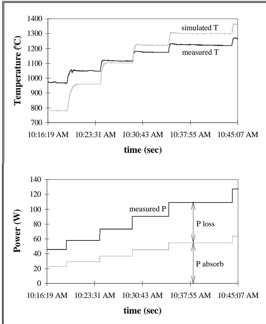
**Figure 4.14 Effect of Significant Power Loss on Temperature**
