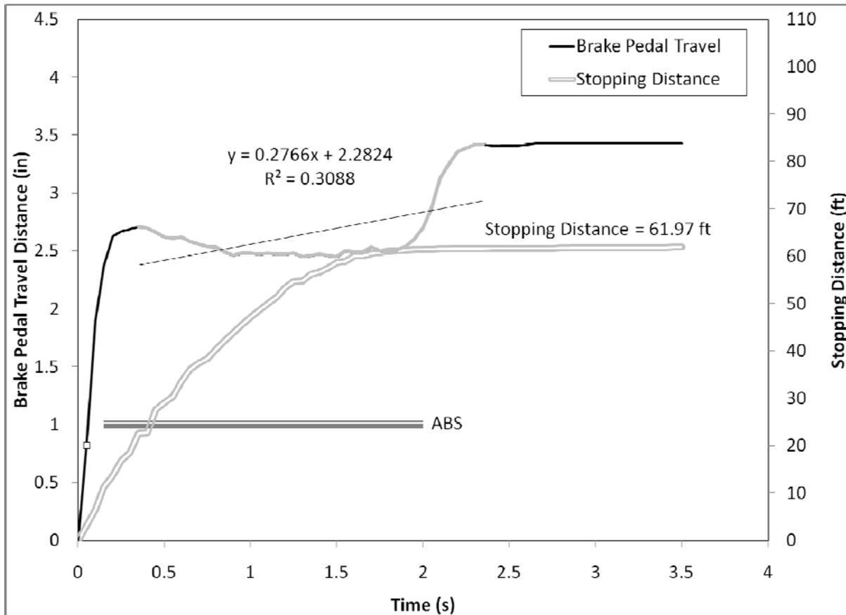
**Figure 105. Brake pedal displacement over the first 4 seconds of the R3 panic braking maneuver for Driver 43, an older male driving the Volvo S80**
