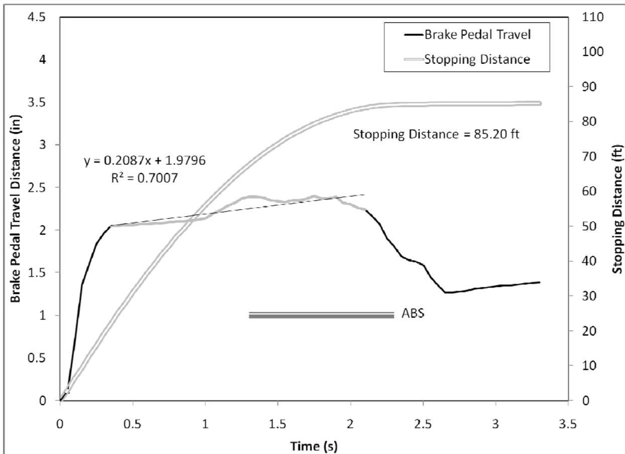
**Figure 132. Brake pedal displacement over the first 3.5 seconds of the R3 panic braking maneuver for Driver 65, a younger female driving the Volvo S80**
