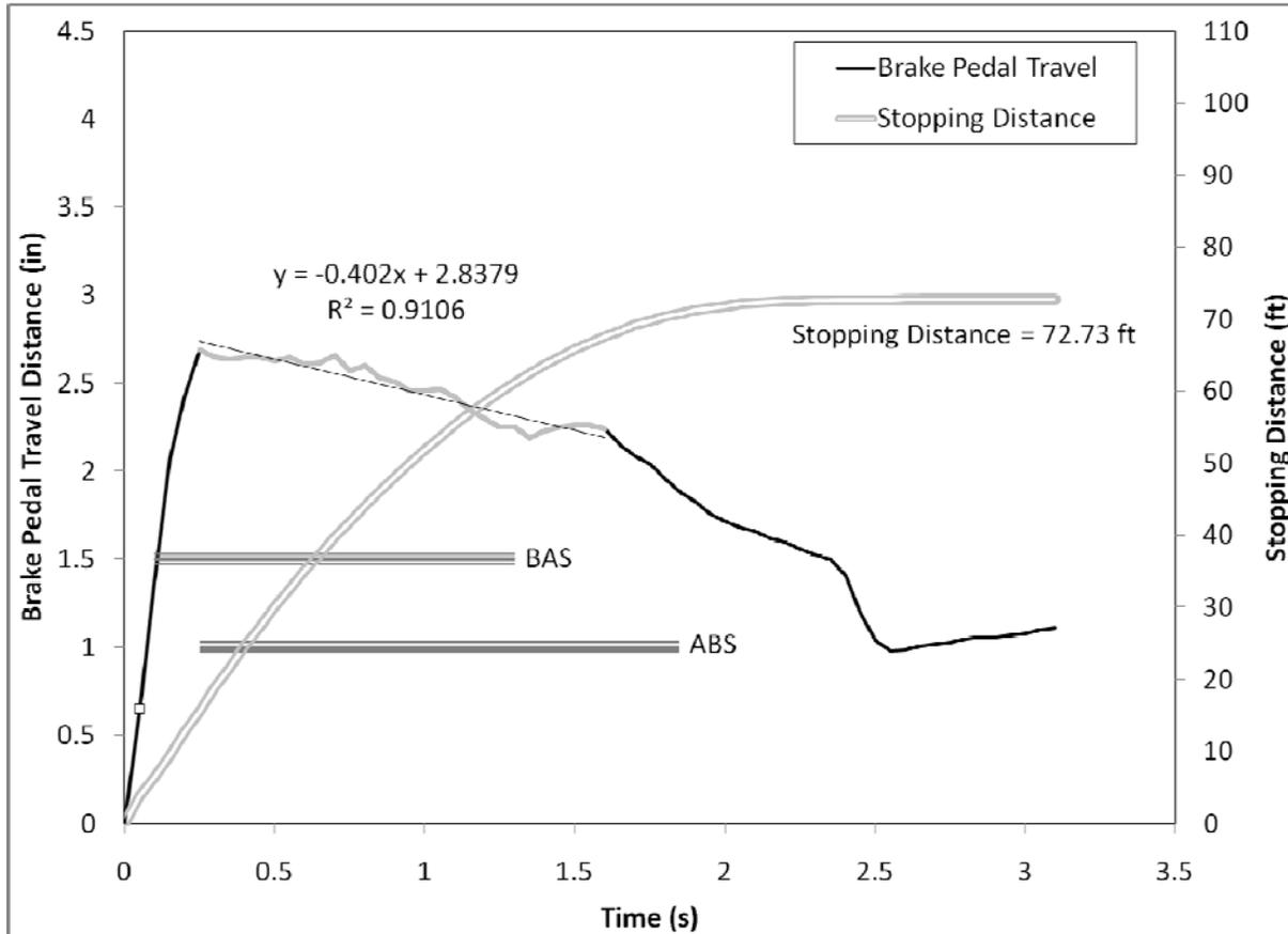
**Figure 130. Brake pedal displacement over the first 3.5 seconds of the R1 panic braking maneuver for Driver 65, a younger female driving the Volvo S80**
