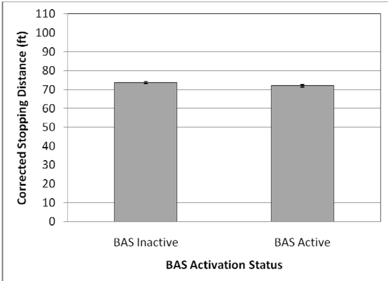
**Figure 38. Average Corrected Stopping Distances for all BAS-Active Stops and BAS-Inactive Stops in which ABS Activated in the Repeated Braking Session**
