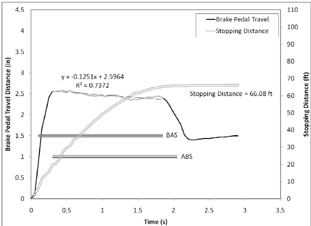
**Figure 113. Brake pedal displacement over the first 3.5 seconds of the R2 panic braking maneuver for Driver 52, a younger female driving the Volvo S80**
