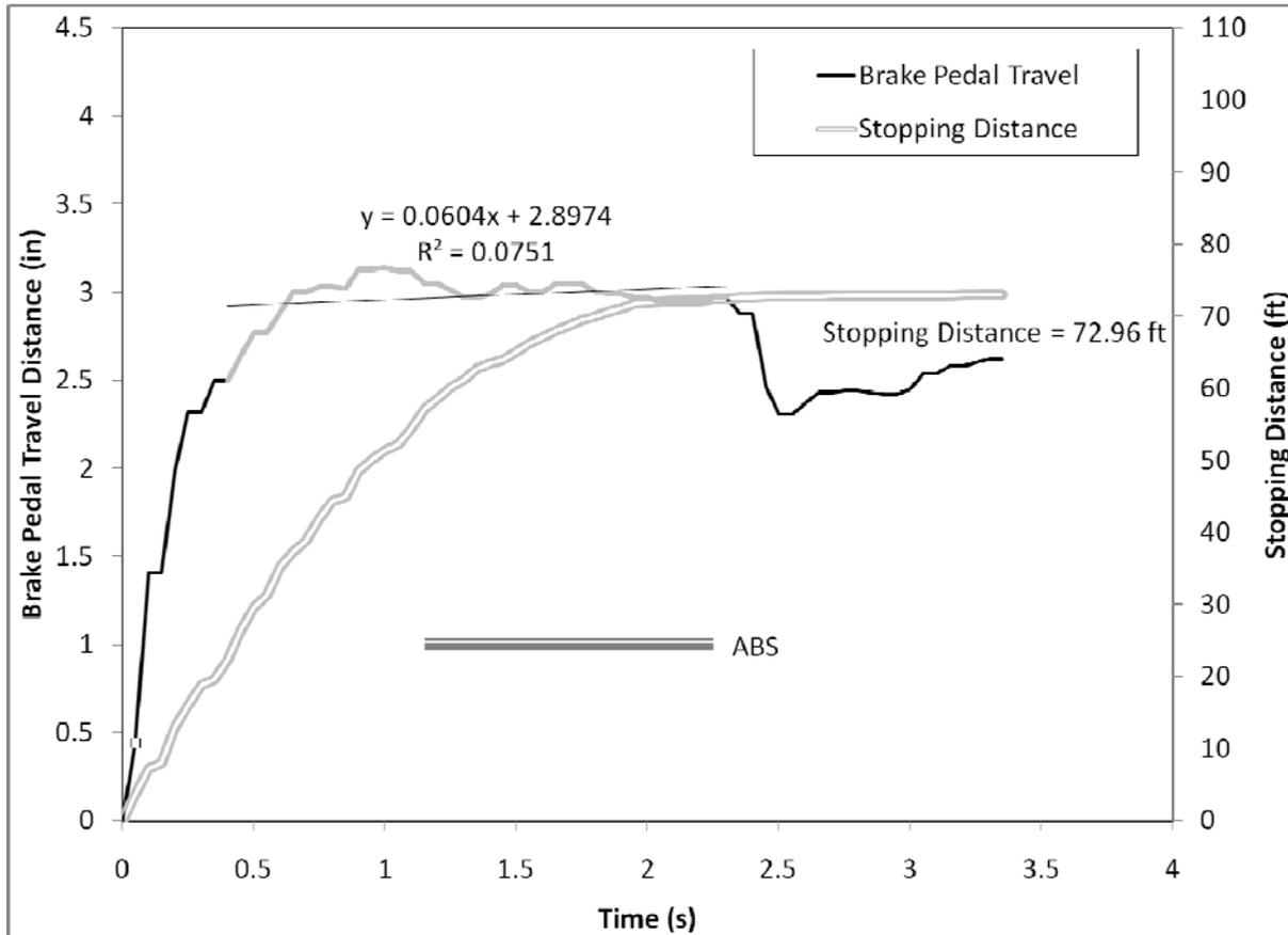
**Figure 97. Brake pedal displacement over the first 4 seconds of the R1 panic braking maneuver for Driver 26, a younger male driving the Mercedes-Benz R350**
