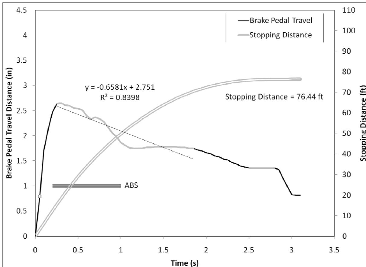
**Figure 131. Brake pedal displacement over the first 3.5 seconds of the R2 panic braking maneuver for Driver 65, a younger female driving the Volvo S80**
