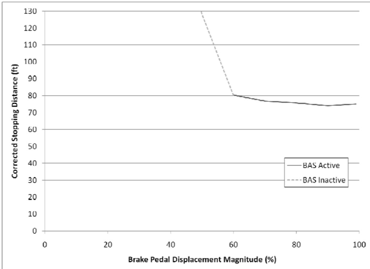
**Figure 14. Corrected Stopping Distance by Brake Pedal Displacement Magnitude for Tests Performed at 45 mph**
