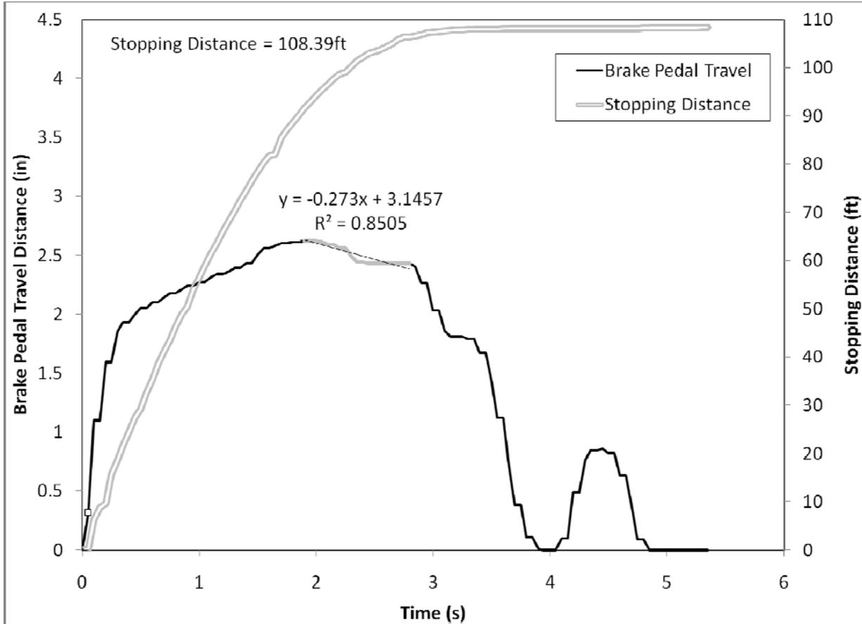
Figure 76. Driver 9, an older male driving the Mercedes-Benz R350, did not activate ABS in the braking maneuver.
