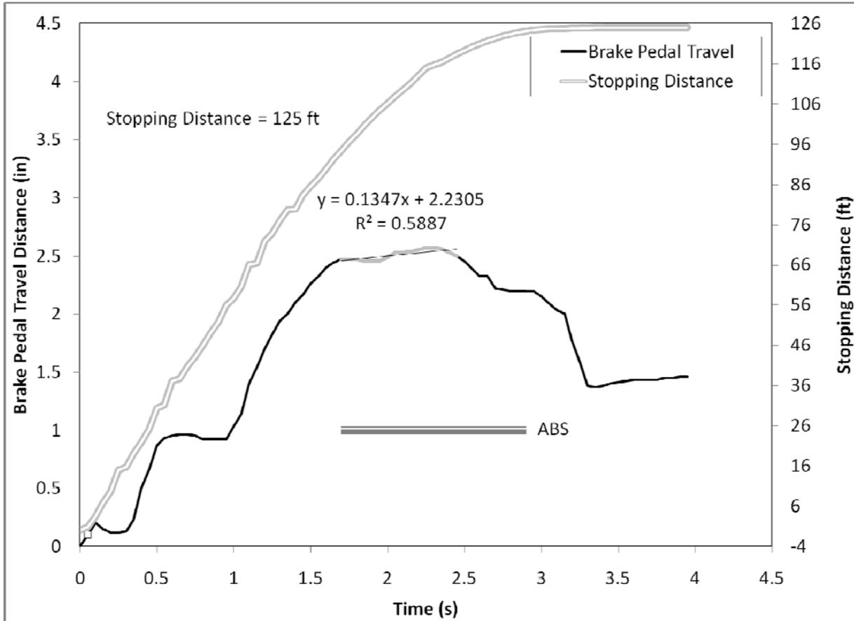
Figure 73. Driver 47, an older male driving the Volvo S80, activated ABS 1.7 seconds into the panic-braking maneuver.
