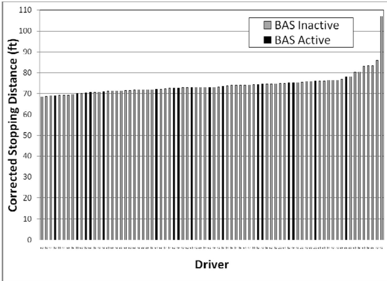
**Figure 46. Corrected Stopping Distance by BAS Activation in the Volvo S80**
