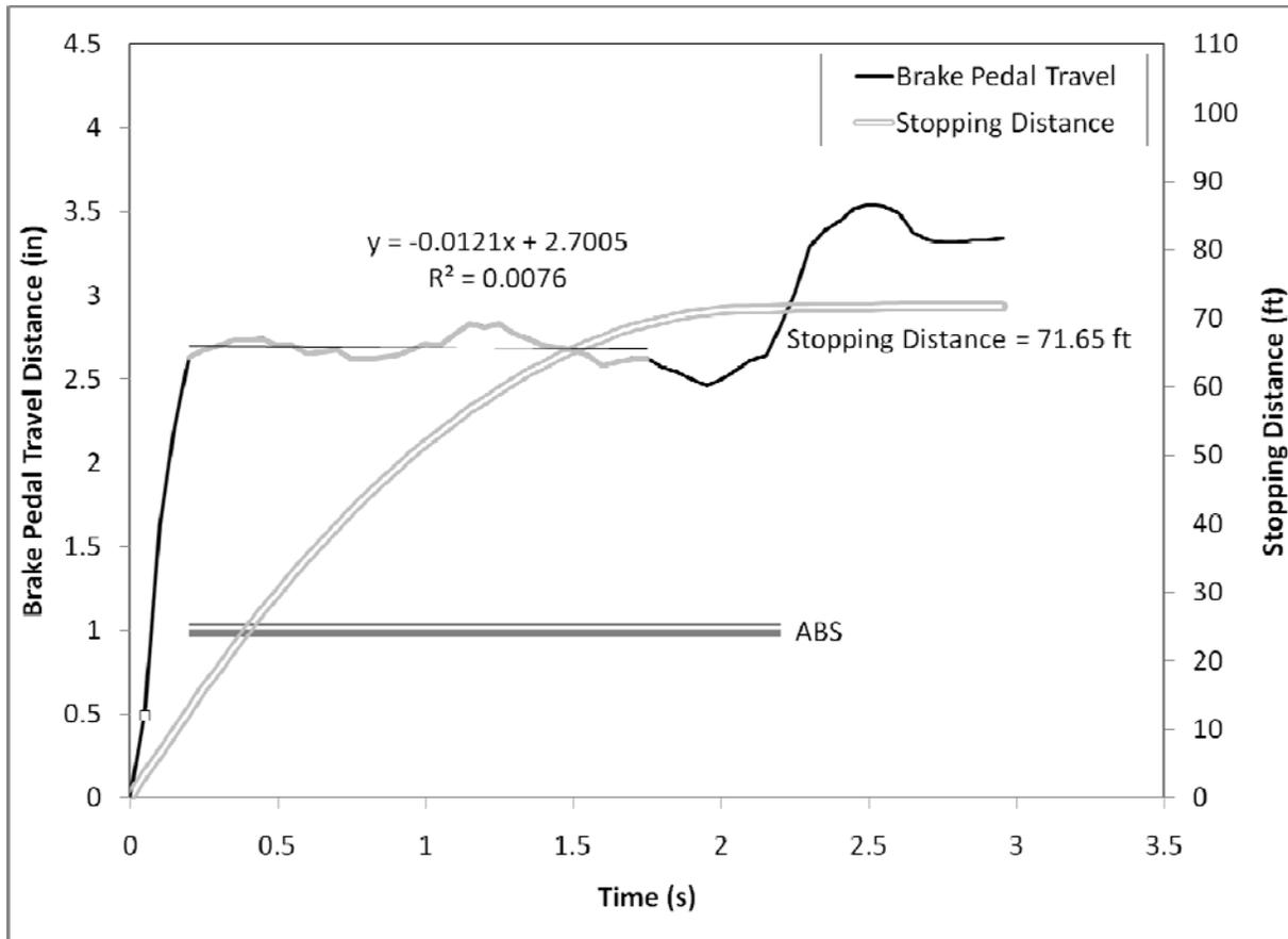
**Figure 108. Brake pedal displacement over the first 3.5 seconds of the R3 panic braking maneuver for Driver 49, a younger male driving the Volvo S80**
