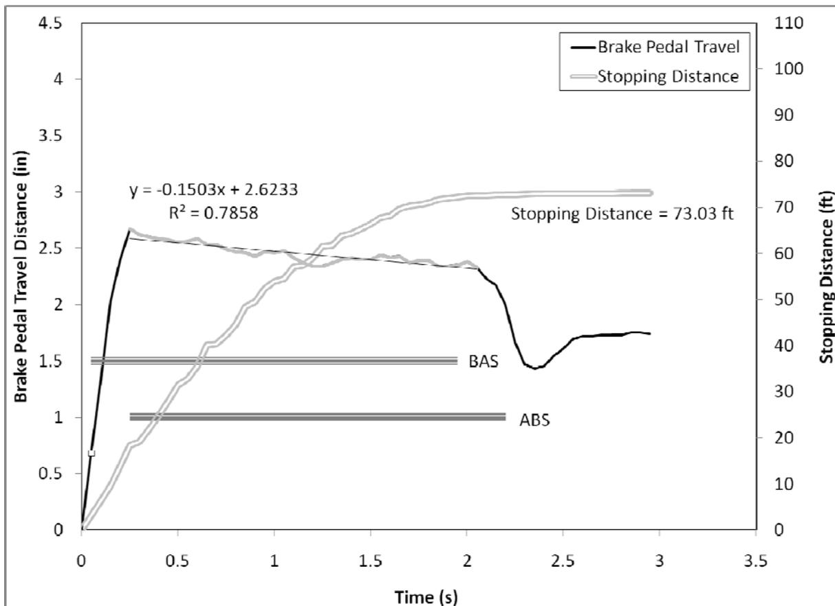
**Figure 129. Brake pedal displacement over the first 3.5 seconds of the R3 panic braking maneuver for Driver 64, a younger male driving the Volvo S80**
