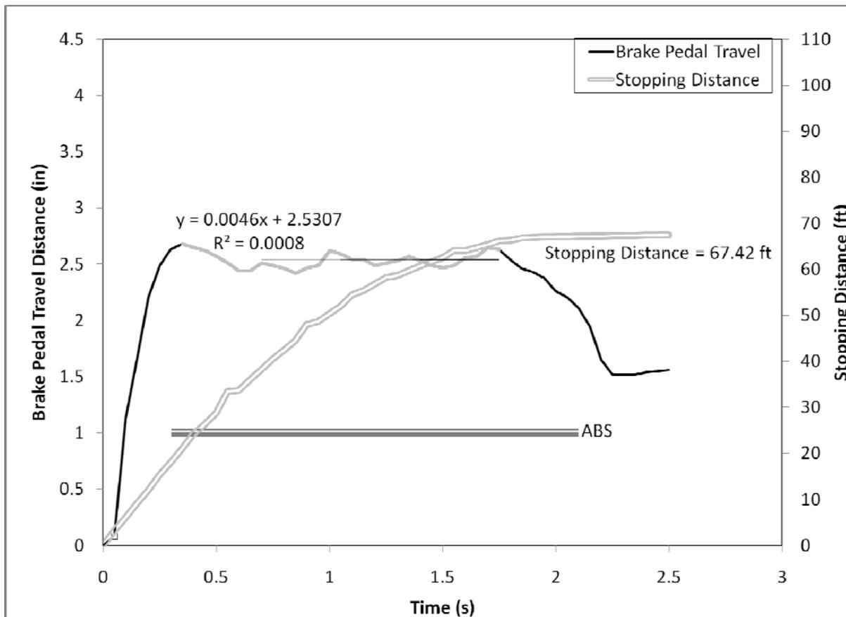
**Figure 114. Brake pedal displacement over the first 3 seconds of the R3 panic braking maneuver for Driver 52, a younger female driving the Volvo S80**
