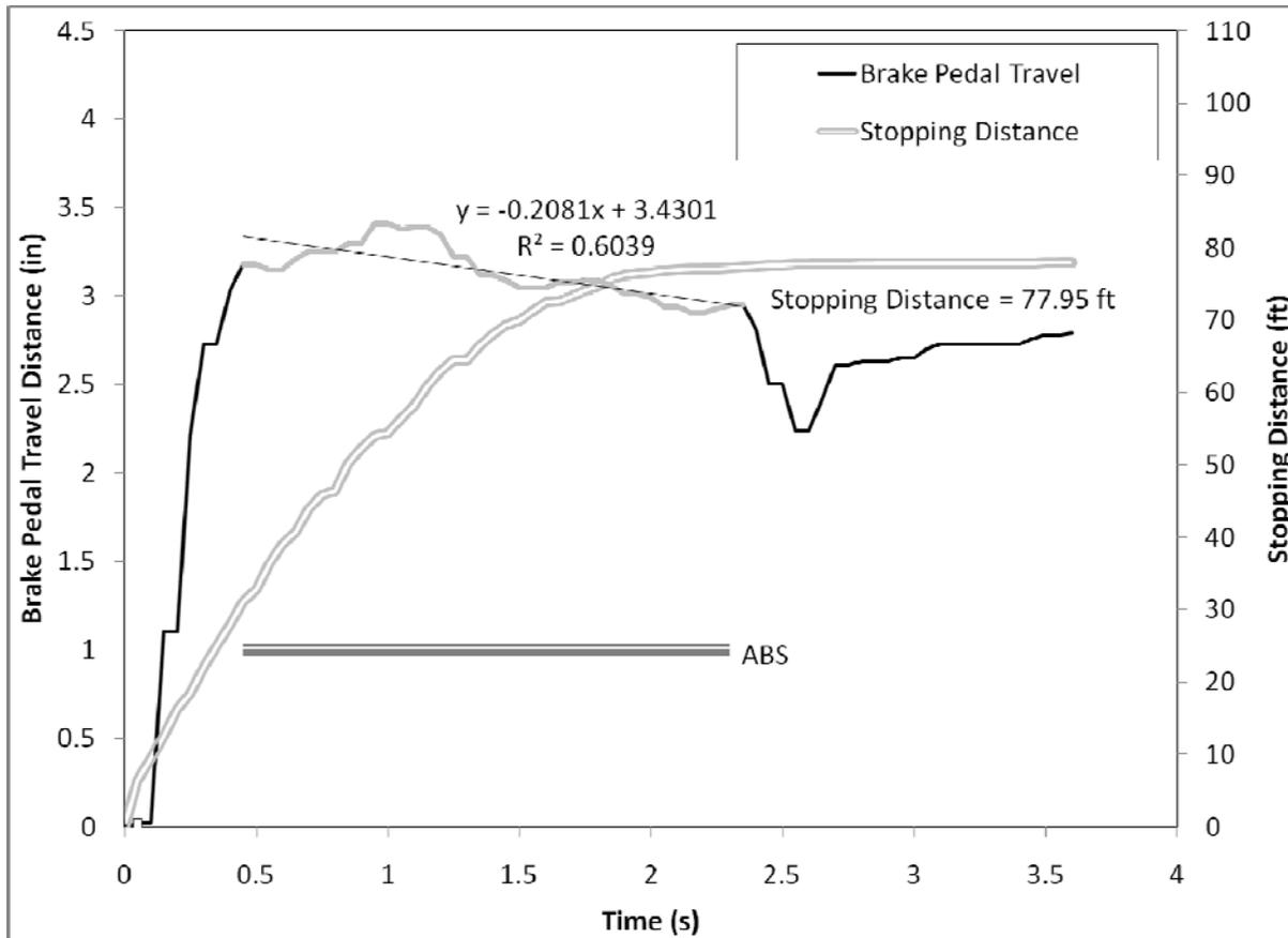
**Figure 93. Brake pedal displacement over the first 4 seconds of the R3 panic braking maneuver for Driver 10, an older male driving the Mercedes-Benz R350**
