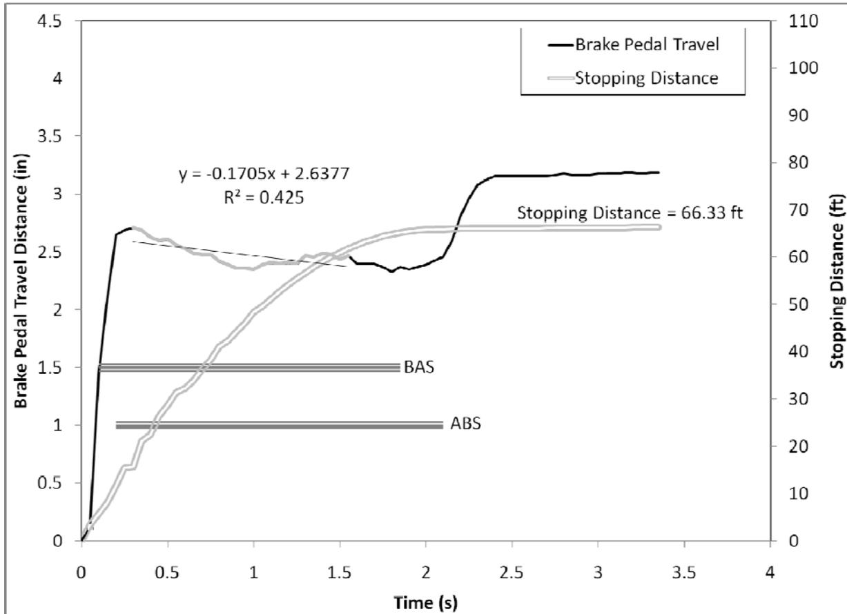
**Figure 103. Brake pedal displacement over the first 4 seconds of the R1 panic braking maneuver for Driver 43, a older male driving the Volvo S80**
