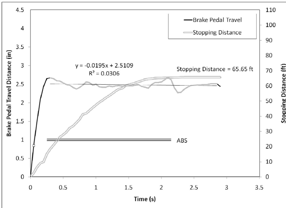
**Figure 111. Brake pedal displacement over the first 3.5 seconds of the R3 panic braking maneuver for Driver 50, a younger female driving the Volvo S80**
