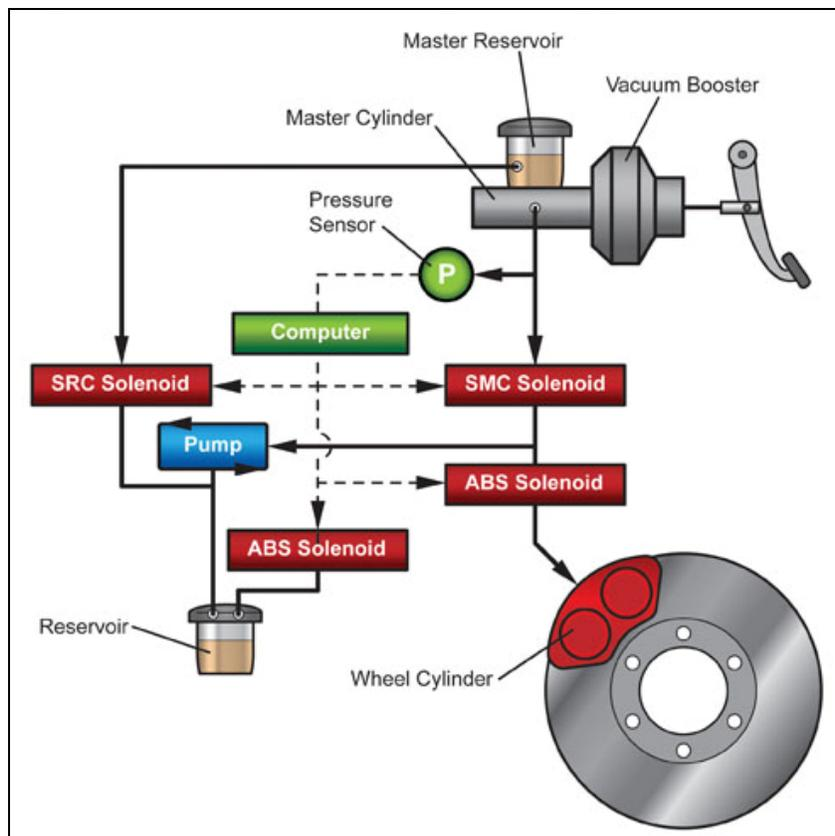
**Figure 6. Components of Pump-motor-applied BAS (from Hara, Ohta, Yamamoto, & Yoshida, 1998)**
