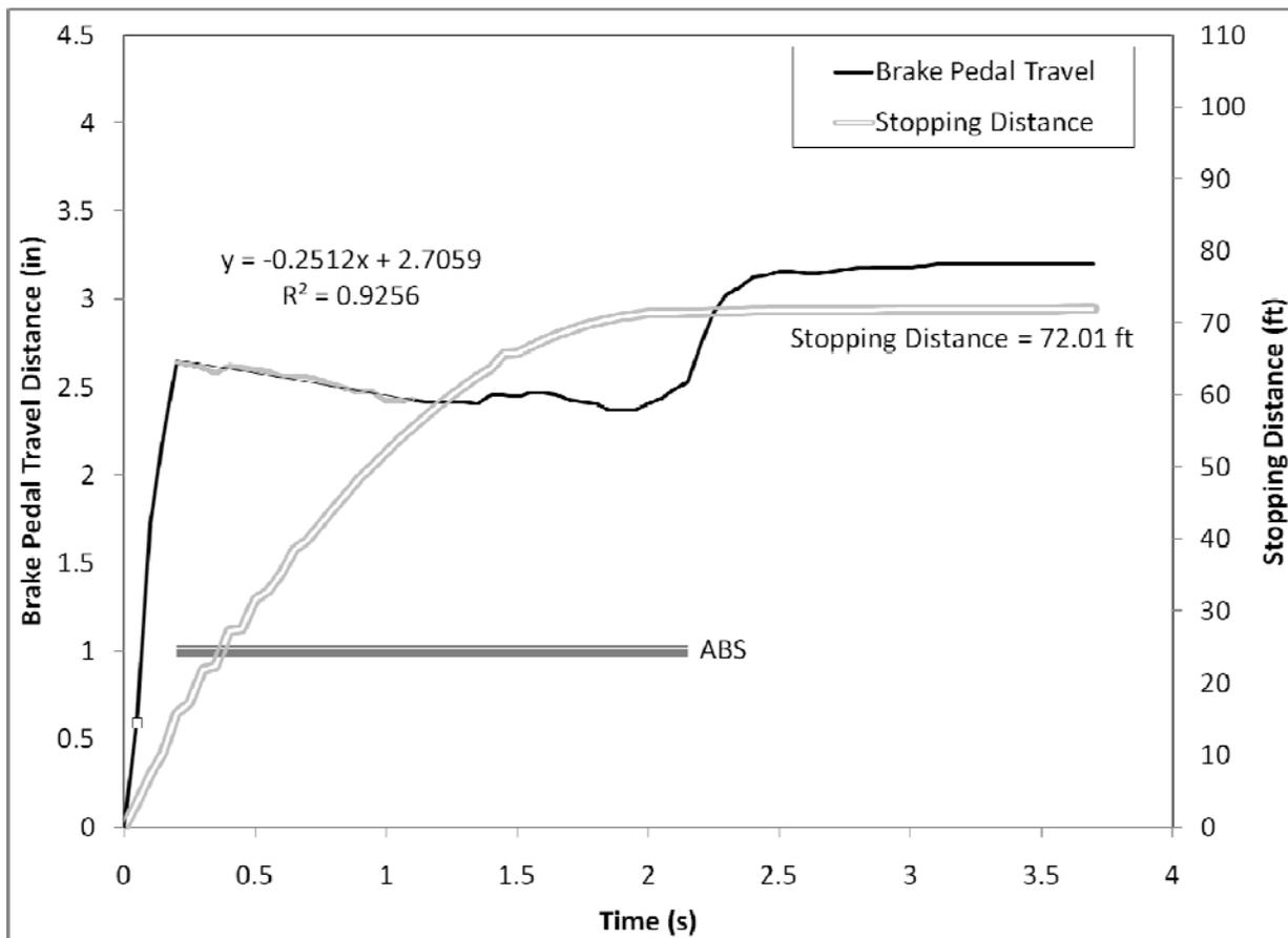
**Figure 104. Brake pedal displacement over the first 4 seconds of the R2 panic braking maneuver for Driver 43, a older male driving the Volvo S80**
