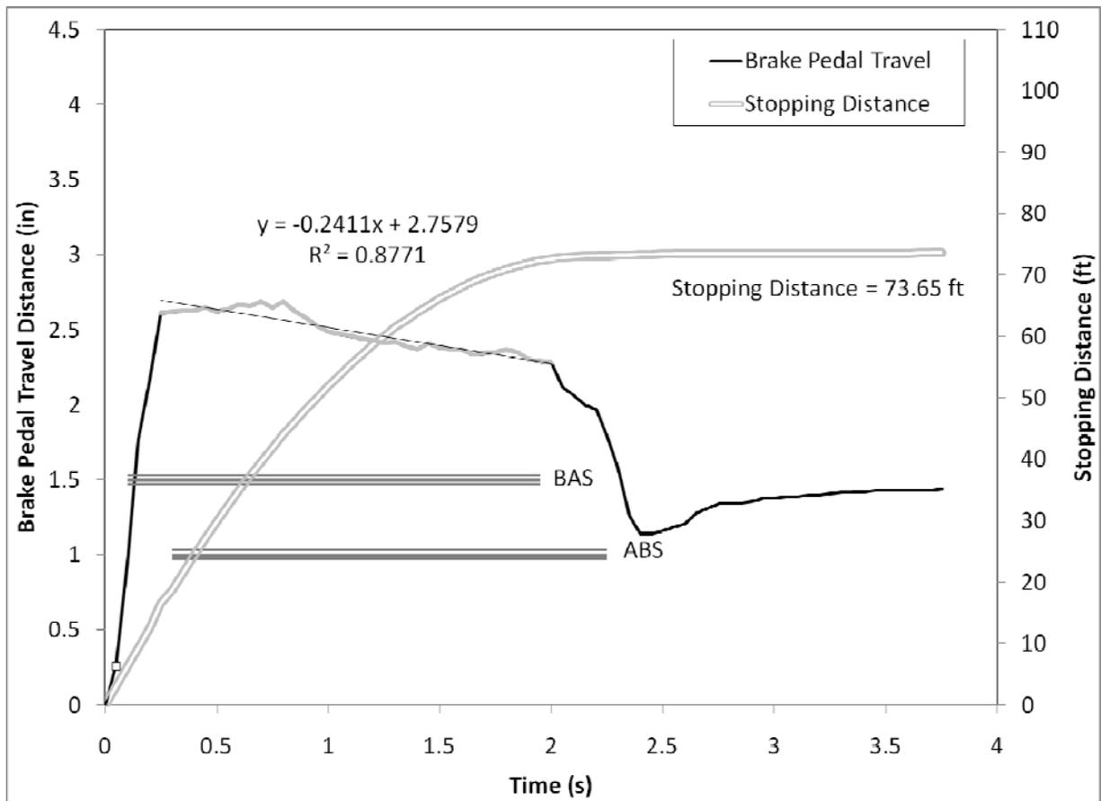
**Figure 96. Brake pedal displacement over the first 4 seconds of the R3 panic braking maneuver for Driver 21, a younger female driving the Volvo S80**
