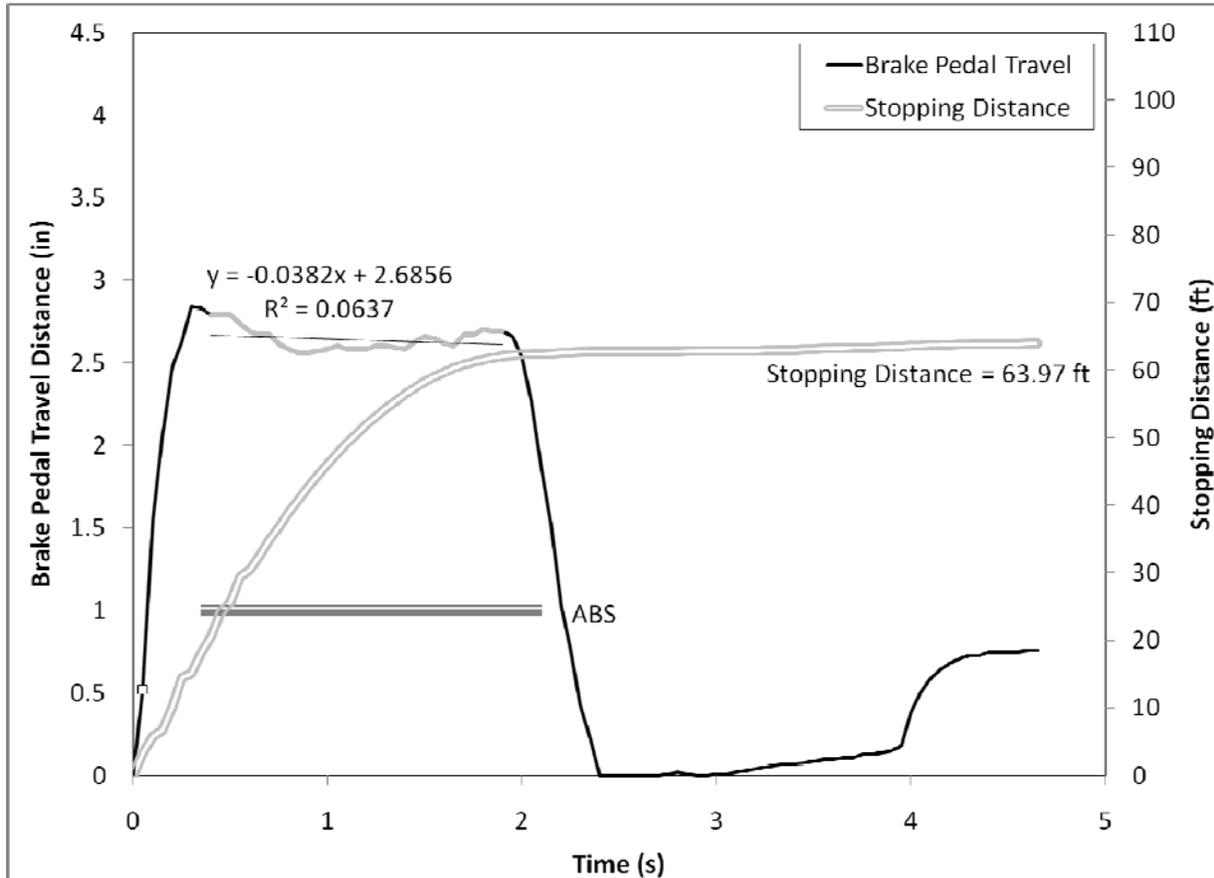
**Figure 124. Brake pedal displacement over the first 5 seconds of the R1 panic braking maneuver for Driver 63, a younger male driving the Volvo S80**
