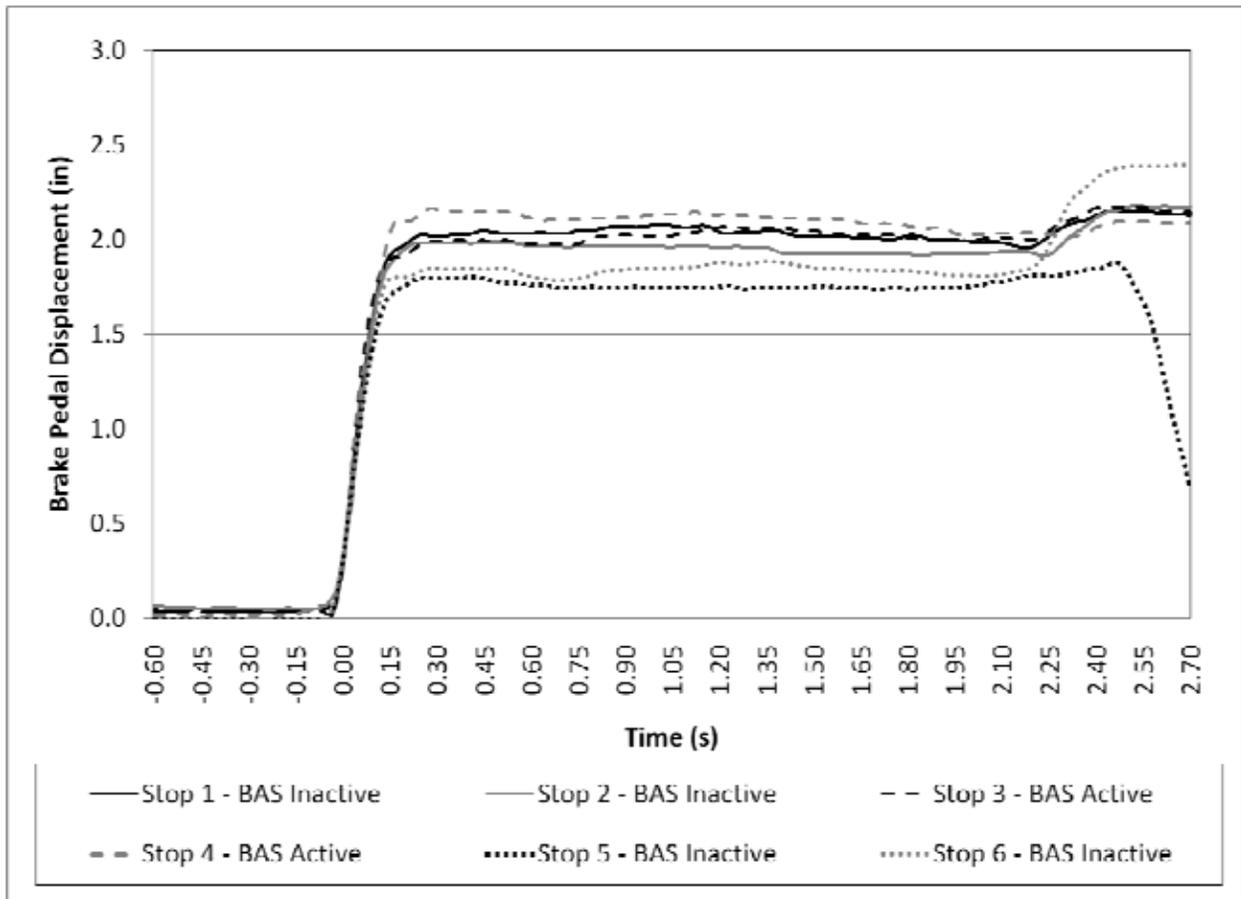
**Figure 22. Four Stops Performed by a Human Driver (Stops 1 – 4). BAS Activated for Stops 3 and 4. Two Stops Performed by Mechanical Brake Controller (Stops 5 and 6)**
