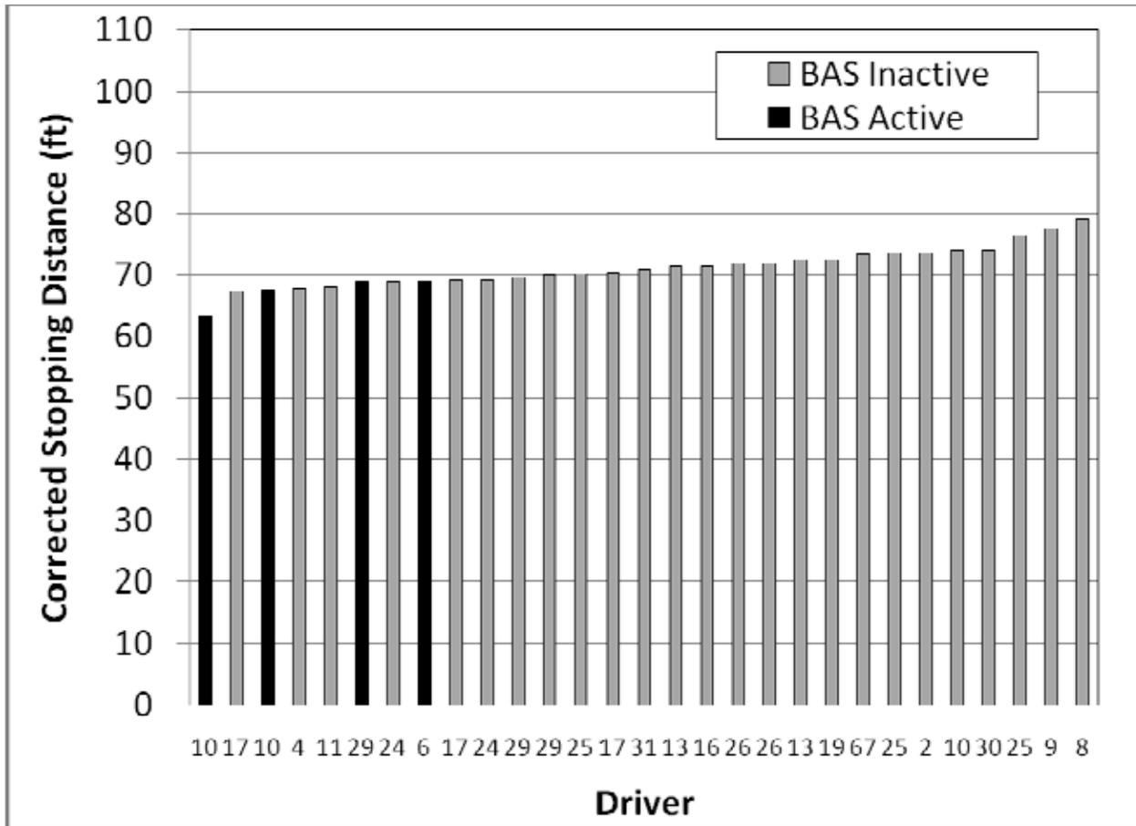
**Figure 45. Corrected Stopping Distance by BAS Activation in the Mercedes-Benz R350**
