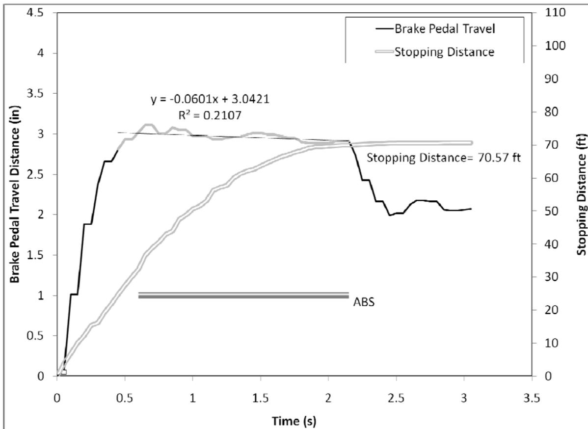
**Figure 99. Brake pedal displacement over the first 4 seconds of the R3 panic braking maneuver for Driver 26, a younger male driving the Mercedes-Benz R350**
