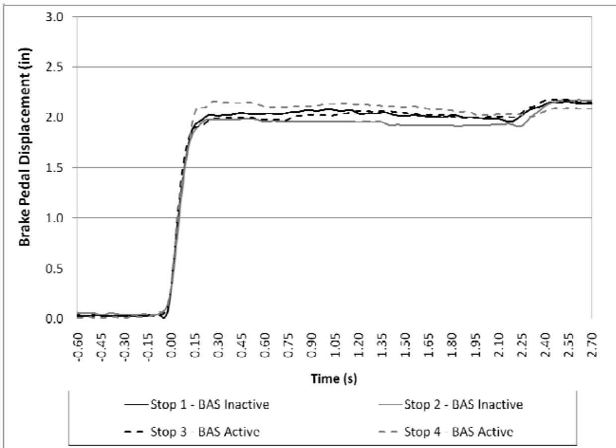
**Figure 20. Four Stops Performed by a VRTC Professional Driver. BAS Activated for Two Stops; All Stops have Similar Braking Profiles and Initial Speeds.**
