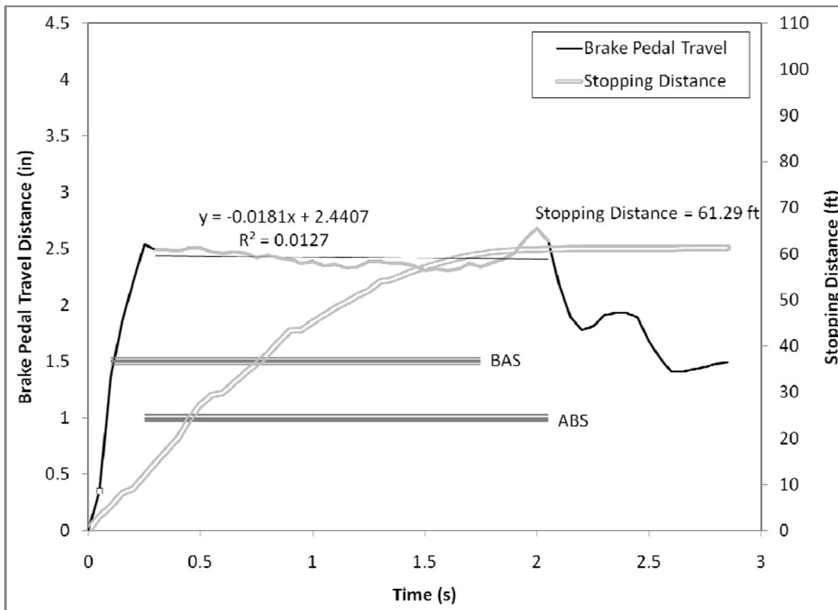
**Figure 110. Brake pedal displacement over the first 3 seconds of the R2 panic braking maneuver for Driver 50, a younger female driving the Volvo S80**
