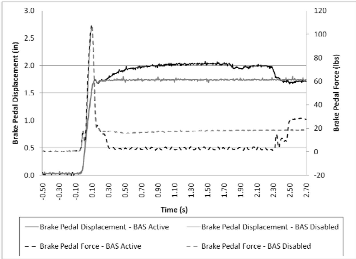
**Figure 19. Plot of Brake Pedal Displacement Magnitude (in) versus Time (s) at Activation Threshold for Two Stops (one with BAS Activated, the other with BAS Disabled) using the Mercedes-Benz R350**
