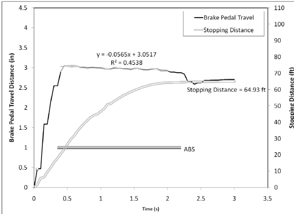
**Figure 101. Brake pedal displacement over the first 3.5 seconds of the R2 panic braking maneuver for Driver 29, a younger male driving the Mercedes-Benz R350**
