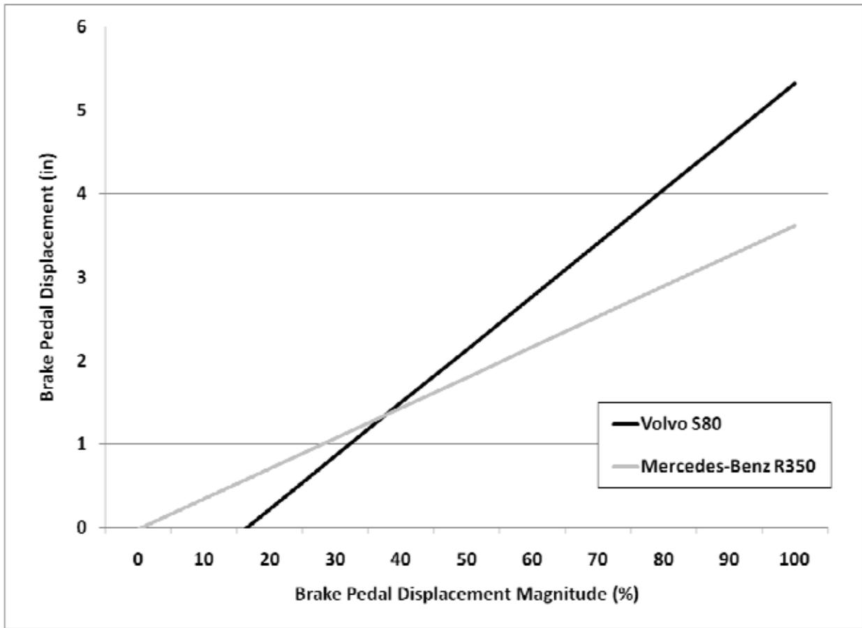
**Figure 30. Plot of Predicted Values for Pedal Travel in Percent and Inches**
