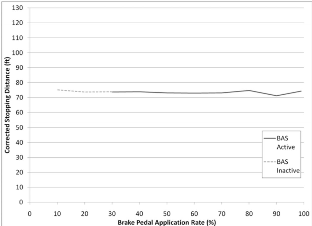
**Figure 17. Corrected Stopping Distance by Brake Pedal Application Rate (Holding Brake Pedal Force Magnitude at 50 percent) at 45 mph**
