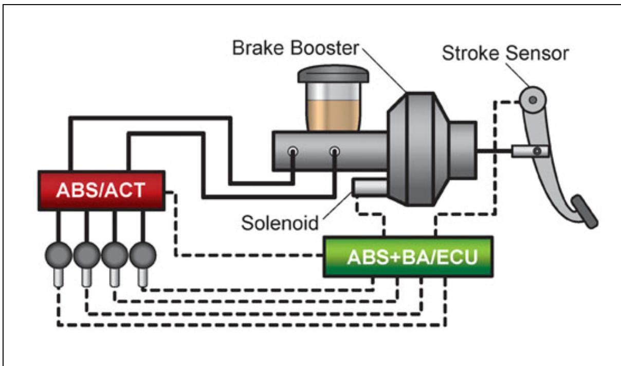
**Figure 4. Diagram Illustrating how Vacuum Booster BAS and Other Braking Elements are Connected (from Yoshida et al., 1998)**
