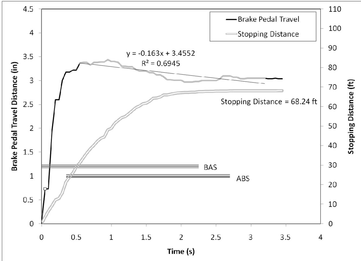
**Figure 91. Brake pedal displacement over the first 4 seconds of the R1 panic braking maneuver for Driver 10, an older male driving the Mercedes-Benz R350**
