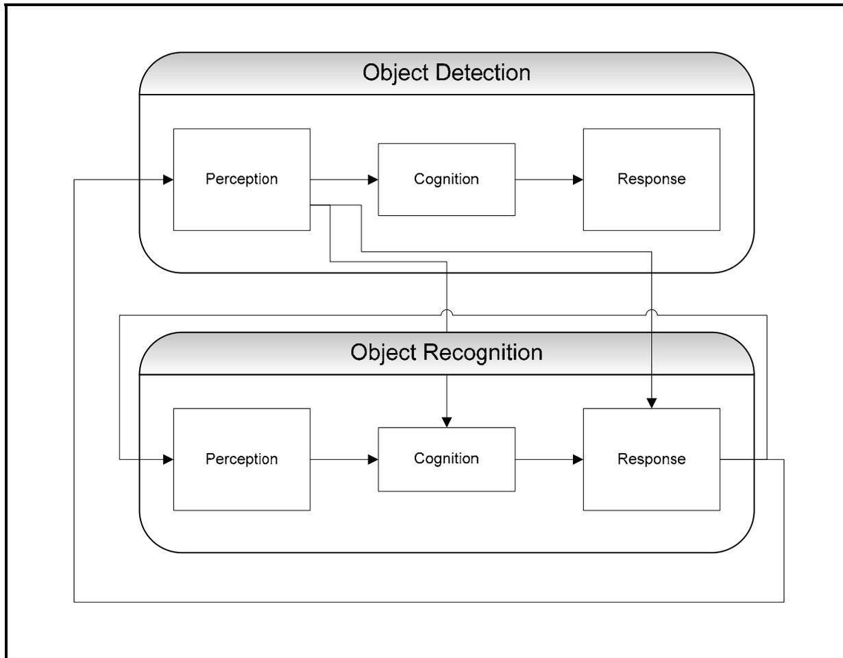
**Figure 53. Stages of Human Information Processing Relevant to Panic-Braking Performance**
