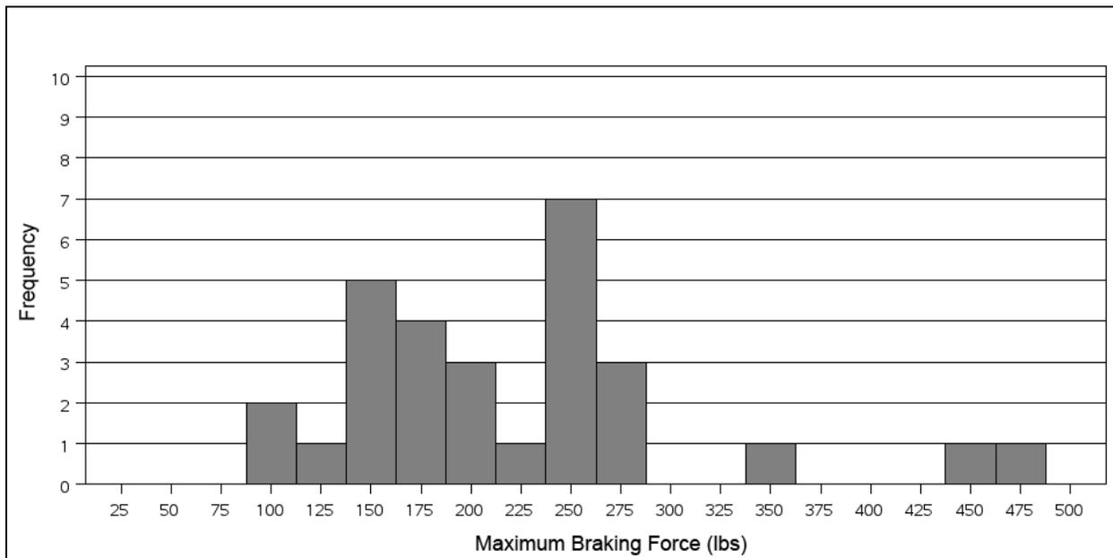
**Figure 49. Maximum Brake Pedal Force for Drivers Assigned to the Volvo S80**
