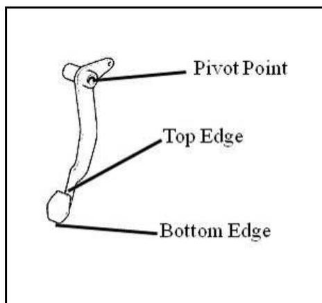
**Figure 29. Diagram Showing Measurement Locations on Brake Pedal Pad**
