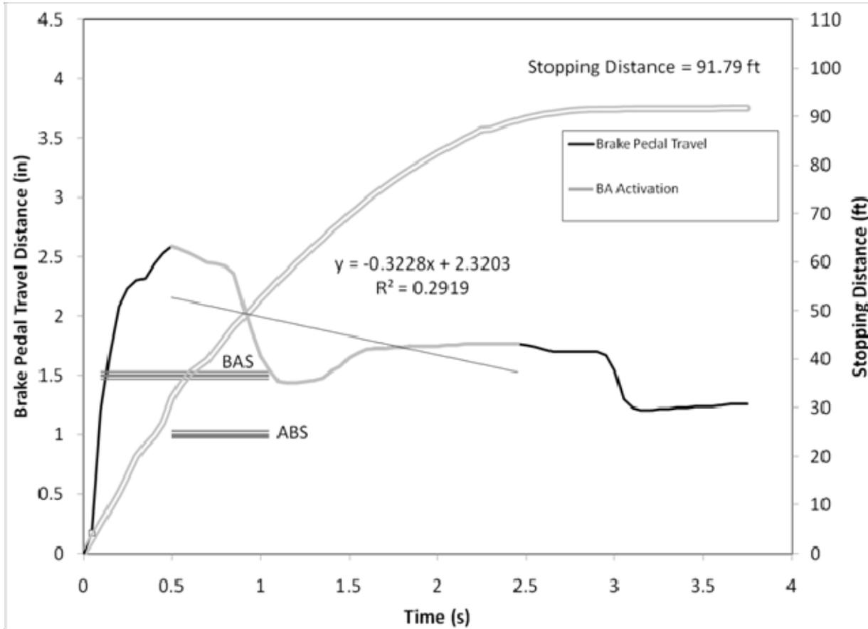
Figure 84. Driver 43, an older male driving the Volvo S80, activated BAS 0.1 second into the anticipated braking maneuver.
