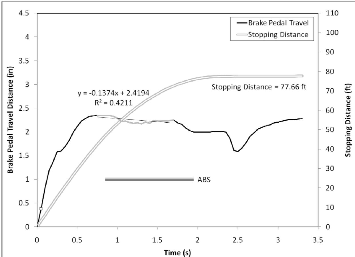
**Figure 133. Brake pedal displacement over the first 3.5 seconds of the R1 panic braking maneuver for Driver 70, an older female driving the Volvo S80**
