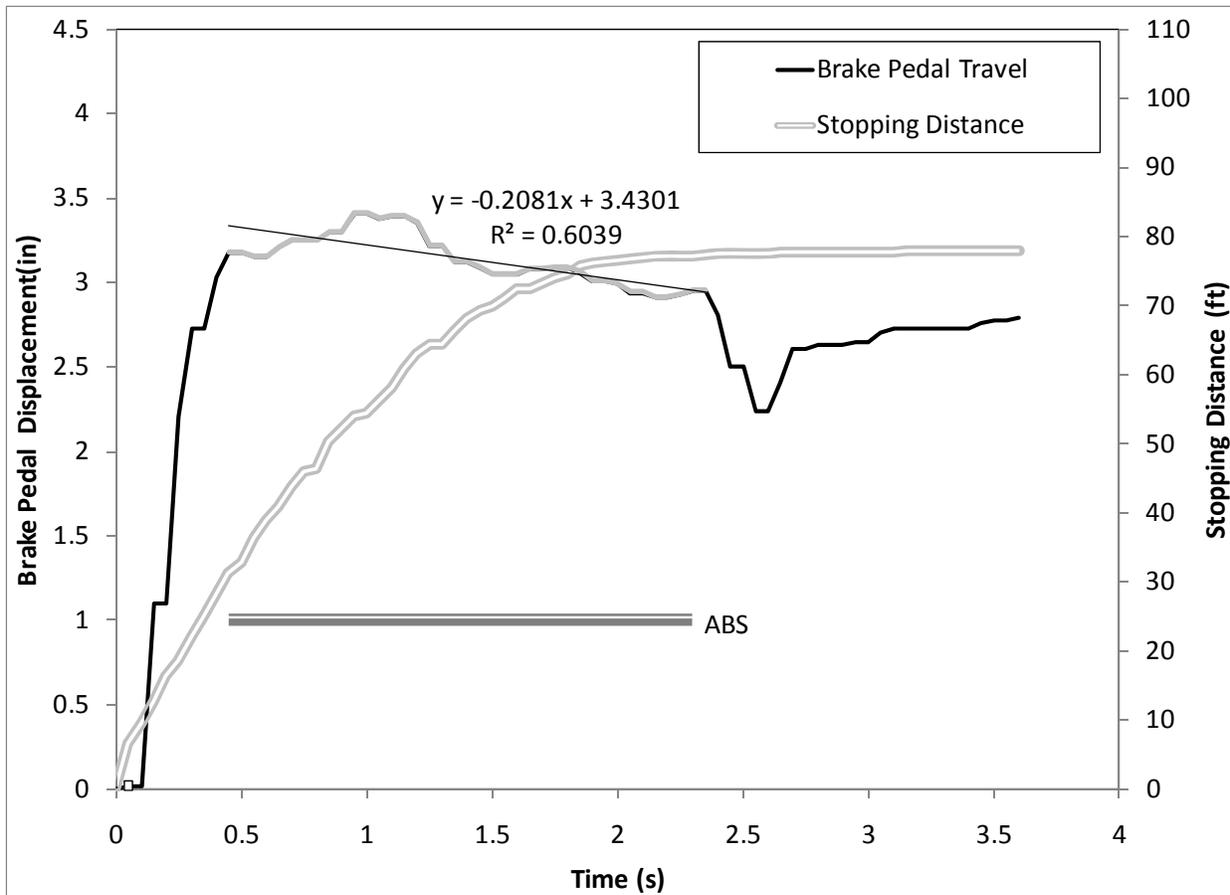
**Figure 42. Driver 10, an Older Male driving the Mercedes-Benz R350, had a Corrected Stopping Distance of 73.98 ft. in the R3 Braking Maneuver**
