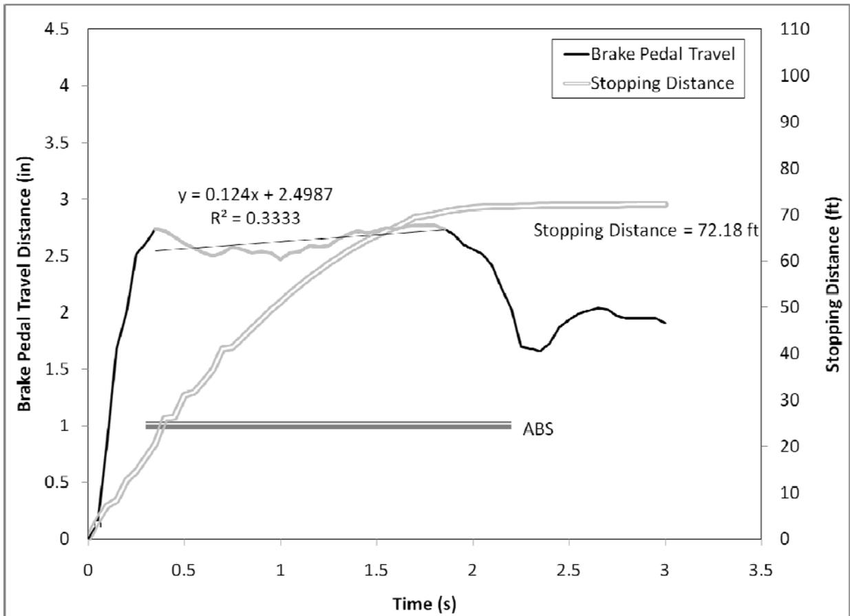
**Figure 128. Brake pedal displacement over the first 3.5 seconds of the R2 panic braking maneuver for Driver 64, a younger male driving the Volvo S80**
