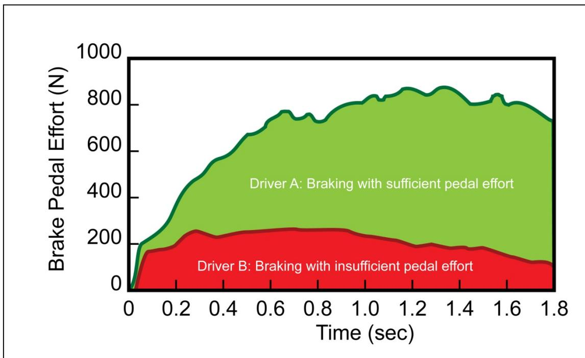
Figure 1. Pedal Effort Plotted Against Time (Adapted from Yoshida et al., 1998)
