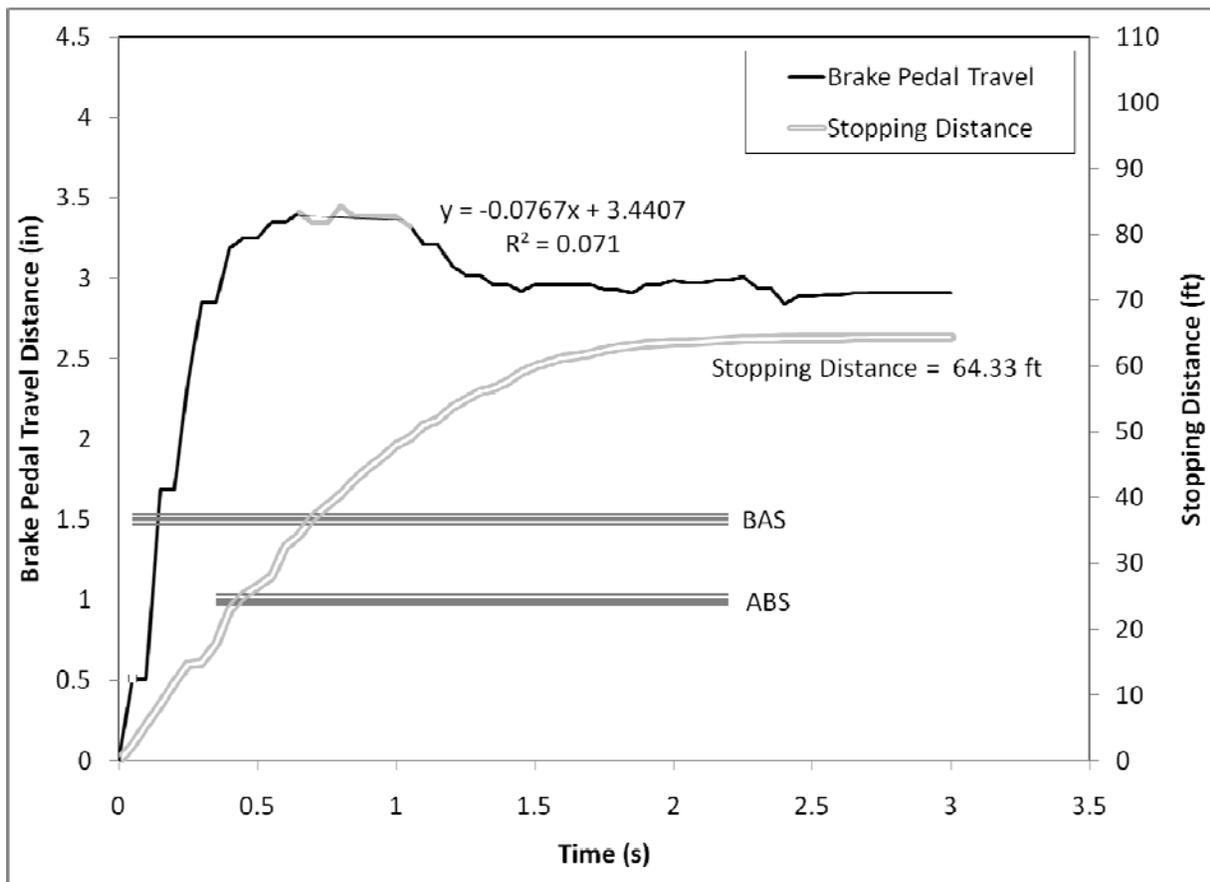
**Figure 102. Brake pedal displacement over the first 3.5 seconds of the R3 panic braking maneuver for Driver 29, a younger male driving the Mercedes-Benz R350**
