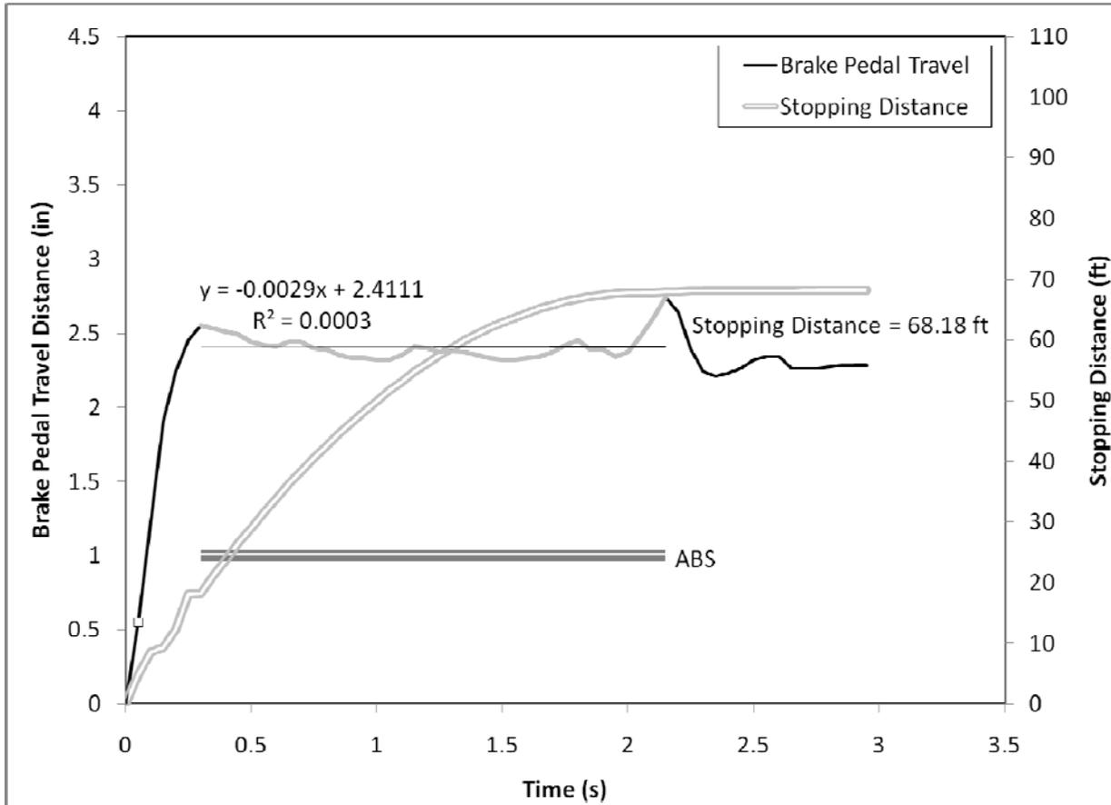
**Figure 115. Brake pedal displacement over the first 3.5 seconds of the R1 panic braking maneuver for Driver 55, a younger female driving the Volvo S80**
