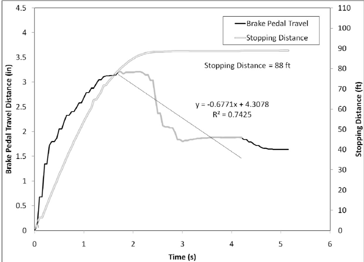
**Figure 80. Driver 25, a younger male driving the Mercedes-Benz R350, did not activate ABS in the braking maneuver.**
