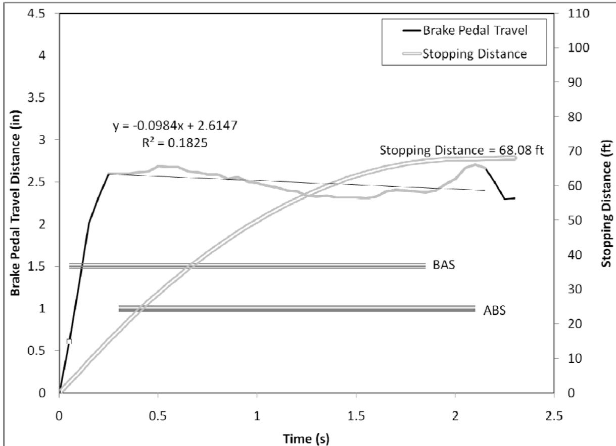
**Figure 118. Brake pedal displacement over the first 2.5 seconds of the R1 panic braking maneuver for Driver 58, a younger male driving the Volvo S80**
