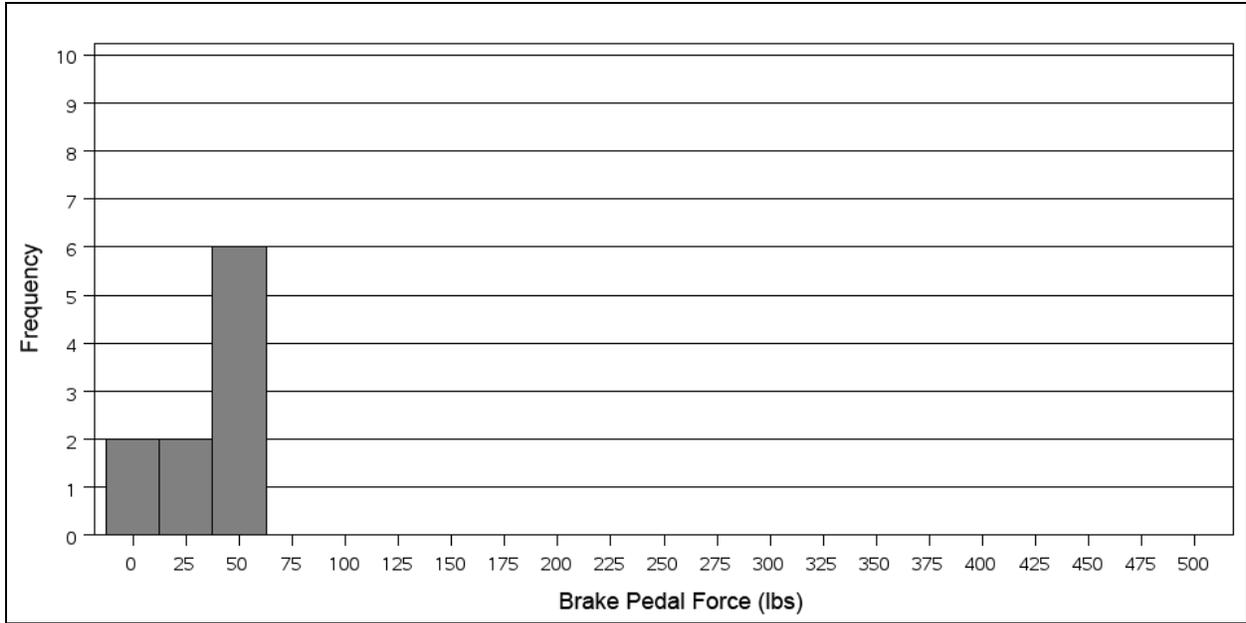
**Figure 50. Distribution of Brake Pedal Forces for Drivers Completing a Stop at an Unexpected Barricade**
