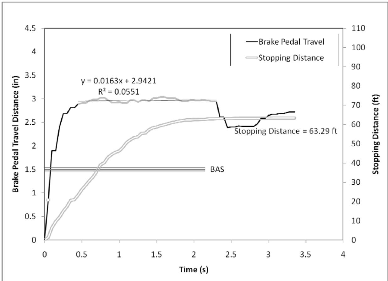
**Figure 98. Brake pedal displacement over the first 4 seconds of the R2 panic braking maneuver for Driver 26, a younger male driving the Mercedes-Benz R350**
