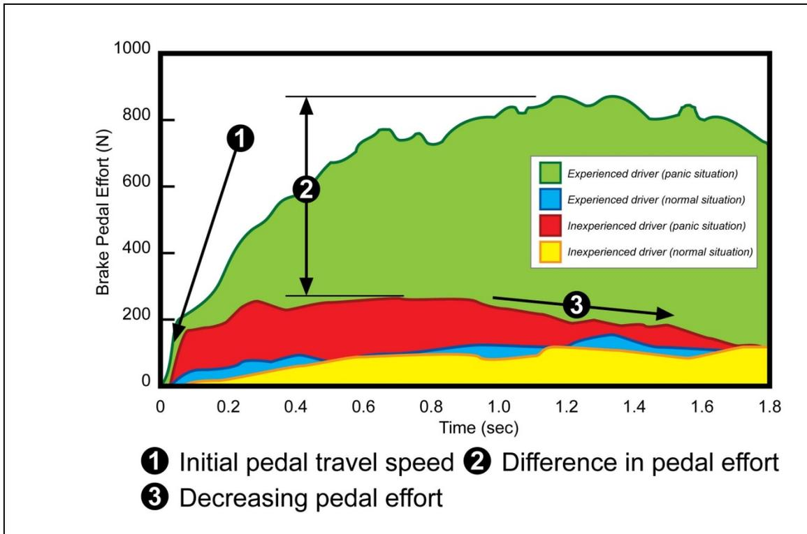
**Figure 2. Pedal Effort Plotted against Time during Panic and Normal Braking (Adapted from Hara, Ohta, Yamamoto, & Yoshida, 1998)**
