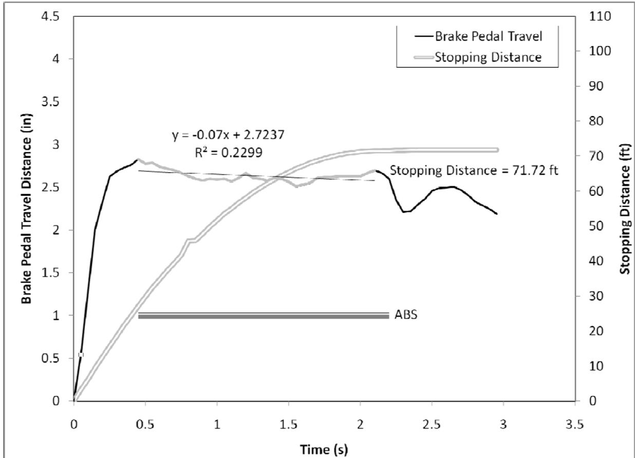
**Figure 121. Brake pedal displacement over the first 3.5 seconds of the R1 panic braking maneuver for Driver 62, a younger male driving the Volvo S80**
