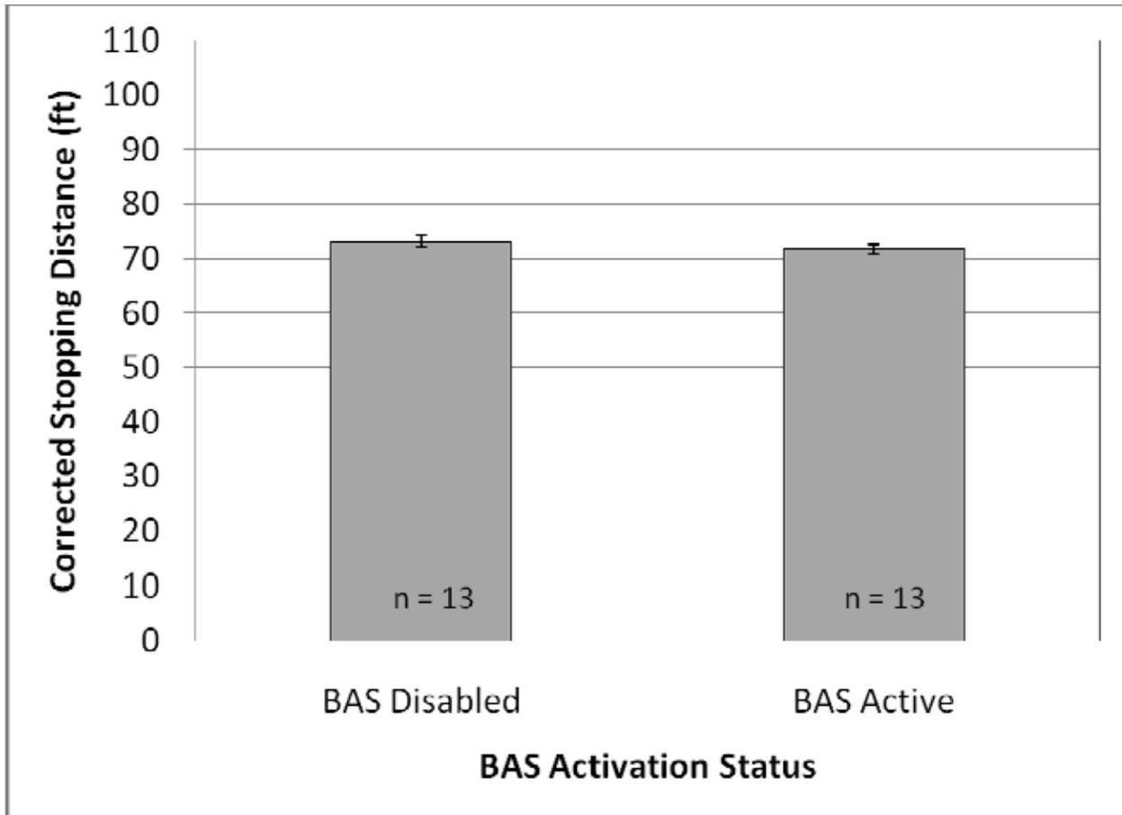
**Figure 40. Average Corrected Stopping Distance by BAS Activation Status for only Drivers that Activated BAS in the Repeated Braking Session**
