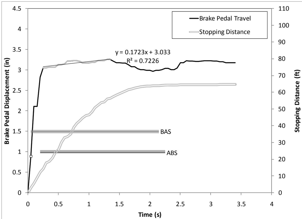
**Figure 41. Driver 10, an Older Male Driving the Mercedes-Benz R350, had a Corrected Stopping Distance of 63.41 ft. in the R2 Braking Maneuver**
