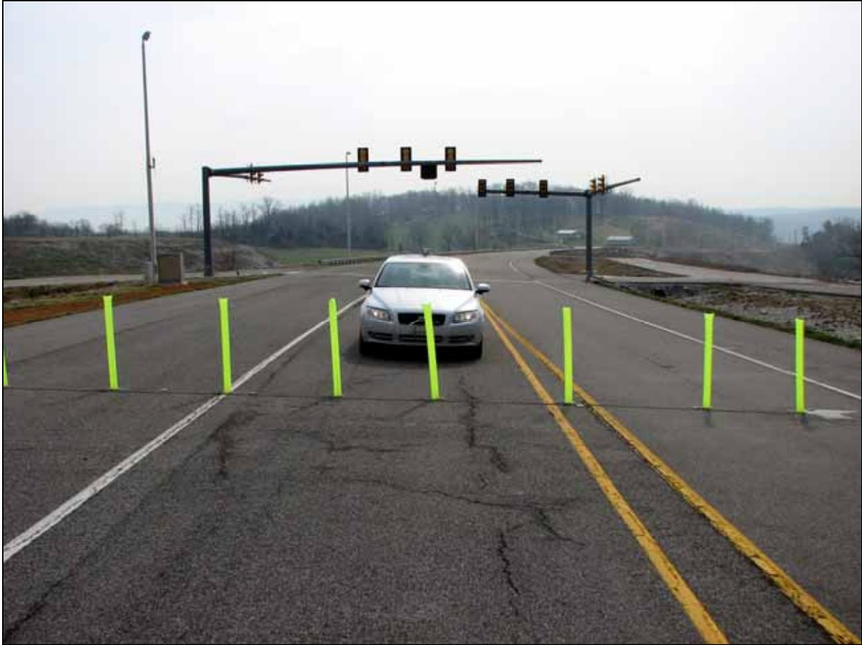
**Figure 35. Inflatable Barricade use for Unexpected Braking Maneuver**
