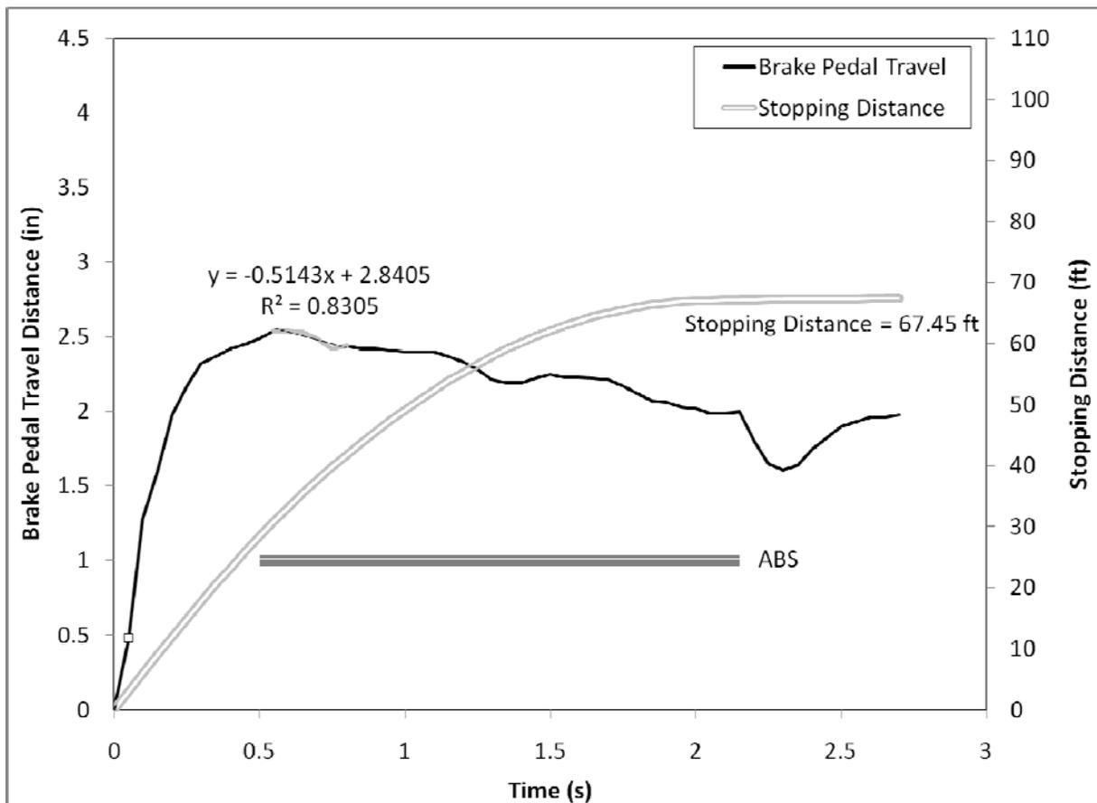
**Figure 135. Brake pedal displacement over the first 3 seconds of the R3 panic braking maneuver for Driver 70, an older female driving the Volvo S80**
