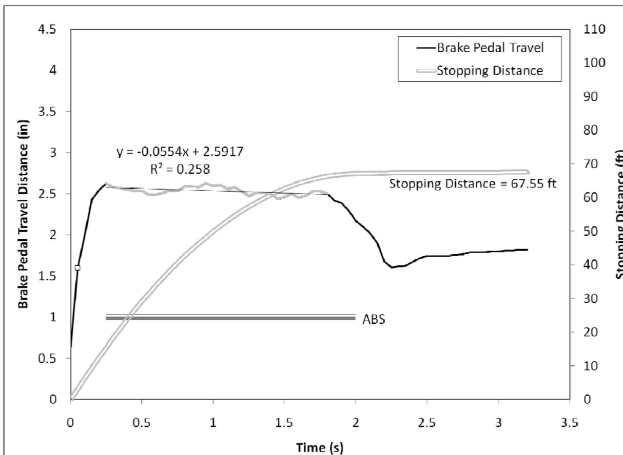
**Figure 122. Brake pedal displacement over the first 3.5 seconds of the R2 panic braking maneuver for Driver 62, a younger male driving the Volvo S80**
