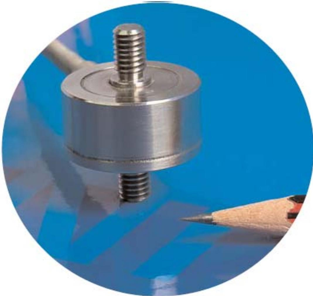
**Figure 62. Load Cell used in the study**
