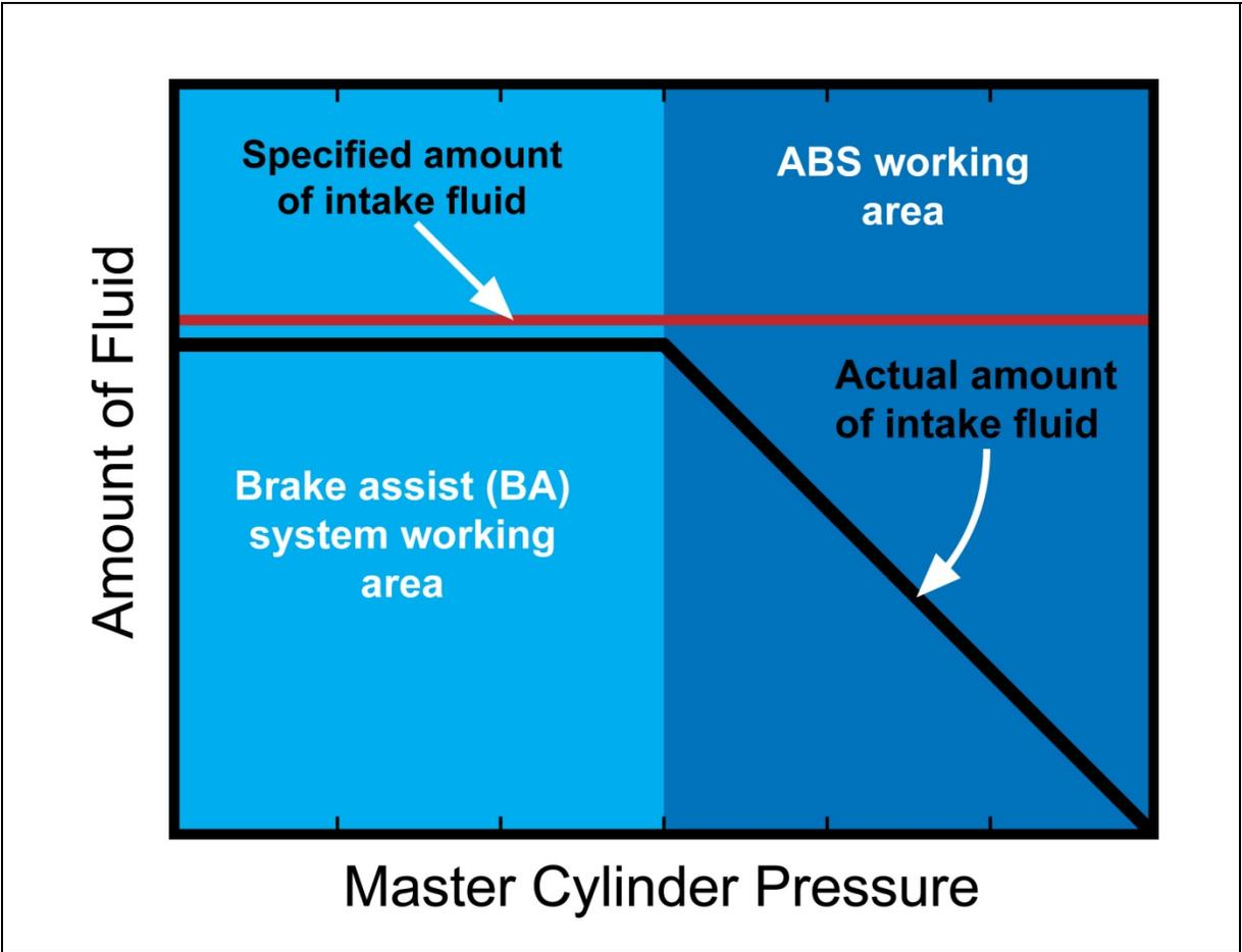
**Figure 9. Illustration of how the Regulation of Intake Fluid Depends on the Master Cylinder Pressure at the Start of Braking (Adapted from Hara, Ohta, Yamamoto, & Yoshida, 1998)**
