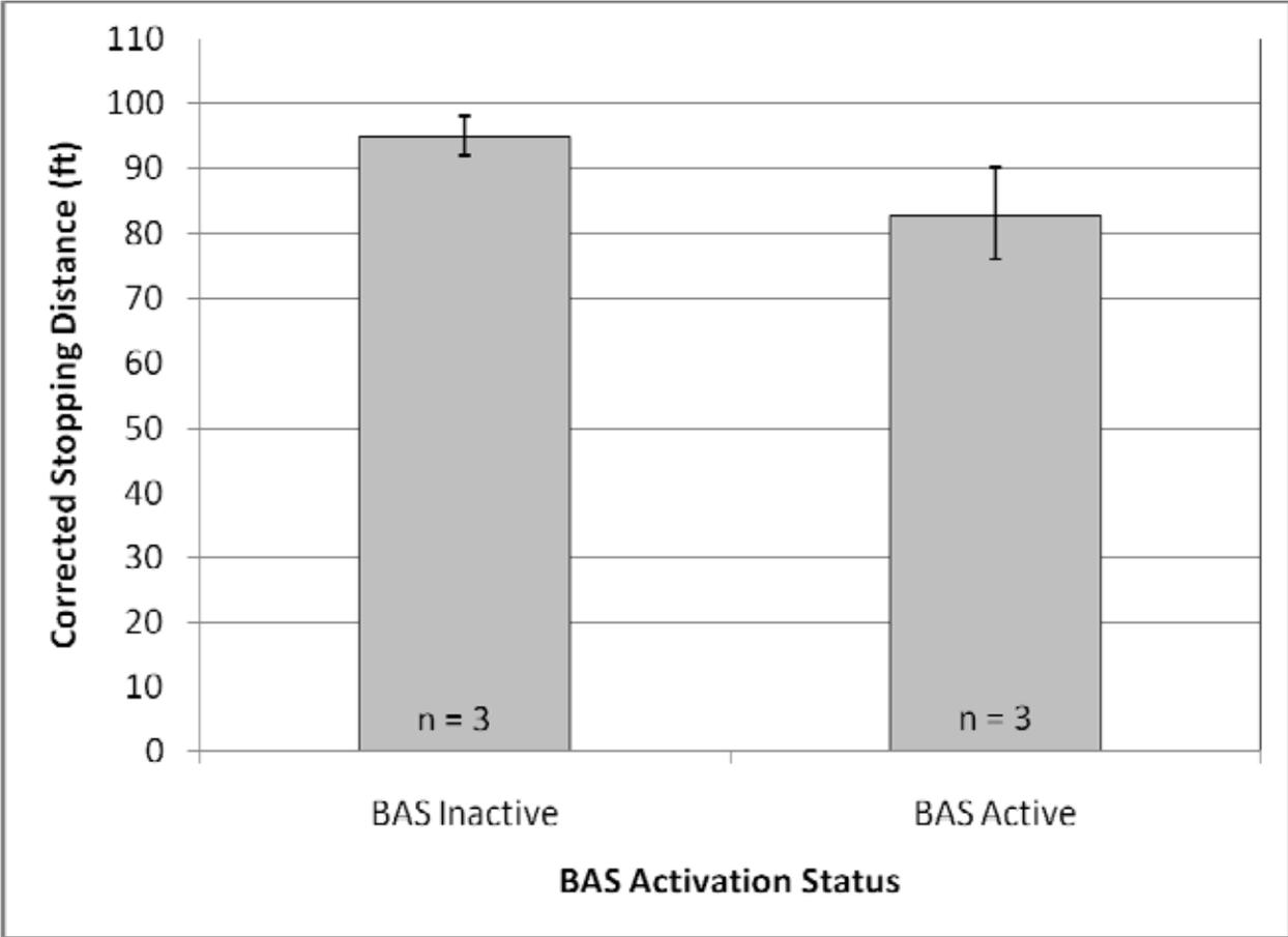
**Figure 36. Average Stopping Distance by BAS Activation. All BAS Activations in the Anticipated Braking Maneuver Occurred using the Volvo S80**
