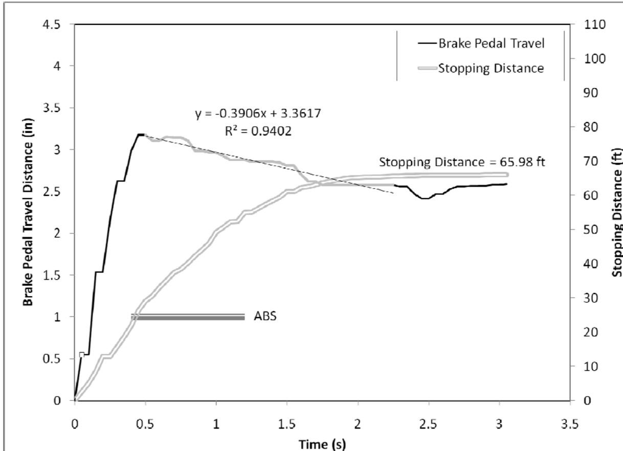
**Figure 100. Brake pedal displacement over the first 3.5 seconds of the R1 panic braking maneuver for Driver 29, a younger male driving the Mercedes-Benz R350**
