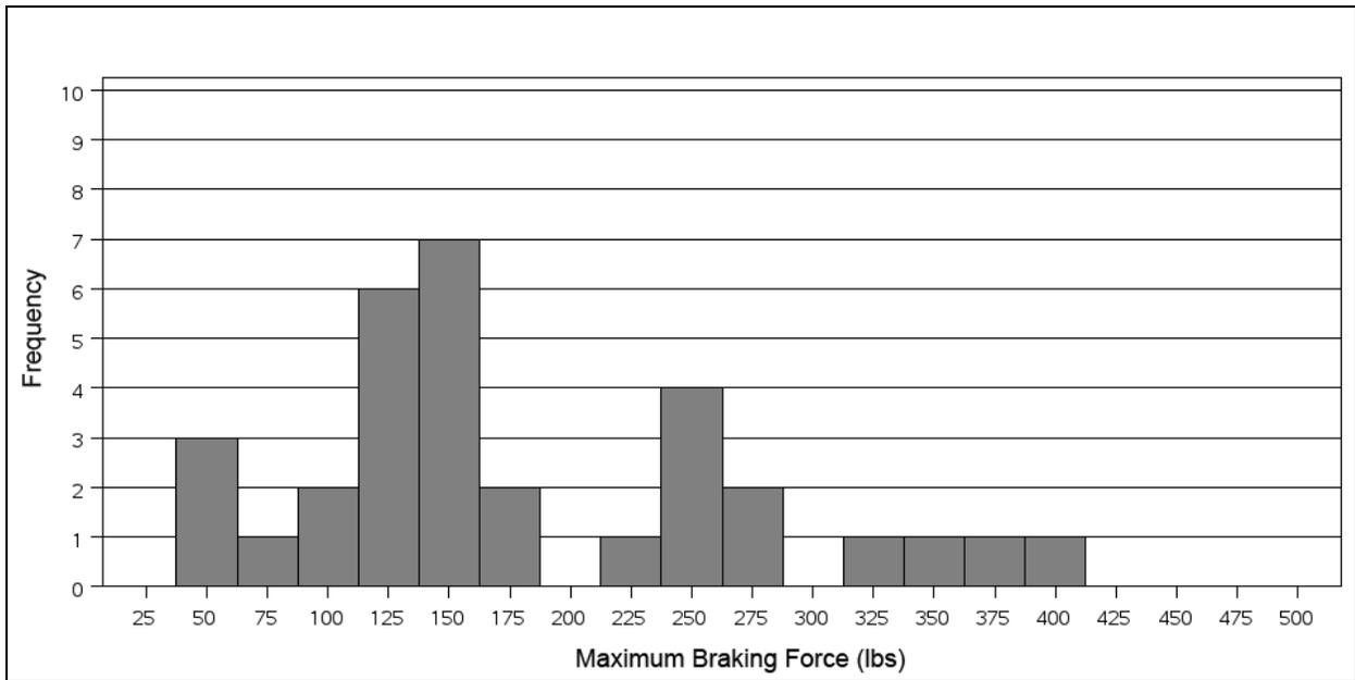
**Figure 48. Maximum Brake Pedal Force for Drivers Assigned to the Mercedes-Benz R350**
