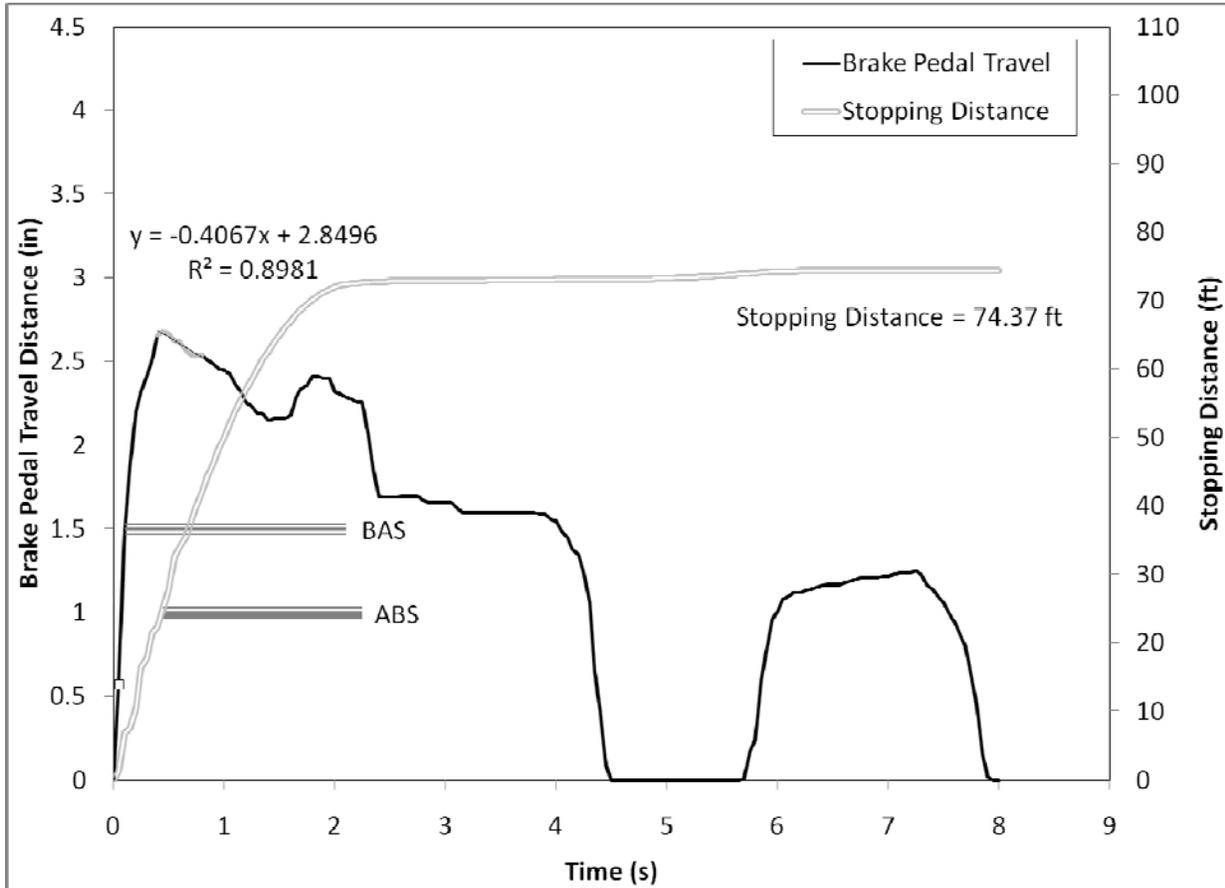
**Figure 86. Driver 48, an older male driving the Volvo S80, activated BAS 0.1 second into the anticipated braking maneuver.**
