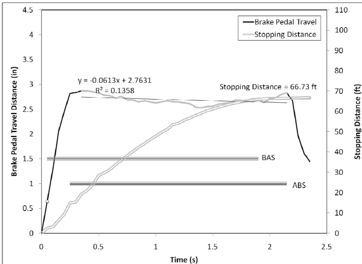
**Figure 126. Brake pedal displacement over the first 2.5 seconds of the R3 panic braking maneuver for Driver 63, a younger male driving the Volvo S80**
