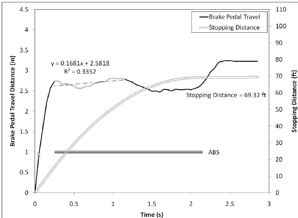
**Figure 120. Brake pedal displacement over the first 3 seconds of the R3 panic braking maneuver for Driver 58, a younger male driving the Volvo S80**
