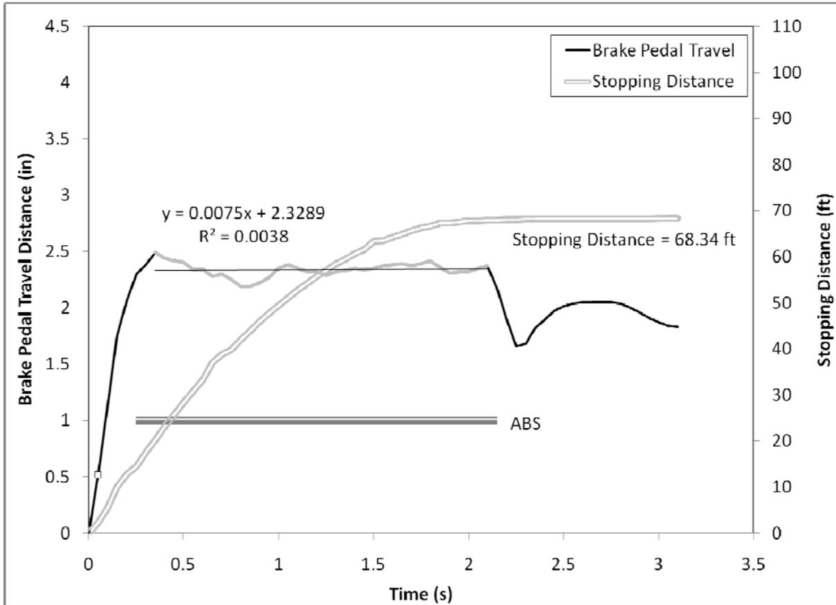
**Figure 127. Brake pedal displacement over the first 3.5 seconds of the R1 panic braking maneuver for Driver 64, a younger male driving the Volvo S80**
