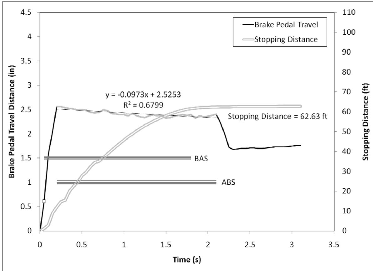
**Figure 109. Brake pedal displacement over the first 3.5 seconds of the R1 panic braking maneuver for Driver 50, a younger female driving the Volvo S80**
