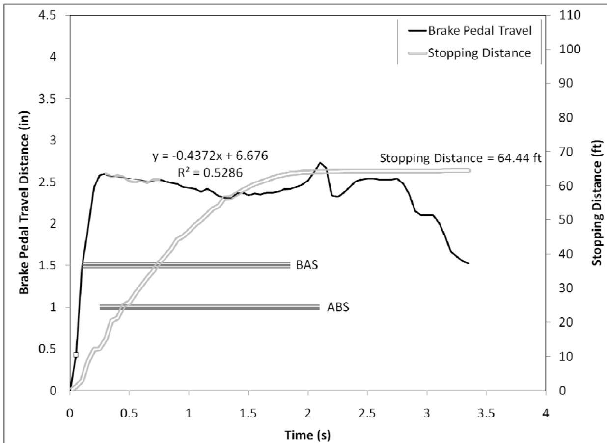
**Figure 117. Brake pedal displacement over the first 4 seconds of the R3 panic braking maneuver for Driver 55, a younger female driving the Volvo S80**
