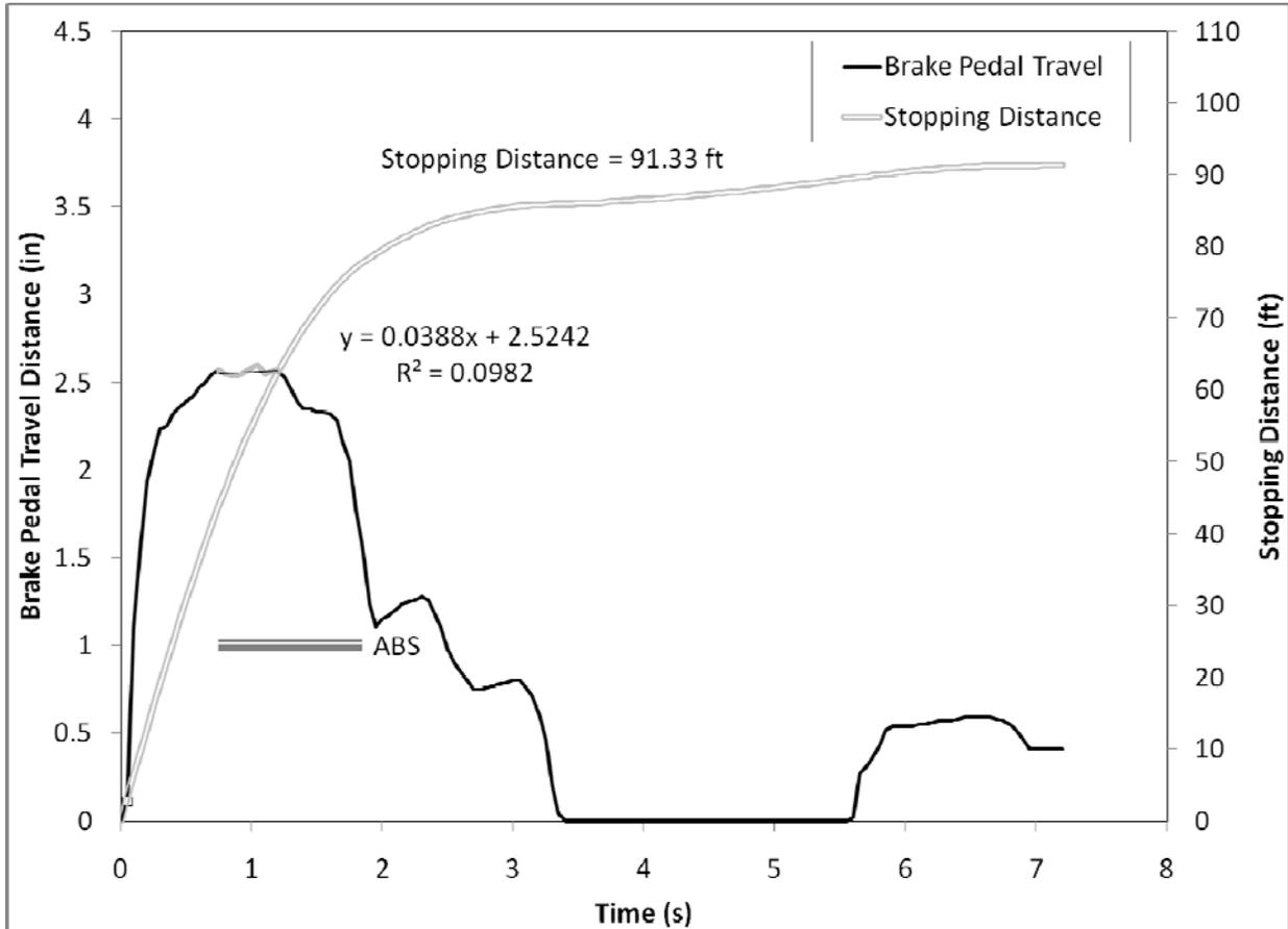
**Figure 89. Driver 69, an older male driving the Volvo S80, did not activate BAS during the anticipated braking maneuver.**
