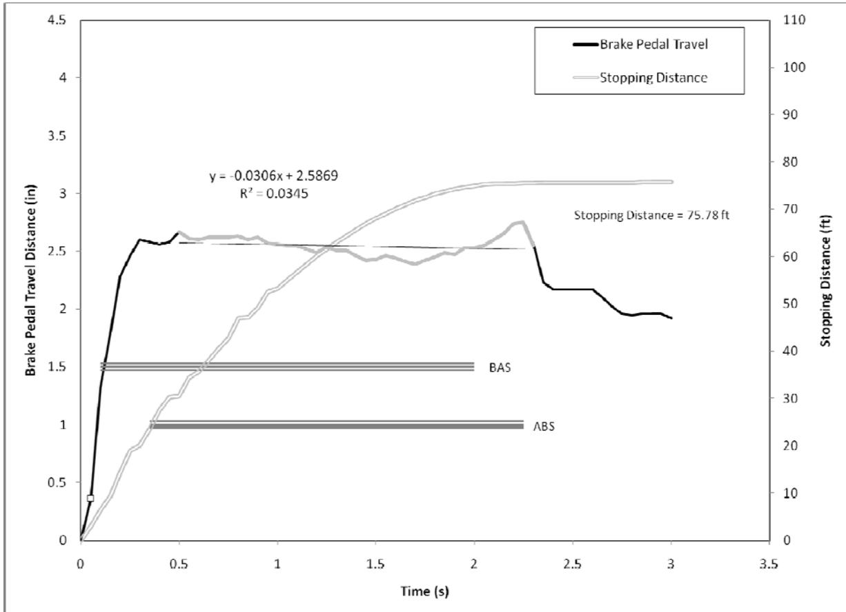
**Figure 85. Driver 44, an older male driving the Volvo S80, activated BAS 0.1 second into the anticipated braking maneuver.**
