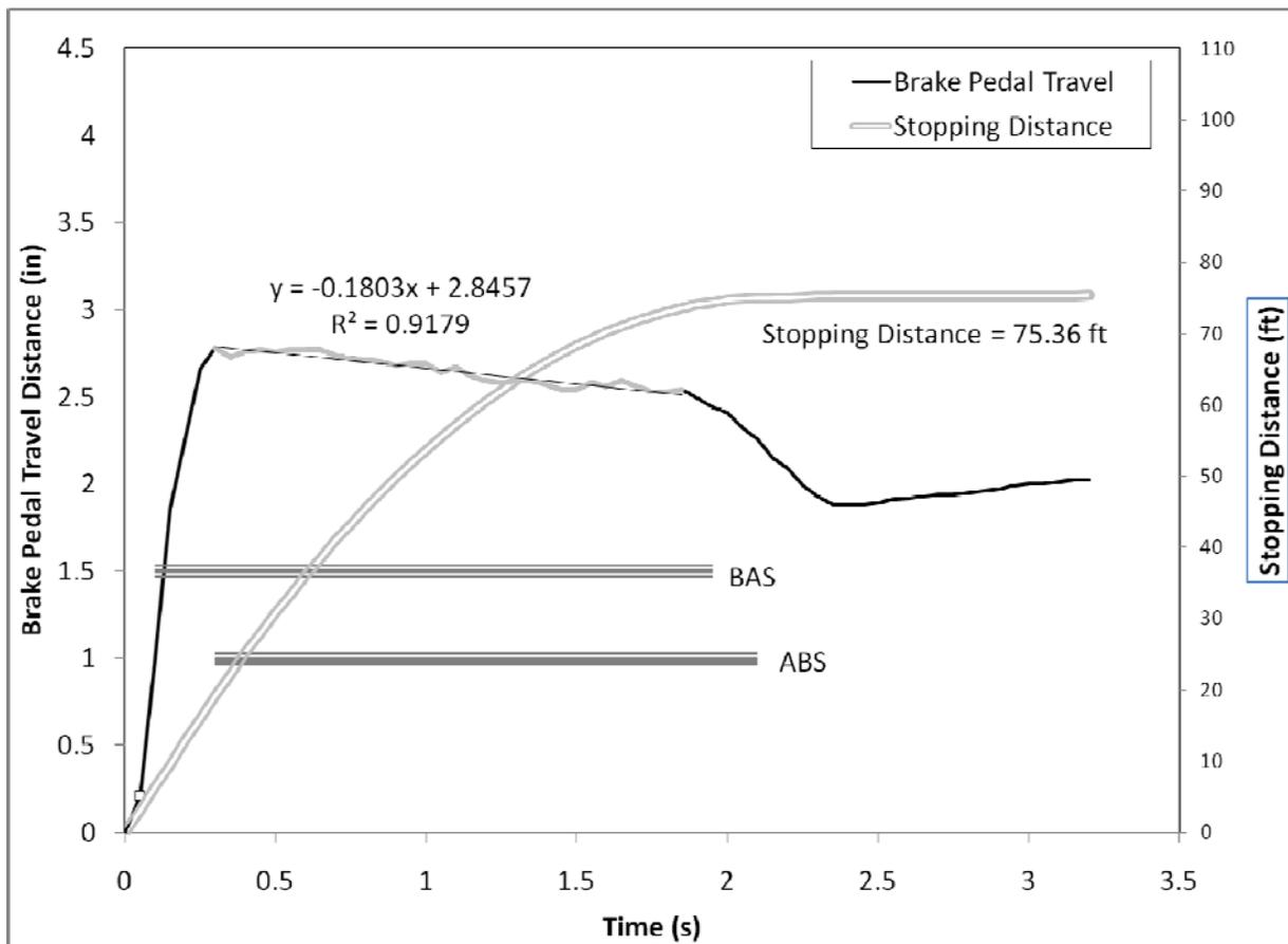
**Figure 123. Brake pedal displacement over the first 3.5 seconds of the R3 panic braking maneuver for Driver 62, a younger male driving the Volvo S80**
