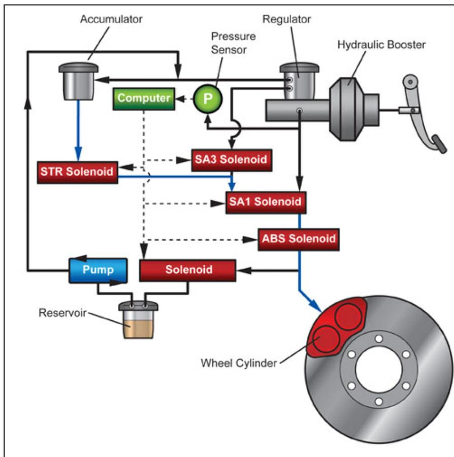
**Figure 7. Hydraulic Servo Brake (Accumulated Pressure Applied) BAS (from Yoshida et al., 1998)**
