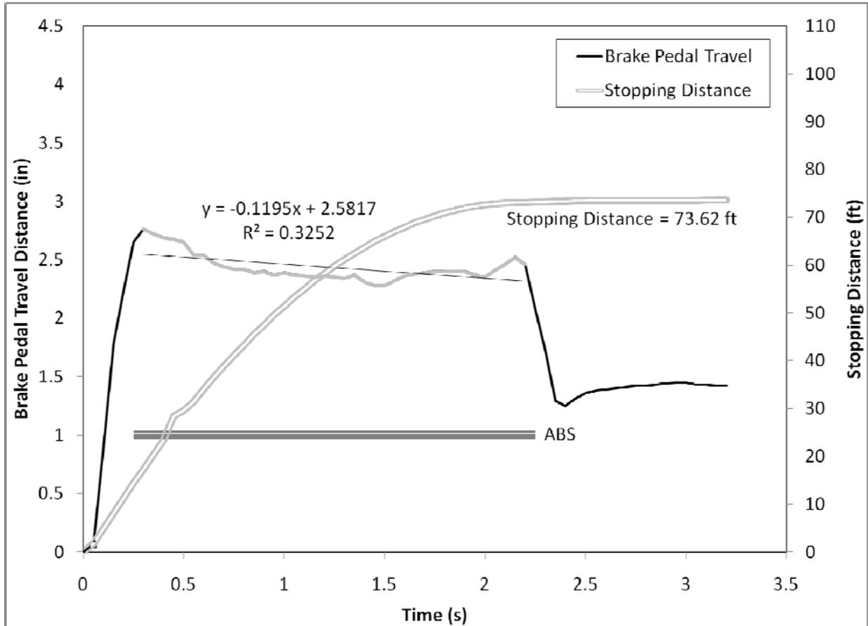
**Figure 94. Brake pedal displacement over the first 3.5 seconds of the R1 panic braking maneuver for Driver 21, a younger female driving the Volvo S80**
