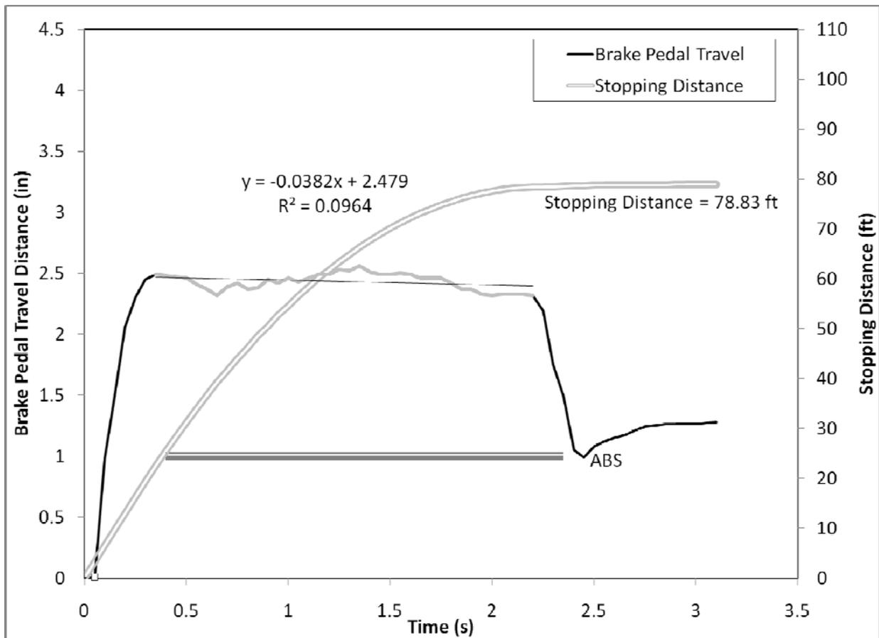
**Figure 95. Brake pedal displacement over the first 3.5 seconds of the R2 panic braking maneuver for Driver 21, a younger female driving the Volvo S80**
