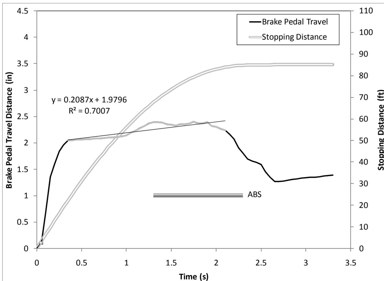
**Figure 44. Driver 65, a Younger Female, Driving the Volvo S80, had a Corrected Stopping Distance of 83.10 ft. in the R3 Braking Maneuver**
