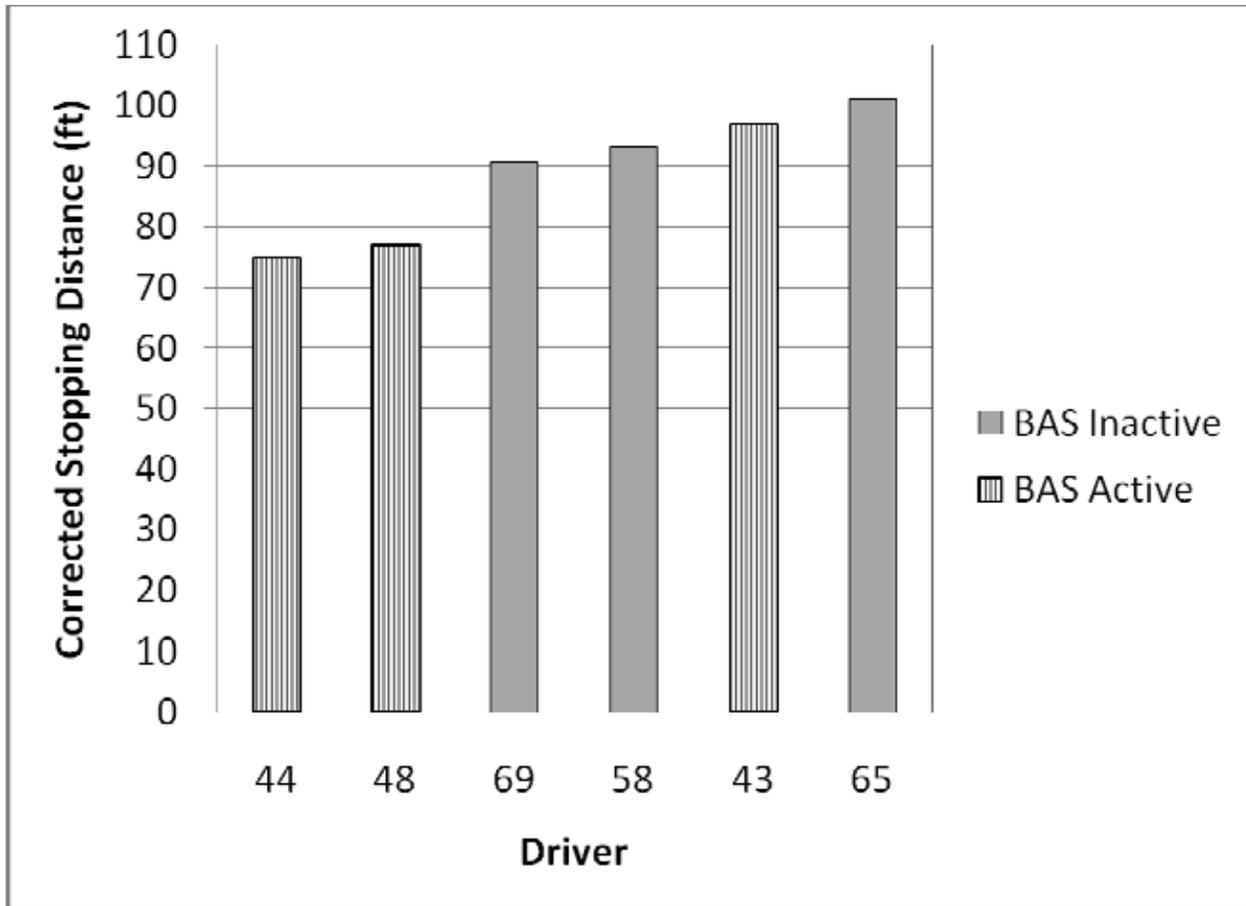
**Figure 37. Corrected Stopping Distances for BAS-Active and BAS-Inactive Stops**
