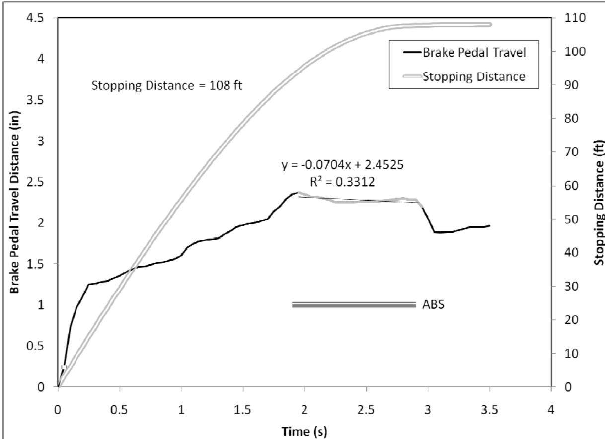
Figure 75. Driver 57, a younger male driving the Volvo S80, activated ABS 1.9 seconds into the panic braking maneuver.
