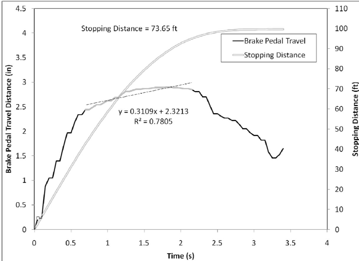
Figure 82. Driver 59, a younger male driving the Mercedes-Benz R350, did not activate ABS in the braking maneuver.
