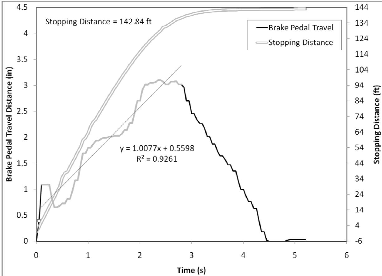
**Figure 78. Driver 19, a younger female driving the Mercedes-Benz R350, did not activate ABS in the braking maneuver.**
