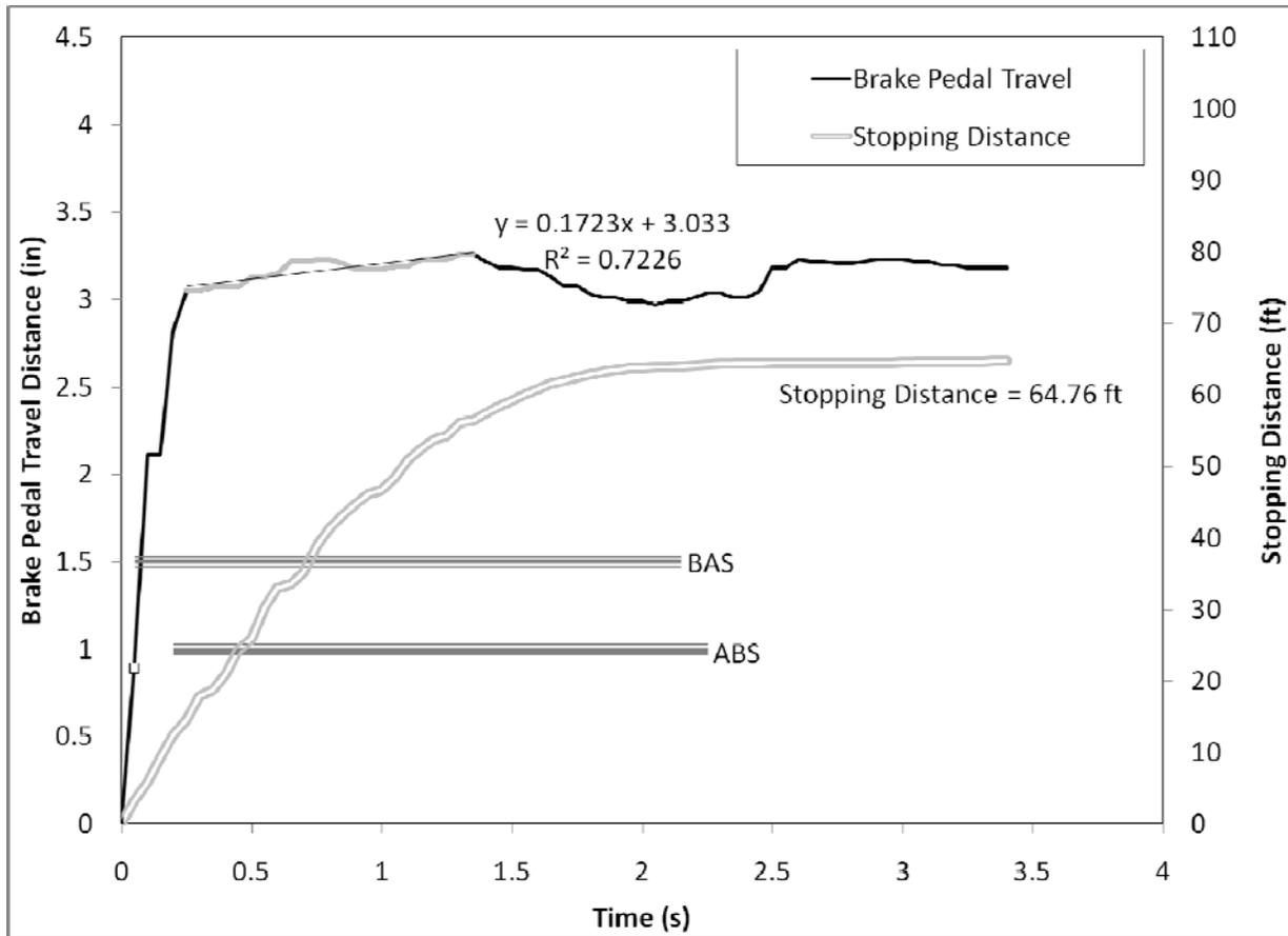
**Figure 92. Brake pedal displacement over the first 4 seconds of the R2 panic braking maneuver for Driver 10, an older male driving the Mercedes-Benz R350**
