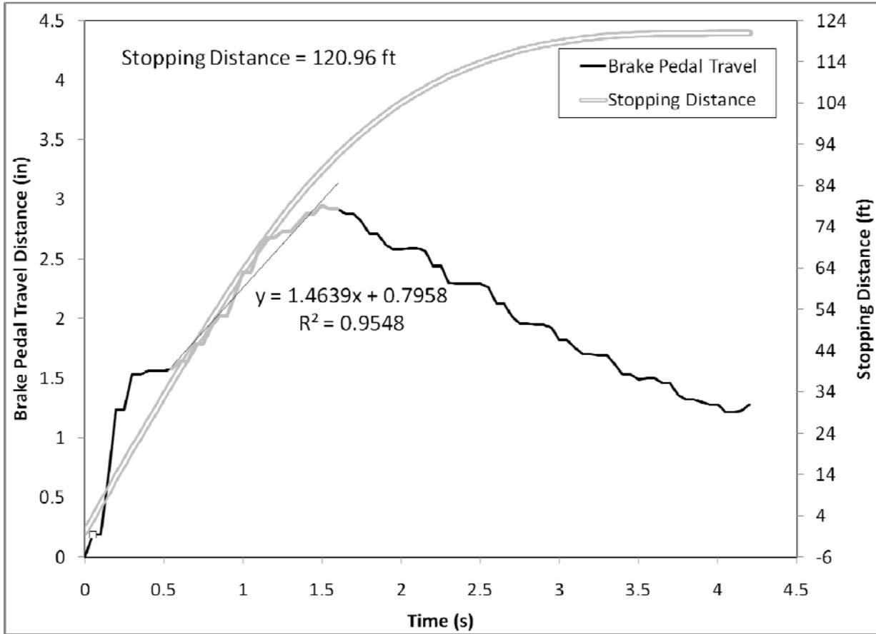
**Figure 79. Driver 23, a younger female driving the Mercedes-Benz R350, did not activate ABS in the braking maneuver.**
