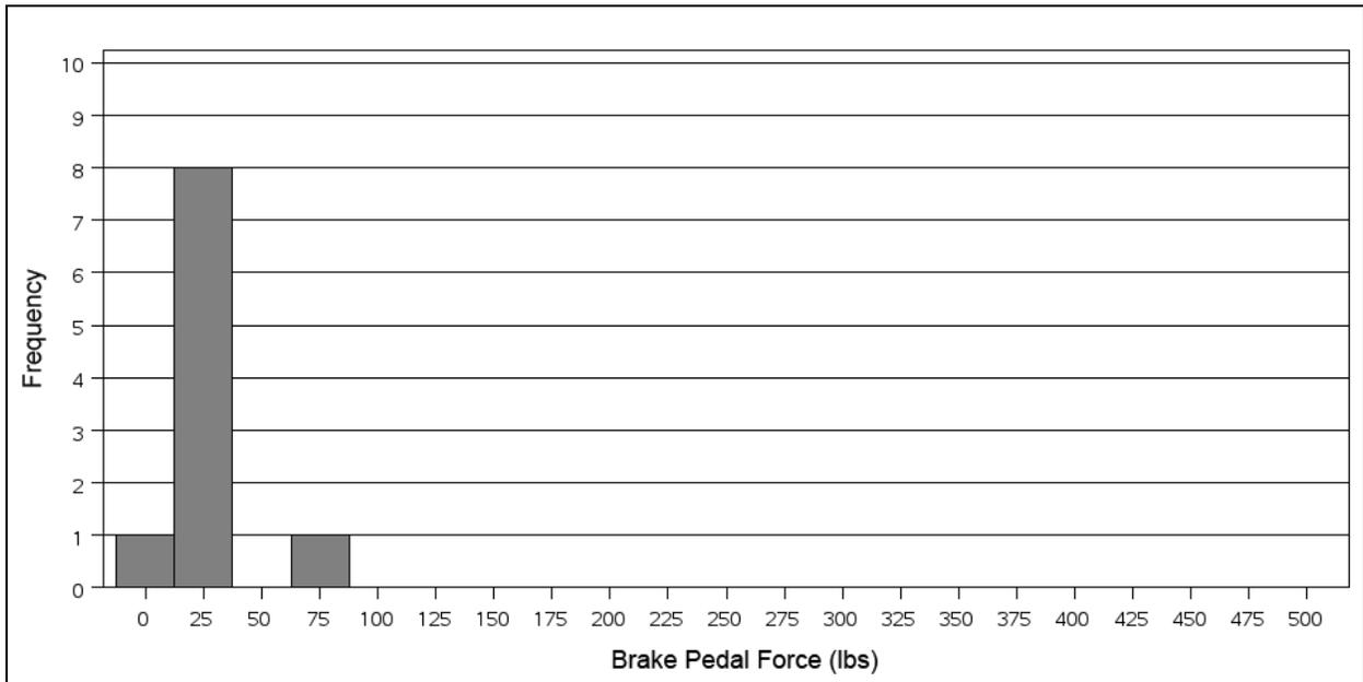
**Figure 51. Distribution of Brake Pedal Forces for Drivers Completing a Stop at an Anticipated Barricade**
