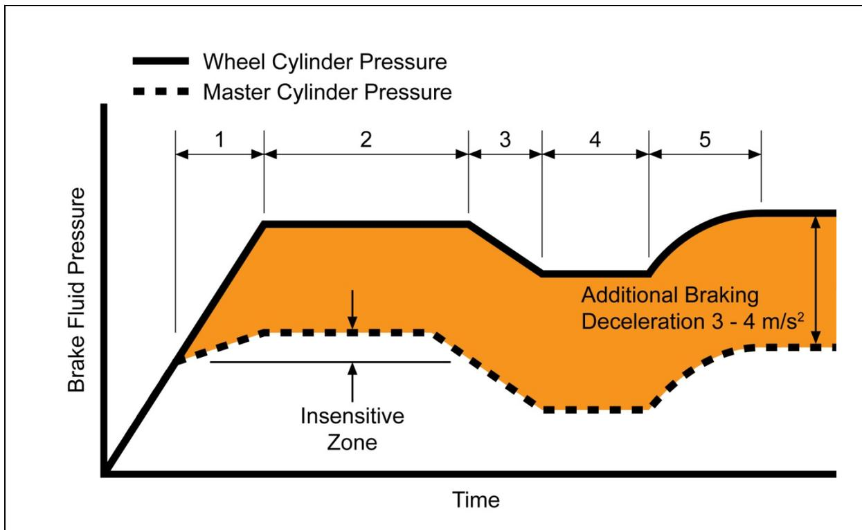
**Figure 3. Pressure Control during Panic Braking (Adapted from Hara, Ohta, Yamamoto, & Yoshida, 1998)**
