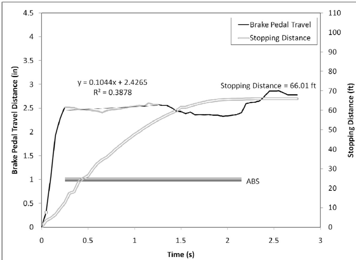
**Figure 116. Brake pedal displacement over the first 3 seconds of the R2 panic braking maneuver for Driver 55, a younger female driving the Volvo S80**
