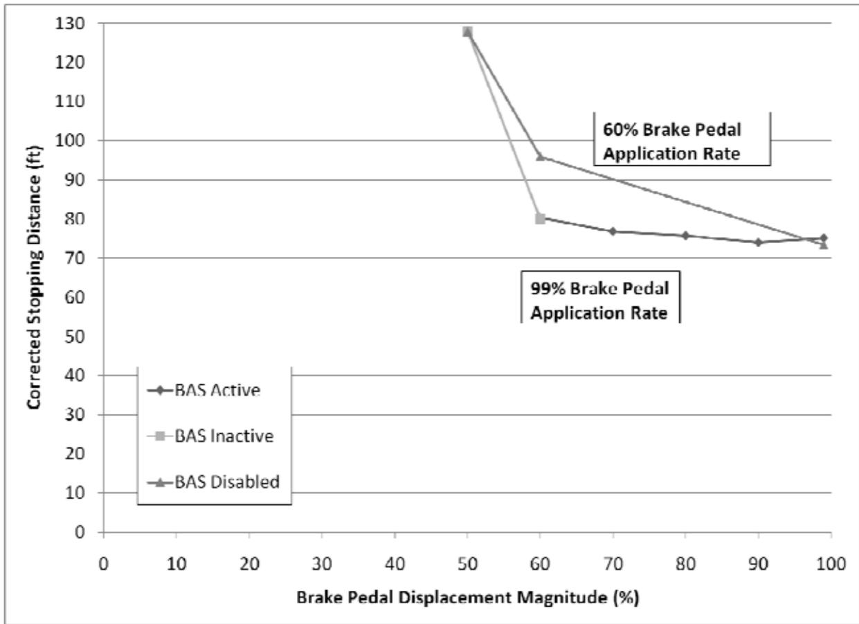
**Figure 18. Operational Envelope for the Mercedes-Benz BAS**
