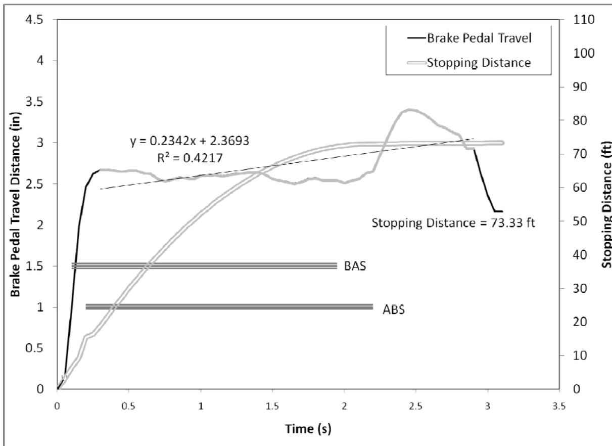
**Figure 107. Brake pedal displacement over the first 3.5 seconds of the R2 panic braking maneuver for Driver 49, a younger male driving the Volvo S80**
