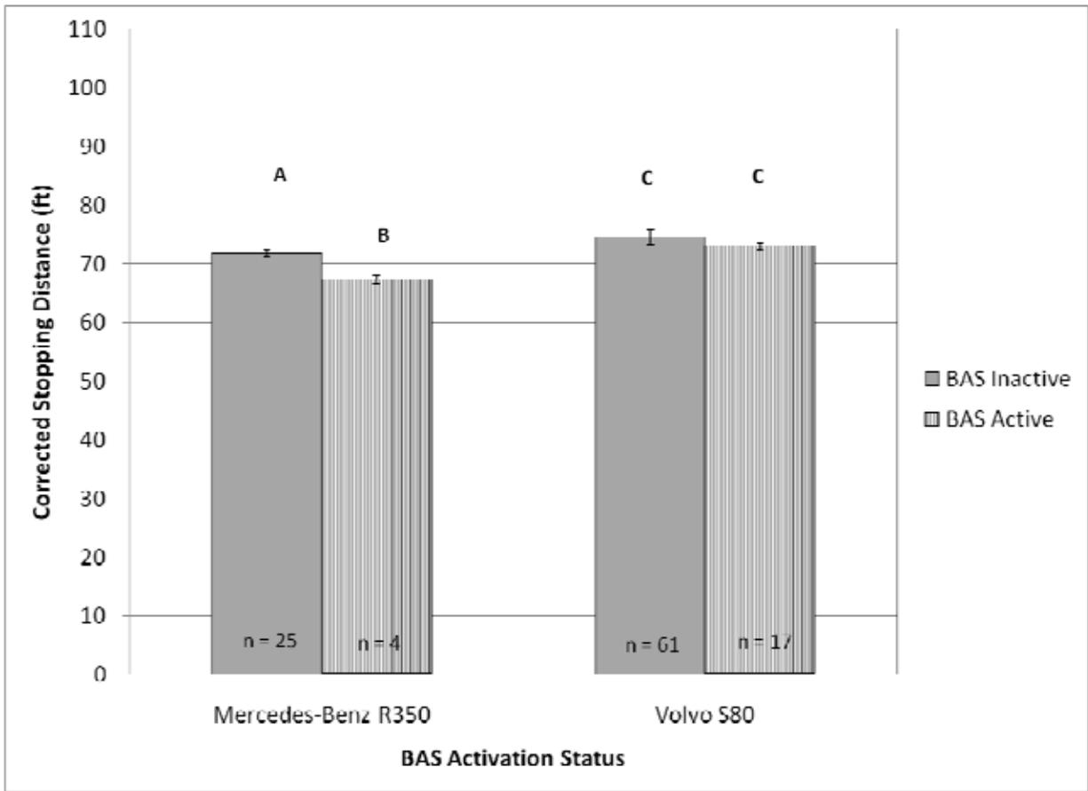
**Figure 47. Mean Corrected Stopping Distances by BAS Activation**
