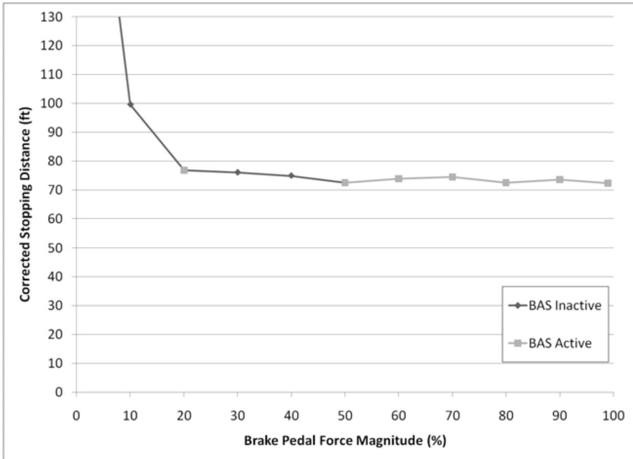
**Figure 16. Corrected Stopping Distance by Brake Pedal Force Magnitude for Tests Performed at 45 mph**
