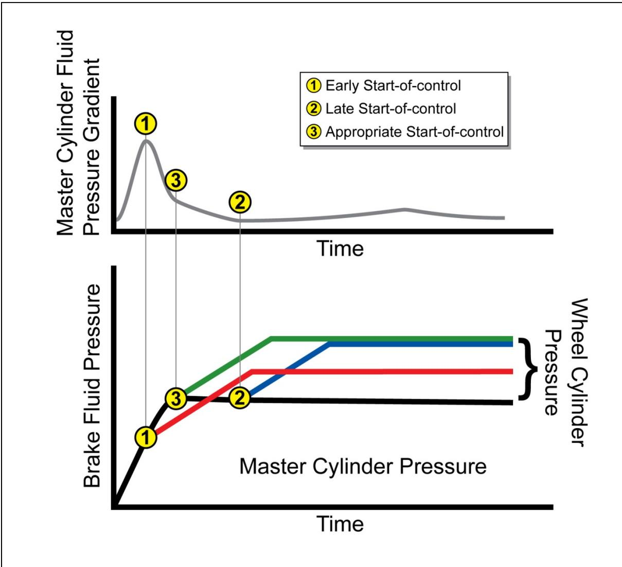
**Figure 8. Timing of BAS Activation by Driver Brake Pedal Input (Adapted from Hara, Ohta, Yamamoto, & Yoshida, 1998)**
