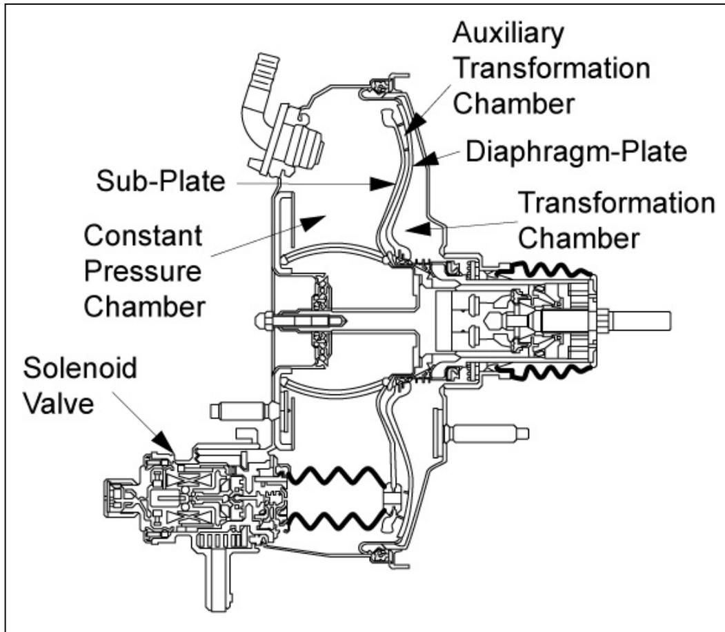
**Figure 5. Components of Vacuum Booster BAS (From Yoshida et al., 1998)**
