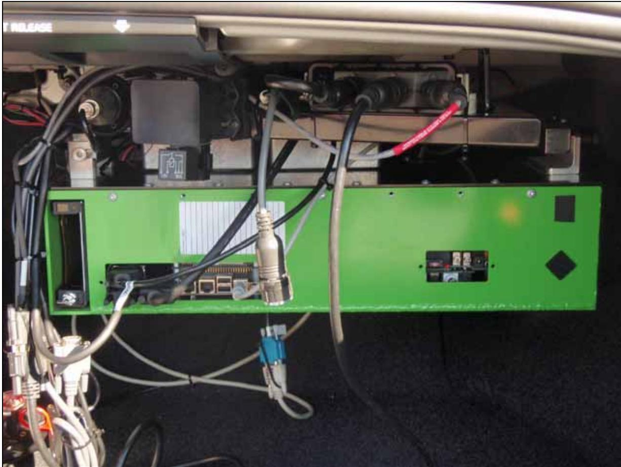
**Figure 25. Data Acquisition System Mounted in the Trunk of the Volvo S80**
