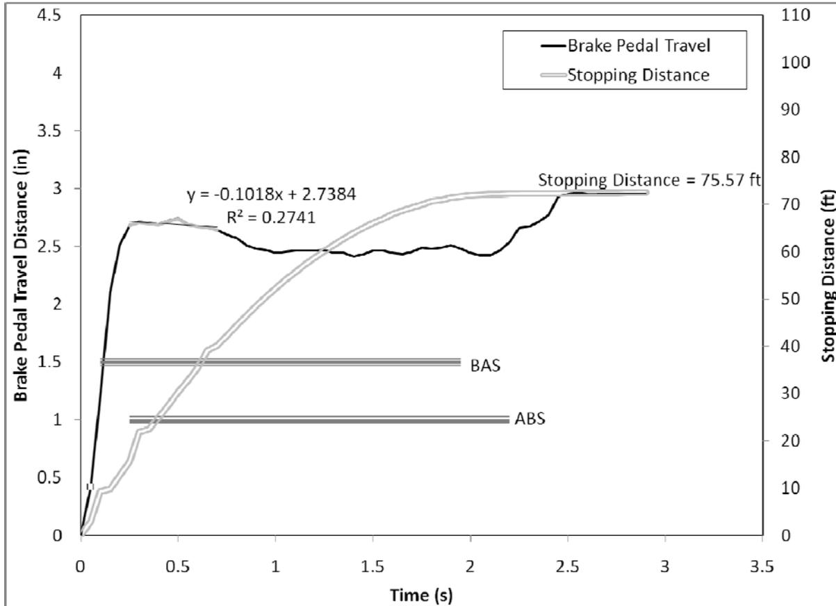
**Figure 106. Brake pedal displacement over the first 3.5 seconds of the R1 panic braking maneuver for Driver 49, a younger male driving the Volvo S80**
