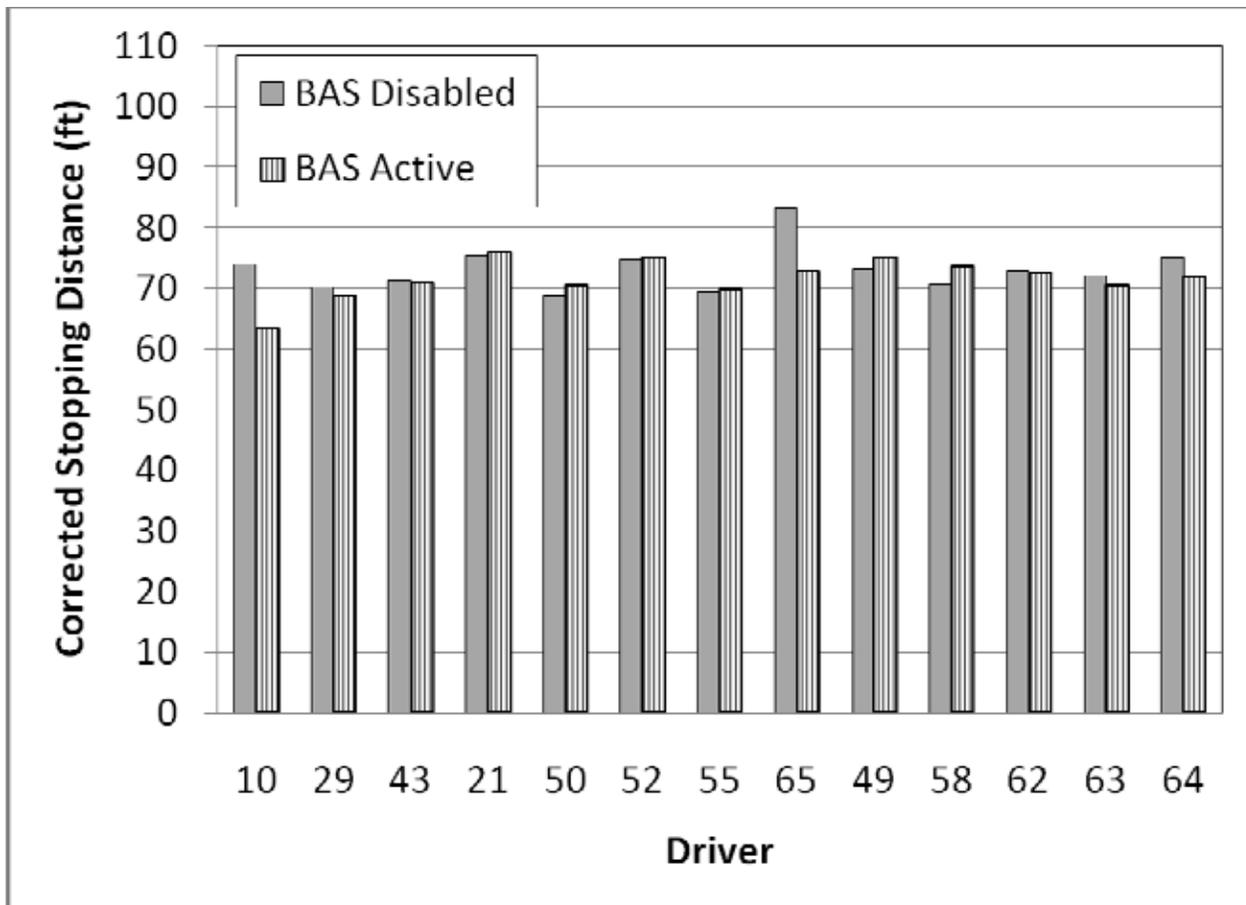
**Figure 39. Corrected Stopping Distances for BAS-Active and BAS-Disabled Braking Maneuvers Produced by Drivers that Activated BAS During the Repeated Braking Session**
