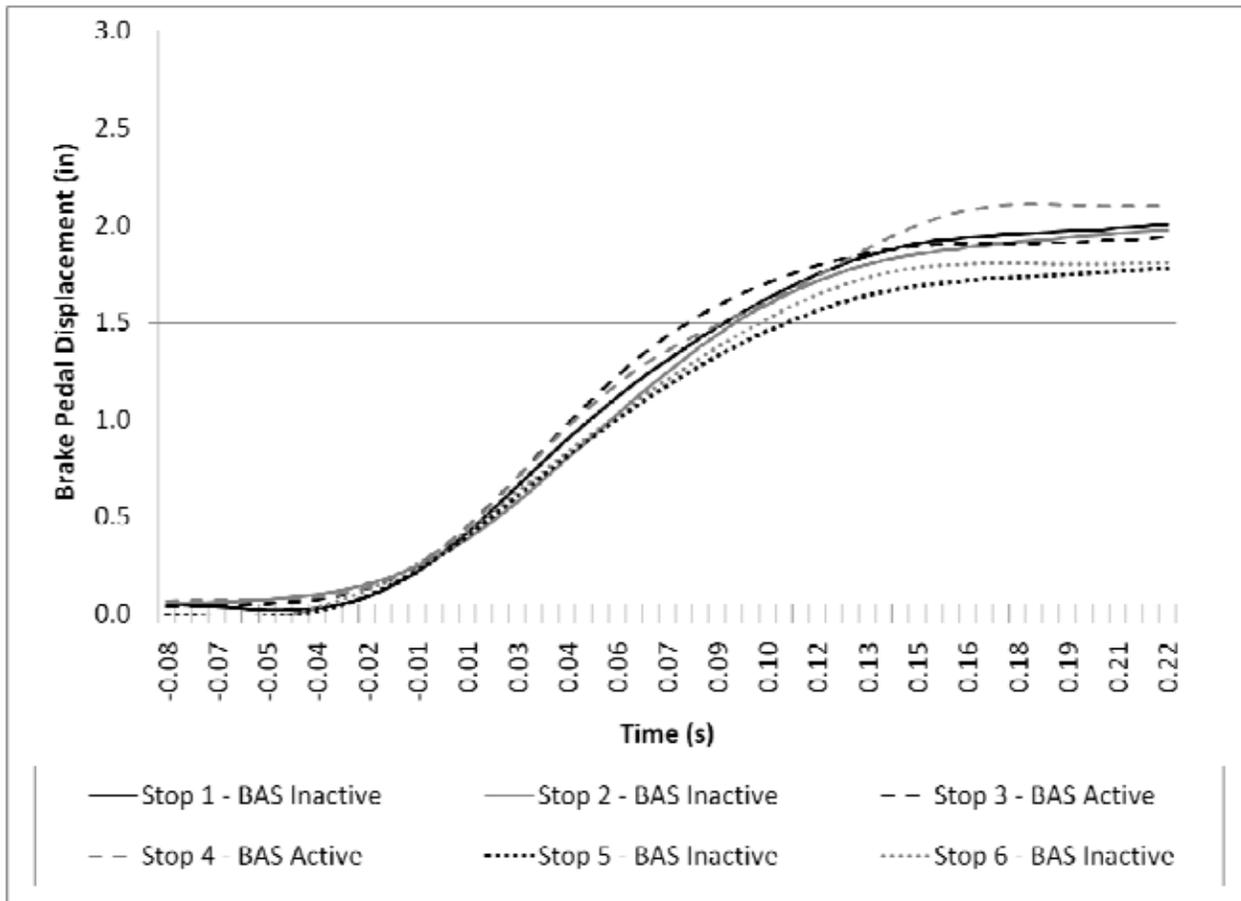
**Figure 23. The brake application rate over the first 0.22 s for all six stops.**
