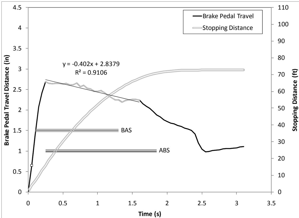
**Figure 43. Driver 65, a Younger Female, Driving the Volvo S80 had a Corrected Stopping Distance of 72.93 ft. in the R1 Braking Maneuver**
