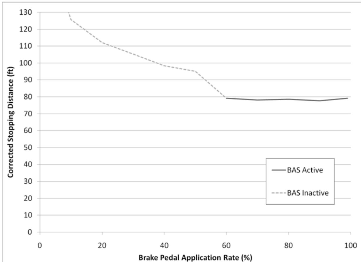
**Figure 15. Corrected Stopping Distance by Brake Pedal Application Rate for Tests Performed at 45 mph**
