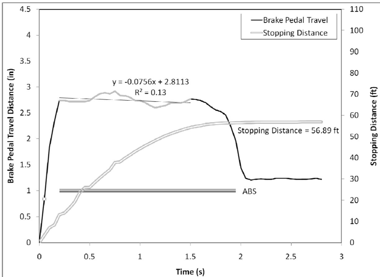
**Figure 125. Brake pedal displacement over the first 3 seconds of the R2 panic braking maneuver for Driver 63, a younger male driving the Volvo S80**
