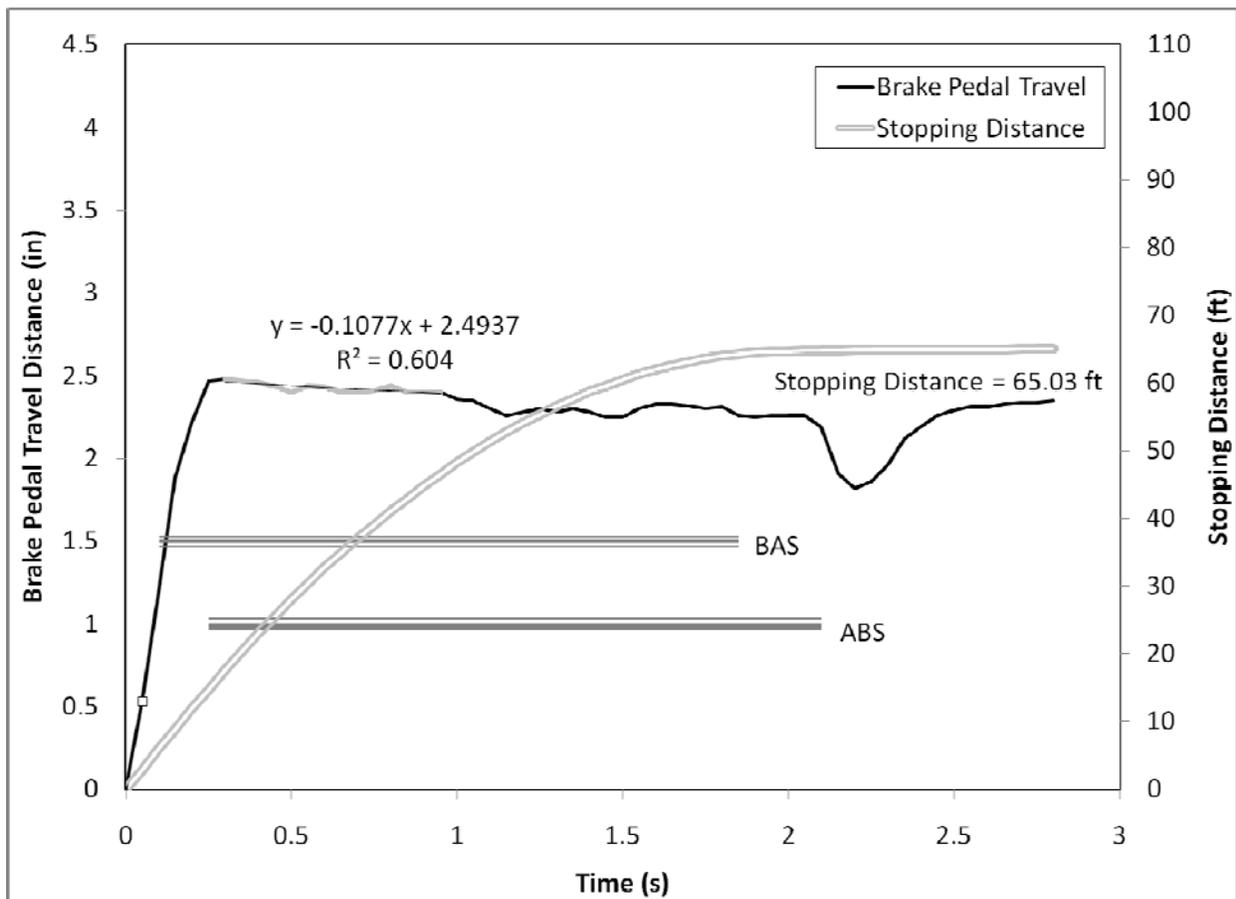
**Figure 134. Brake pedal displacement over the first 3 seconds of the R2 panic braking maneuver for Driver 70, an older female driving the Volvo S80**
