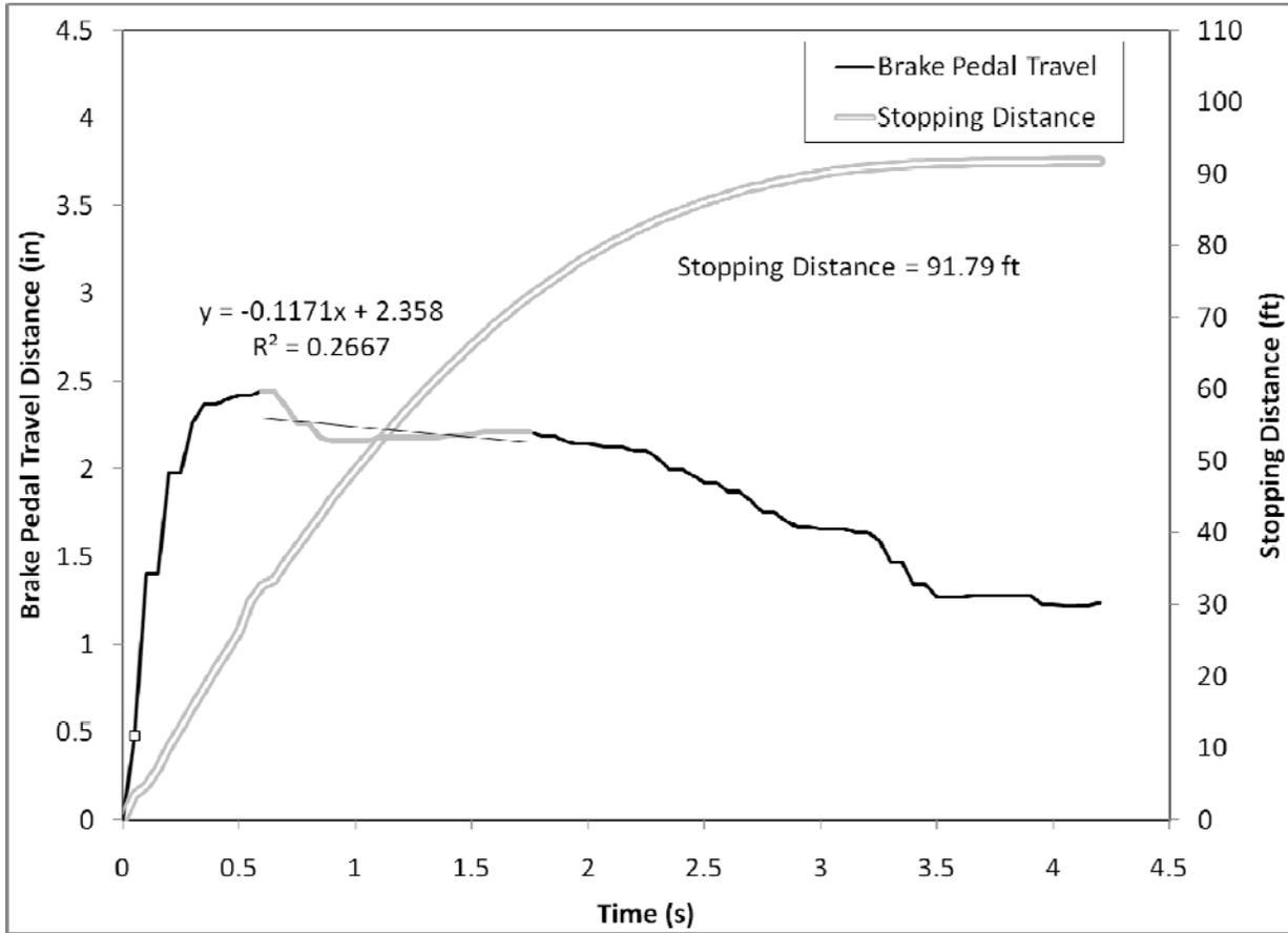
Figure 77. Driver 11, an older male driving the Mercedes-Benz R350, did not activate ABS in the braking maneuver.
