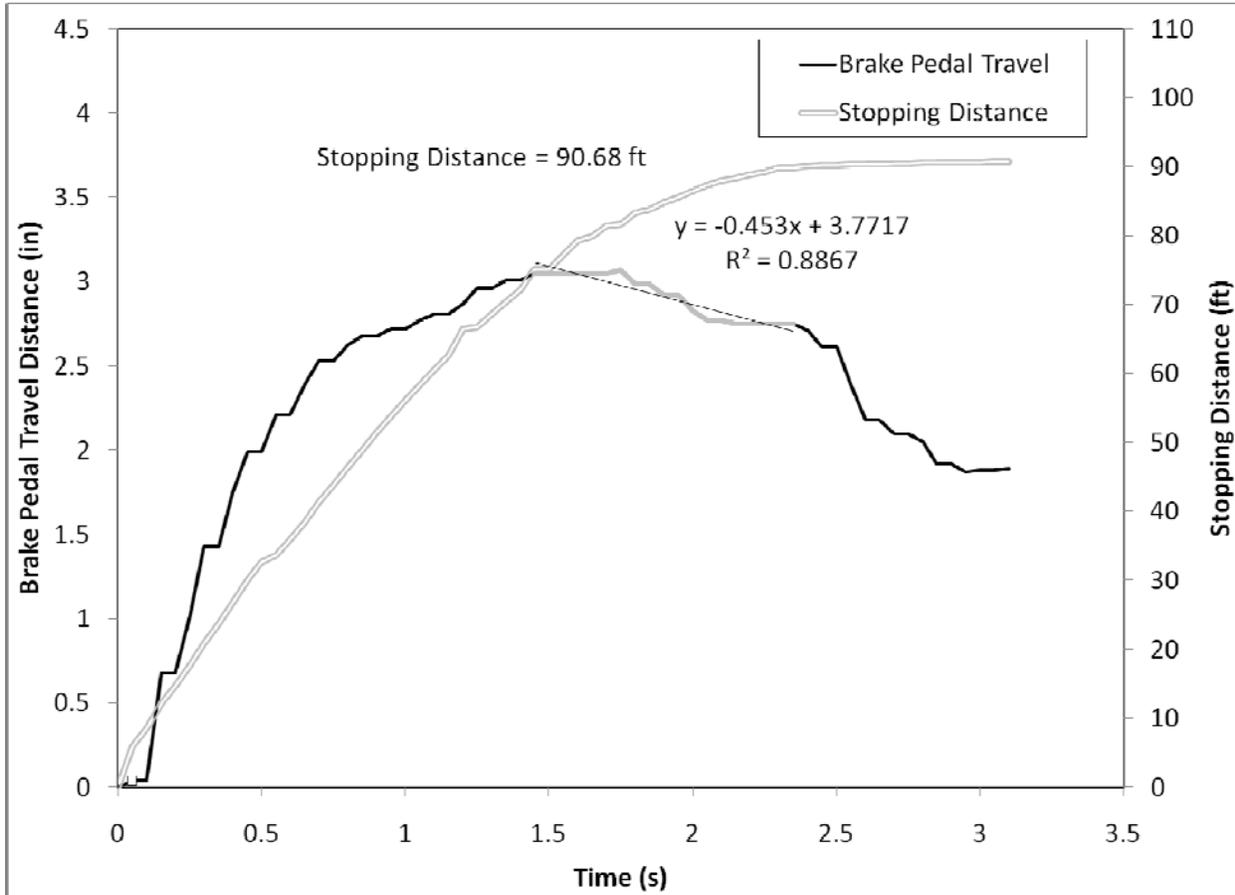
**Figure 81. Driver 29, a younger male driving the Mercedes-Benz R350, did not activate ABS in the braking maneuver.**
