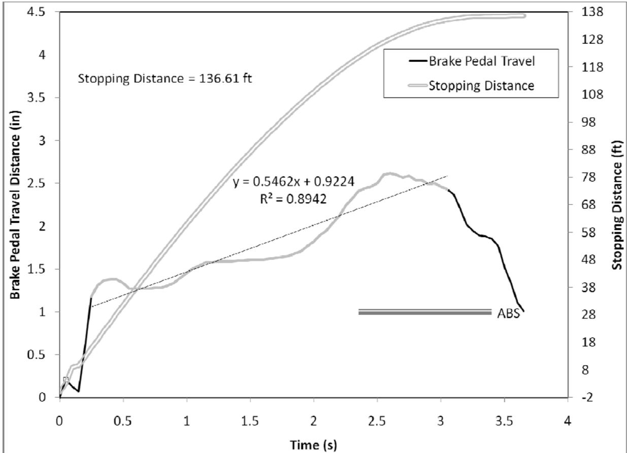
**Figure 72. Driver 44, an older male driving the Volvo S80, activated ABS 2.35 seconds into the panic-braking maneuver.**
