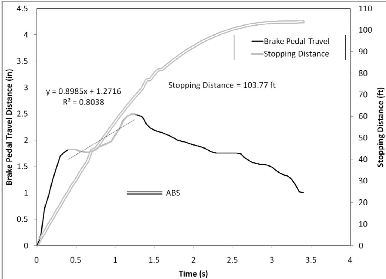
**Figure 74. Driver 53, a younger female driving the Volvo S80, activated ABS 1.15 seconds into the panic-braking maneuver.**
