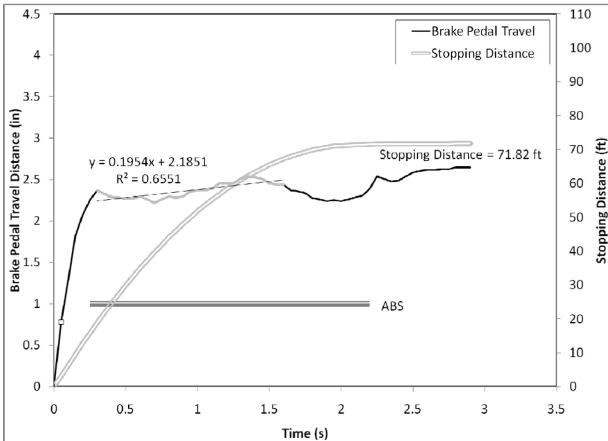
**Figure 119. Brake pedal displacement over the first 3.5 seconds of the R2 panic braking maneuver for Driver 58, a younger male driving the Volvo S80**
