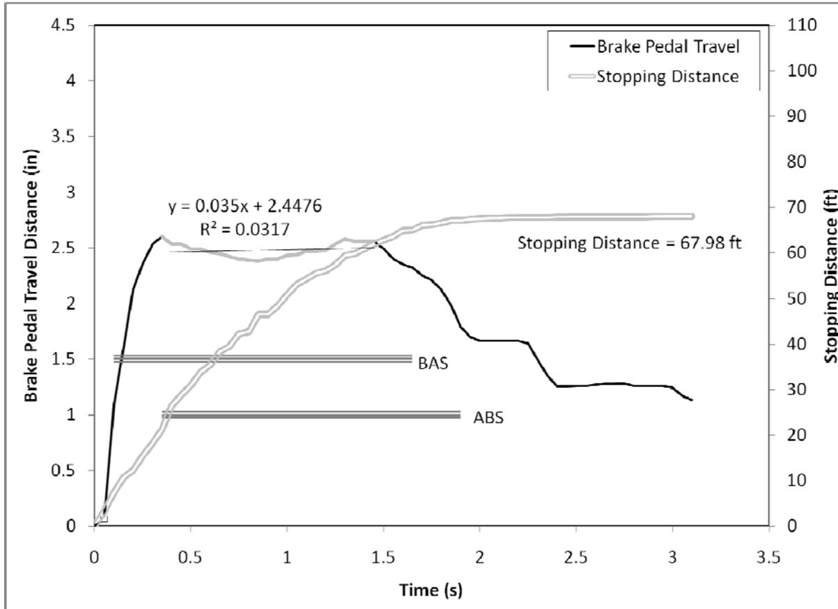
**Figure 112. Brake pedal displacement over the first 3.5 seconds of the R1 panic braking maneuver for Driver 52, a younger female driving the Volvo S80**
