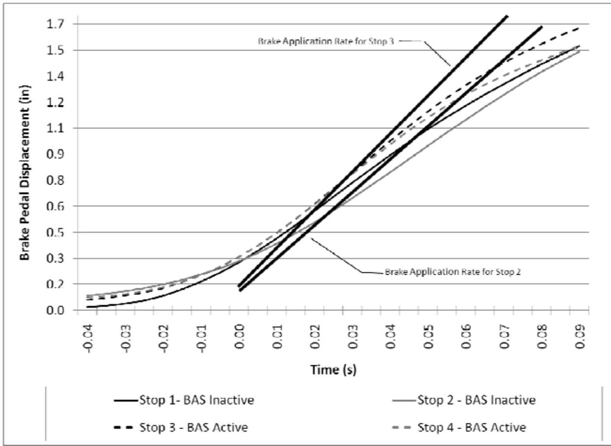
**Figure 21. Brake Application Rate for the Four Stops over the First 0.09 s**
