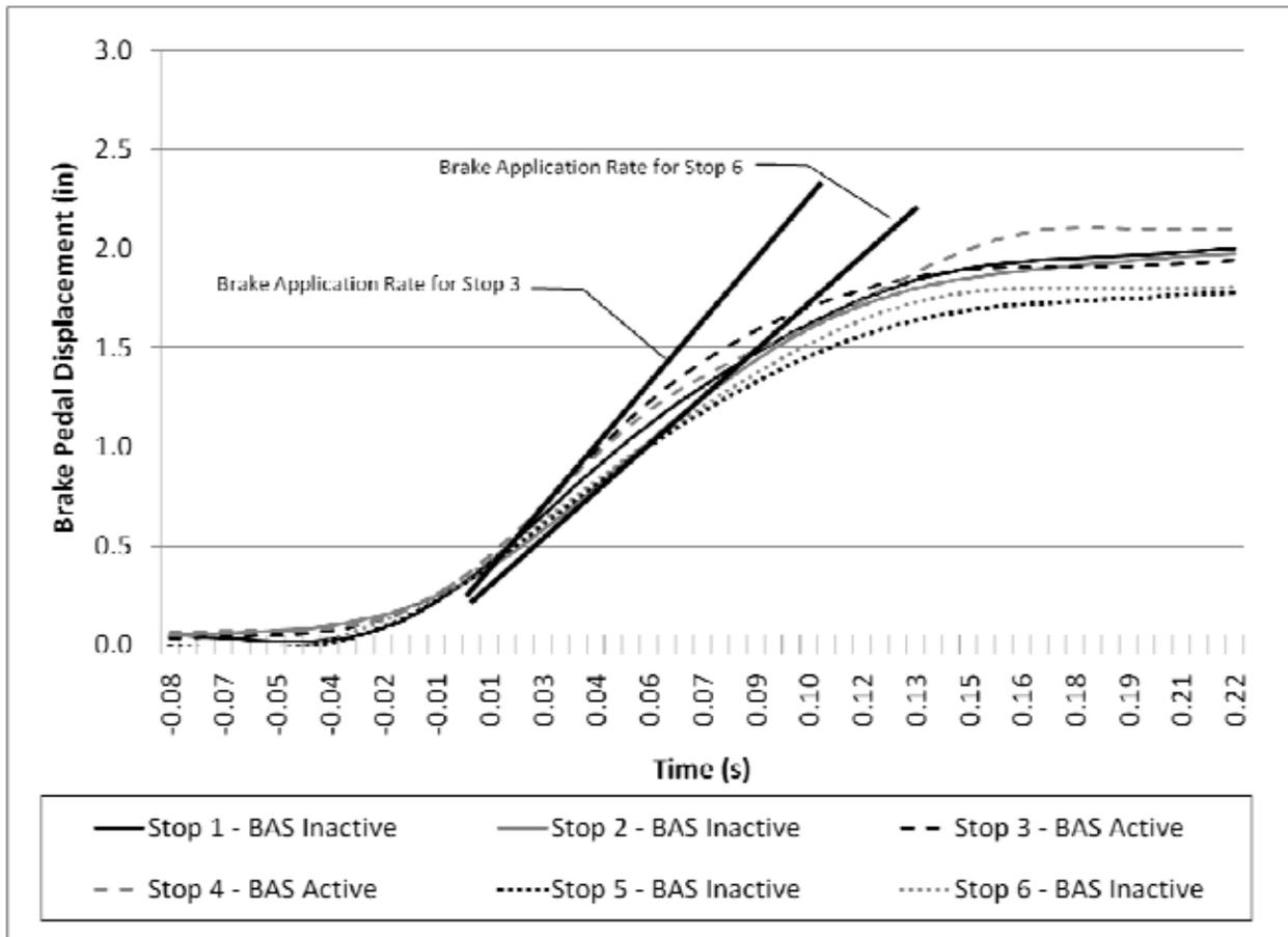
**Figure 24. The brake application rate for Stops 3 and 6 over the first 0.03 s.**
