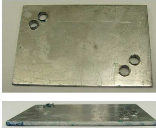
Figure 6.4: Adapter that enables ferrite core to be used in the spin coater.
