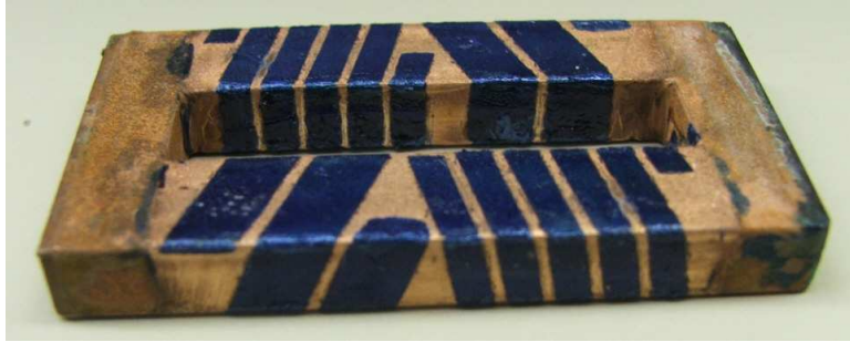
Figure 6.13: The core after applying the etch resist.
