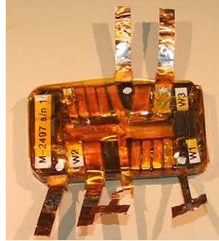
Figure 1.11: The transformer used for experimental verification of the models.
