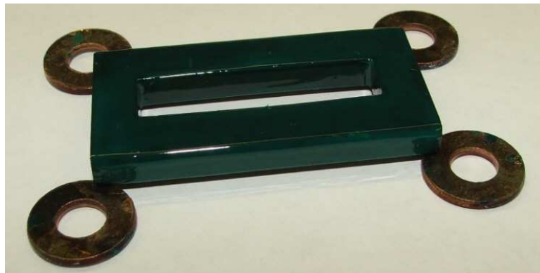
Figure 6.5: The core after applying solder mask.
