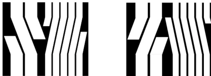
Figure 6.12: Photo mask used in UV exposure of the etch resist.
