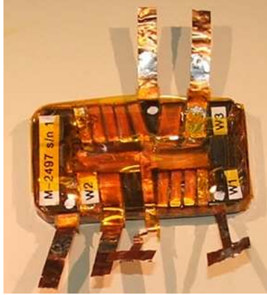
Figure 2.8: The transformer used for experimental verification of the models.
