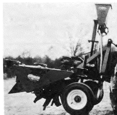
Figure 5. Power driven rototiller for the application of granular nematicides.
