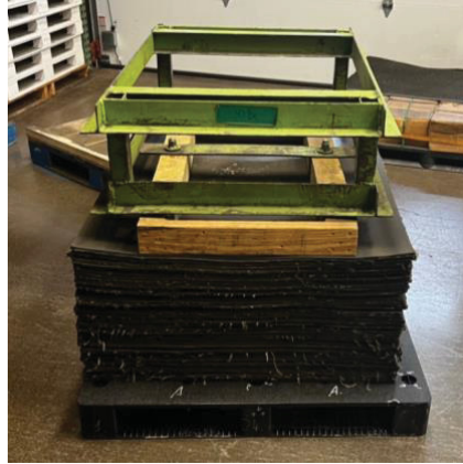
Figure 3.3: Simulated Unit Load Utilized for the FasTrack Simulation (1,500 lbs).
