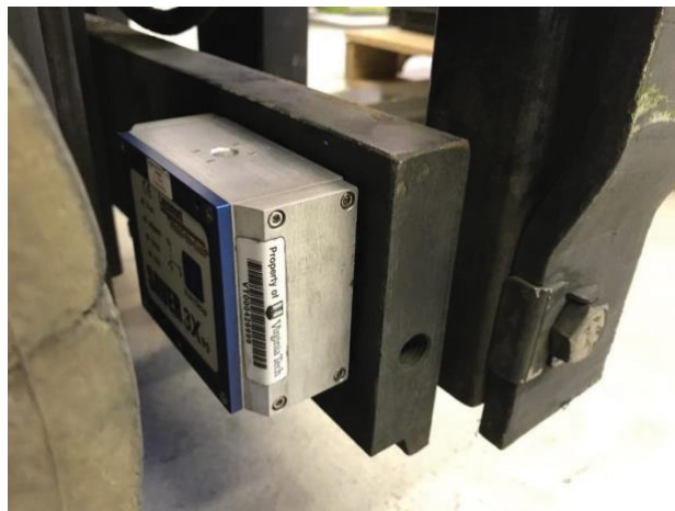
Figure 2.1: Location of Sensor of Fork Tine Carriage.
