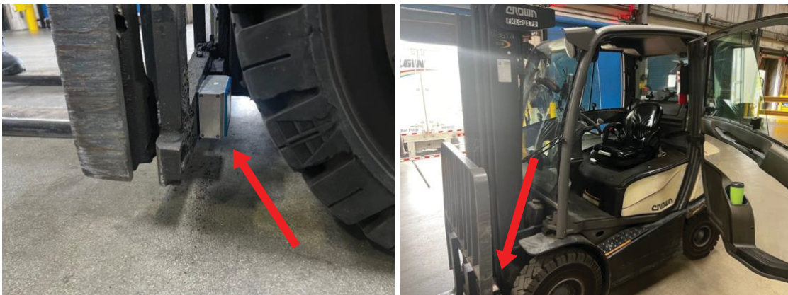
Figure 3.2: Sensor Placement for Field Data Collection.
