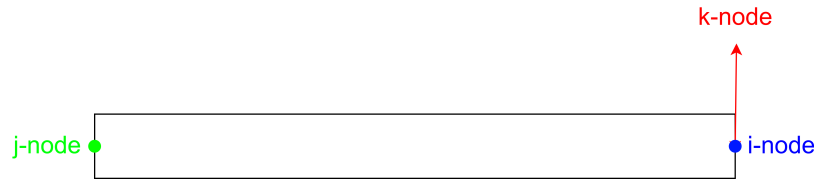
Figure 5.1: Diagram of Nodes for Beam Elements
