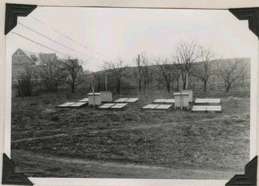
View of the eight electric hotbeds being studied. The small houses are for meters, switches and thermo- meters.
