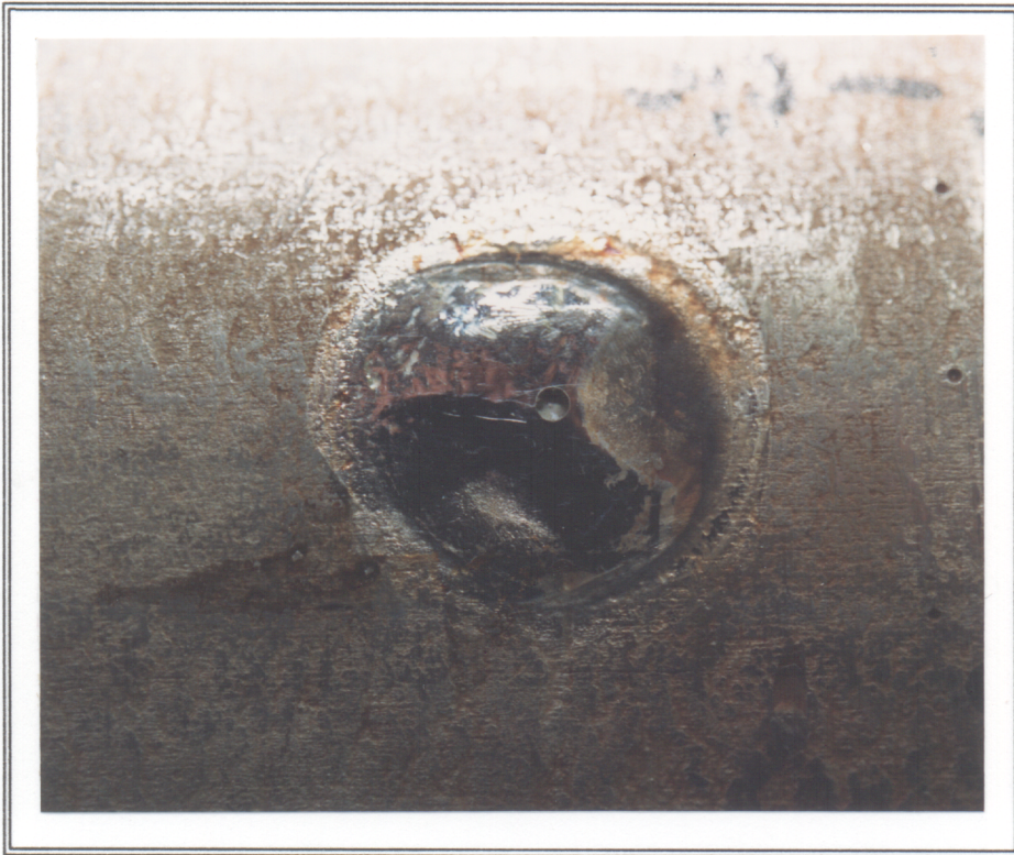
Figure 5-5 Electropolishing And Hole-drilling Site Electropolishing Hole Diameter Equals One Inch
