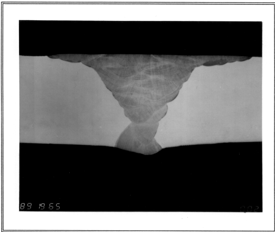
Figure 4-4 Transverse View Of The Weld And Wall Section Magnification Of Two
