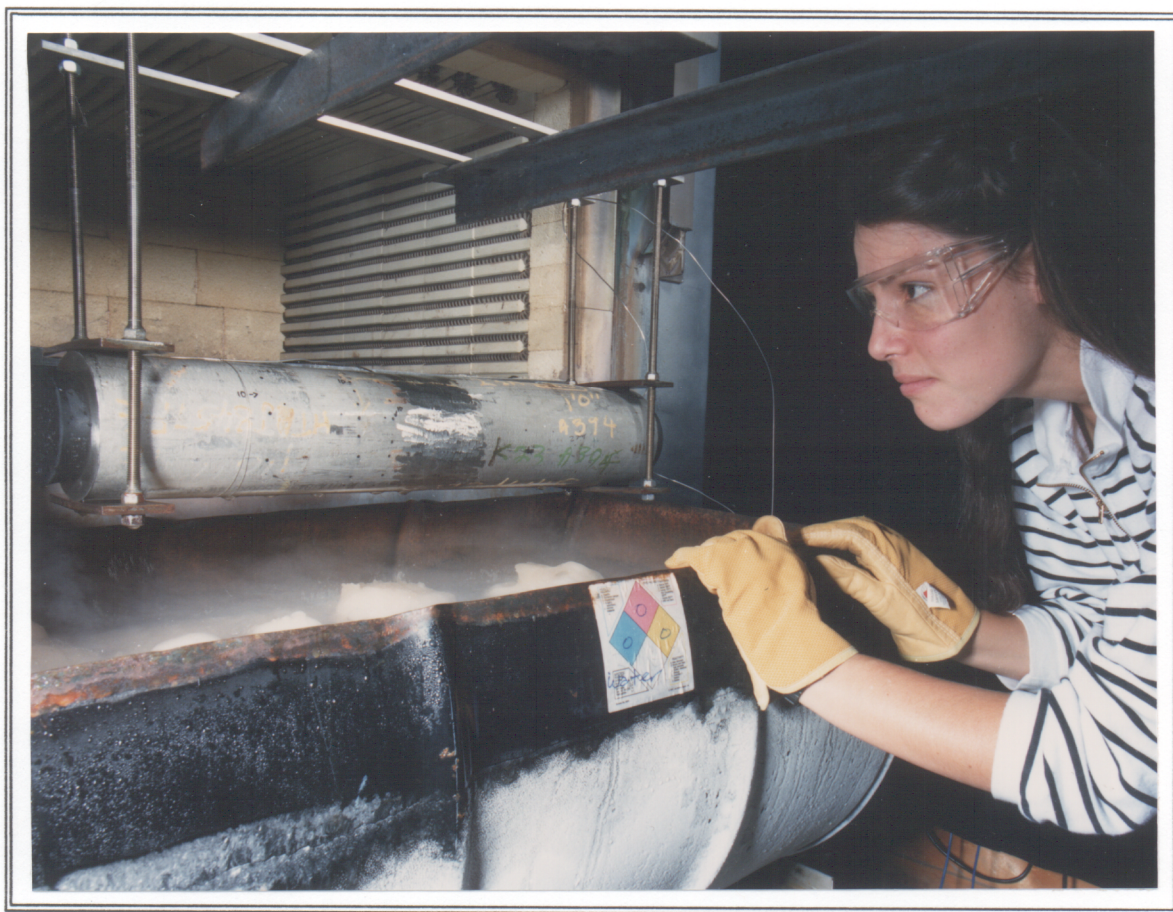
Figure 5-6 Apparatus Of The Thermal Cycling Process (ORNL)
