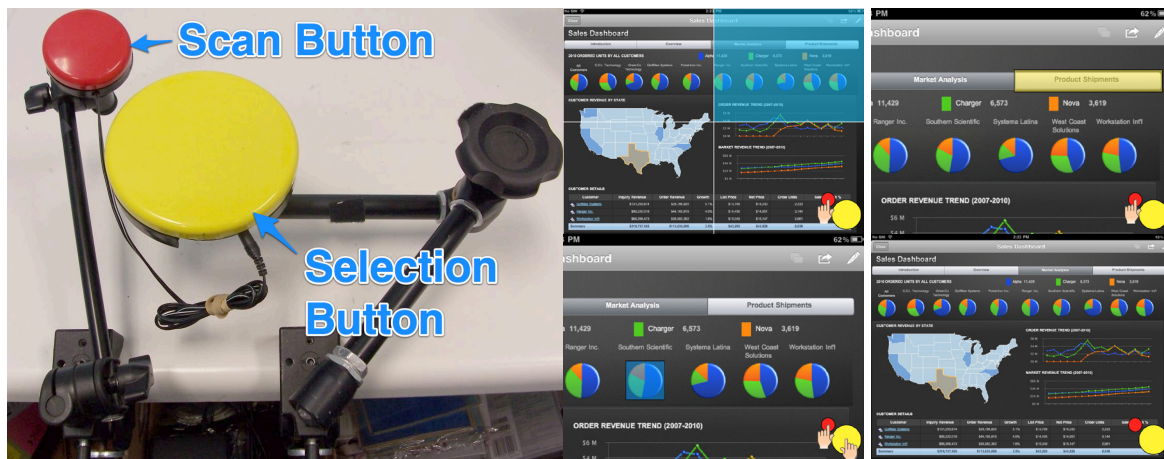
Figure 61 – Setup used for the switch interface and sequence of actions demonstrating the use of a progressive refinement technique combined with the switch interface in a tablet application.
