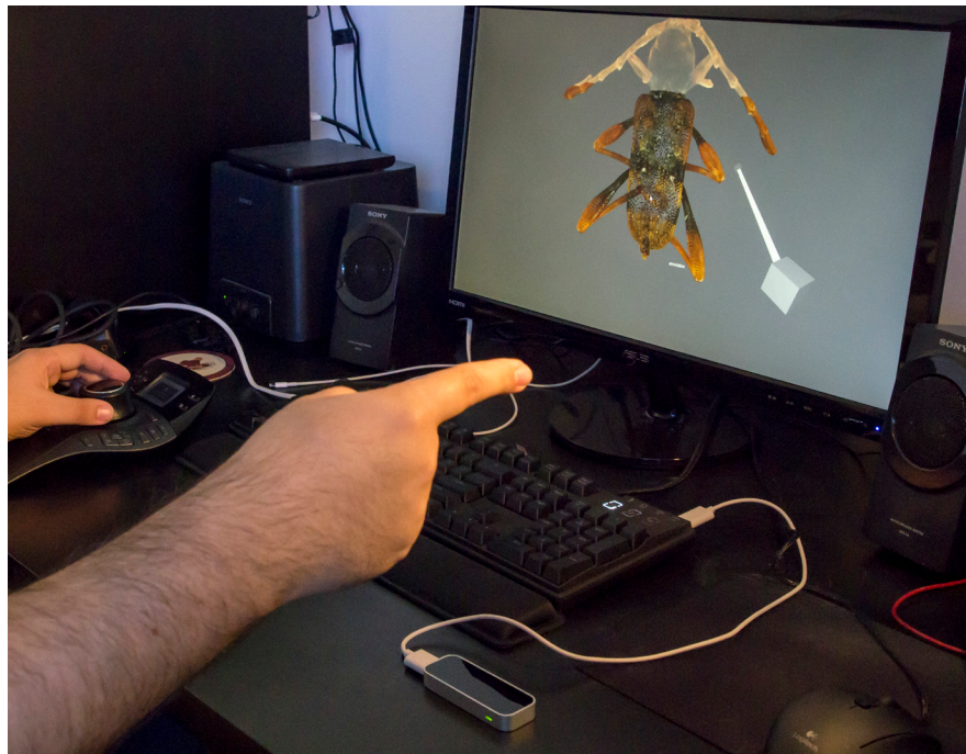
Figure 46 – Complete setup used in the evaluation of gesture-based progressive refinement techniques for point cloud selection.
