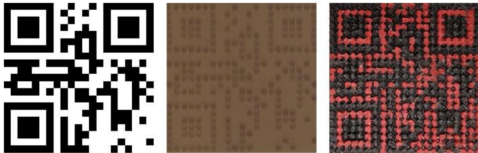
Figure 4.1. The a) original QR code and manufactured QR codes on b) powder bed fusion and c) material extrusion systems.
