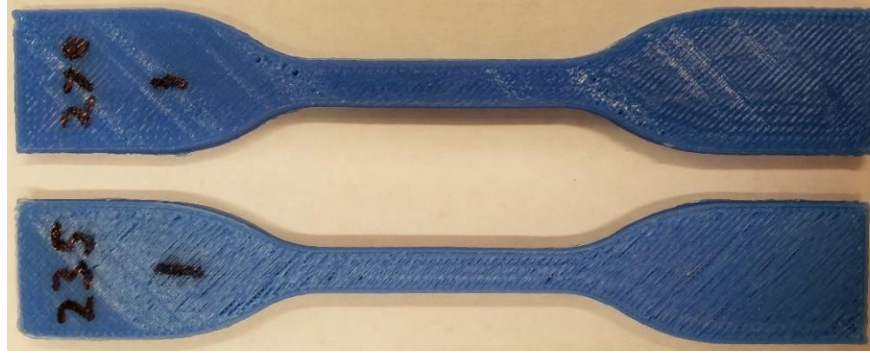
Figure 4.21. Comparison of samples manufactured at the low and high temperatures. The lower temperature part (bottom) under-extruded in places, resulting in a worse surface finish.
