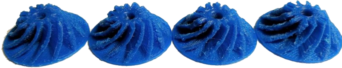
Figure 4.15. Images of the a) benchmark and three levels of fin base thickness changes: b) 1.25, c) 1.5, and d) 2 mm.
