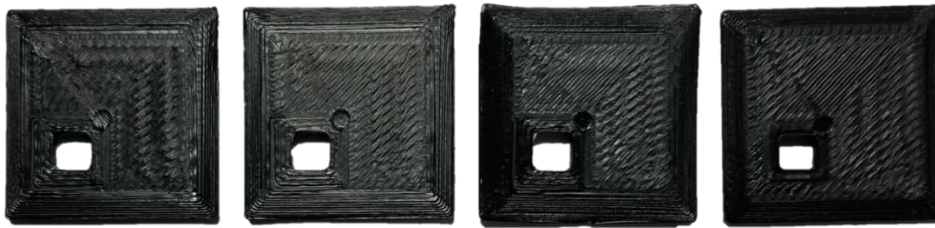
Figure 5.17. Image of the parts produced in the three experiments described above: a) no attack, b) attacked extrusion temperature, c) internal void attack, and d) perimeter count attack.
