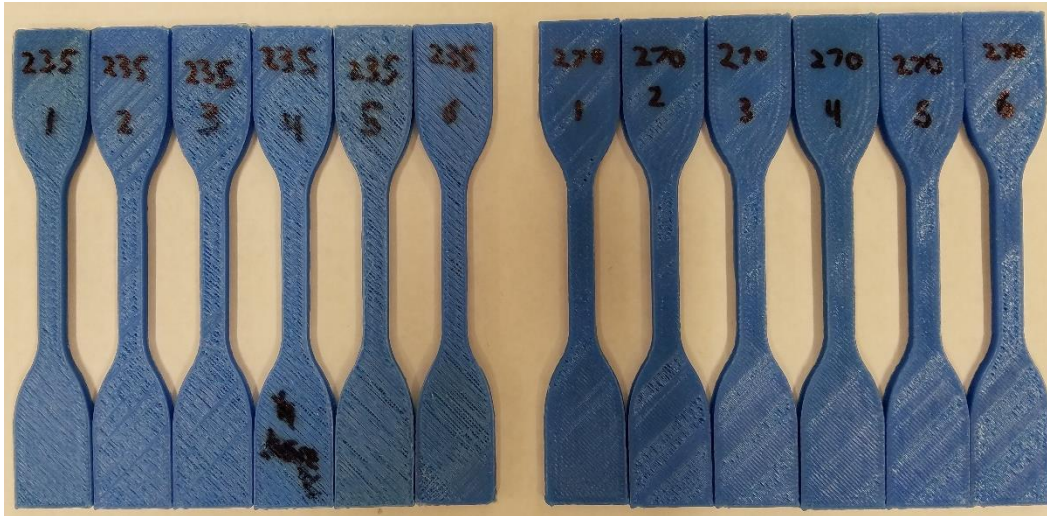
Figure 4.19. Tensile test specimens: a) low temp (235 °C) and b) high temp (270 °C).
