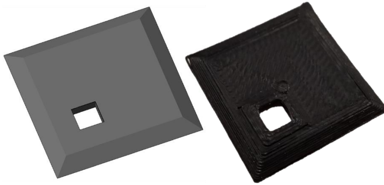
Figure 5.2. Test part used in the material extrusion implementation. The pyramid is 2 mm tall (10 layers) with a 30x30 mm base.
