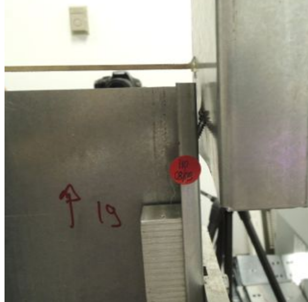
Picture 4.3.4.5.b. – Gap of a WF connection
