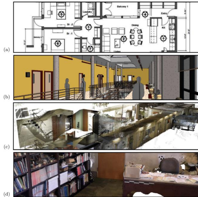
Figure 1: Different representations of indoor spaces including (a) Computer-Aided Drawing (CAD), (b) Building-Information Models (BIM), (c) Point-cloud, and (d) textured mesh. From Chen and Clarke (2019).
