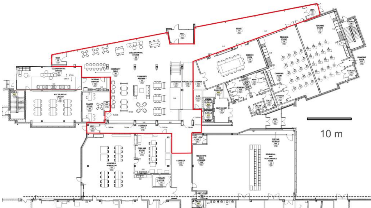
Figure 7: The ground-floor of the Community Assembly space of the CID at Virginia Tech. The extent of lidar data collection is outlined in red.
