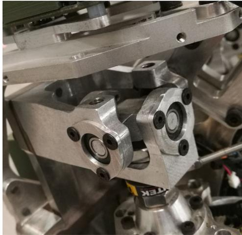
Figure 2.6: The universal joints on humanoid robots in TREC lab
