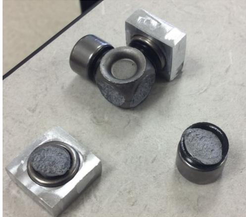
Figure 2.9: A failed universal joint.
