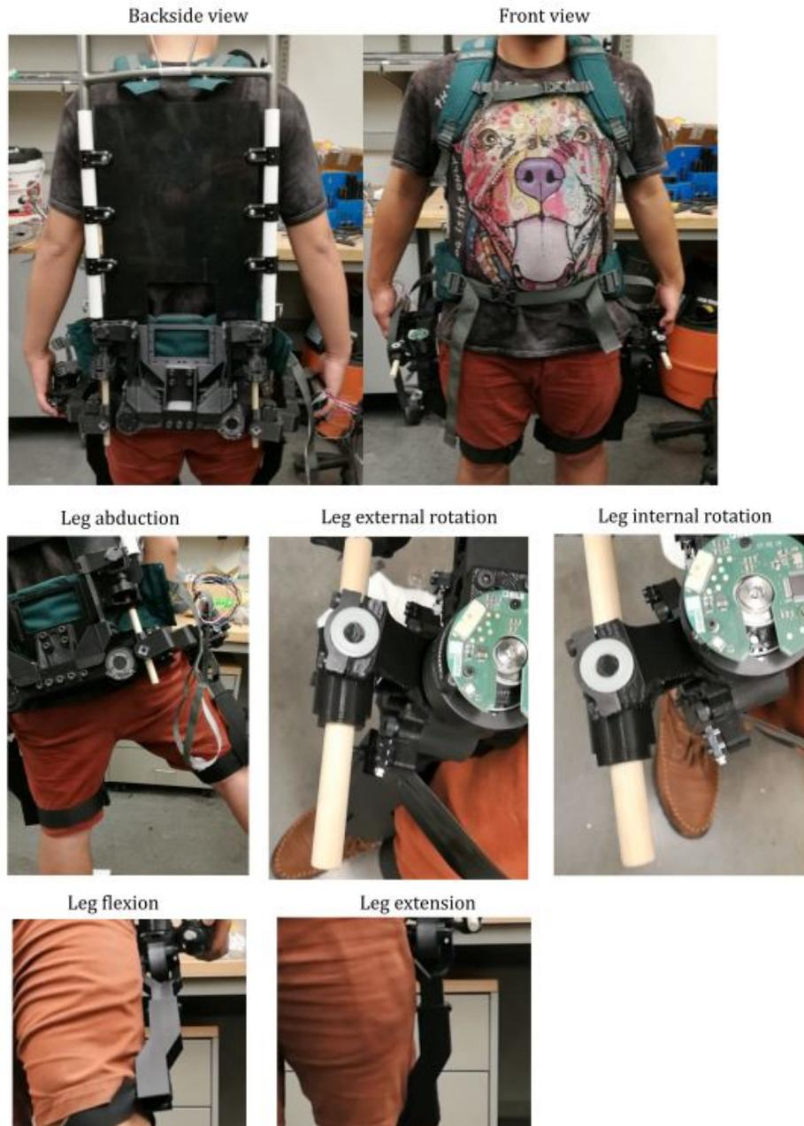
Figure 5.20: Experiments with wearing the 3D printed prototype.
