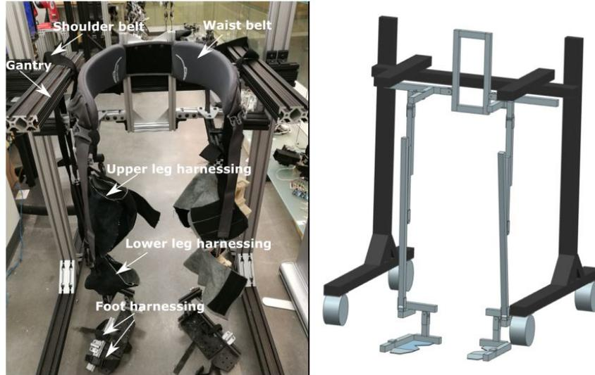
Figure 3.7: Prototype of 12-DoF lower-body exoskeleton.
