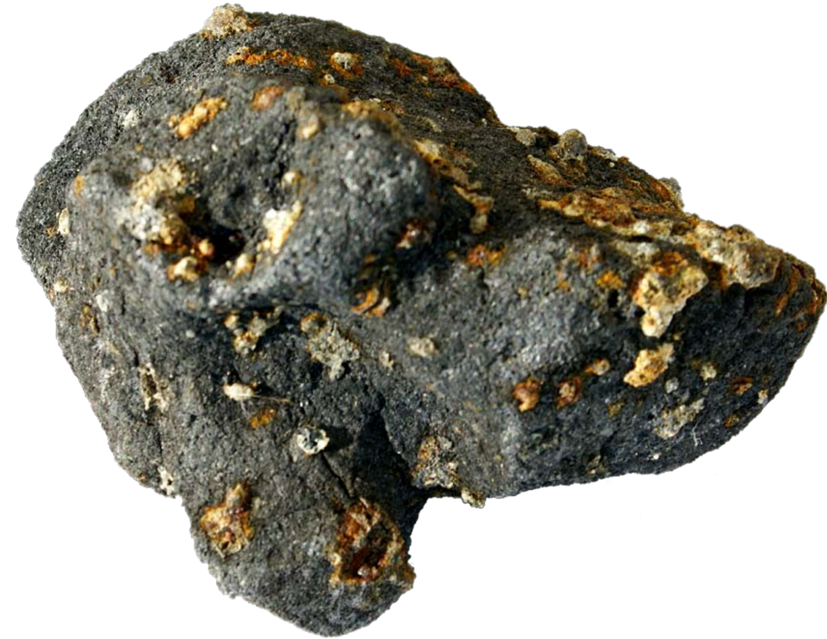
Coke [left] burns at a specific temperature to ensure raw metal melts evenly. Slag [right] is unusable metallic left-over from a pour.
