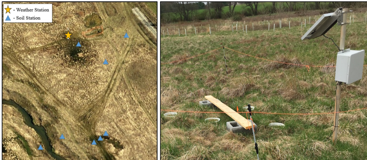
Figure B-2. (a) Locations of all soil sensor stations in the floodplain. (b) Soil moisture station at the active floodplain site.
