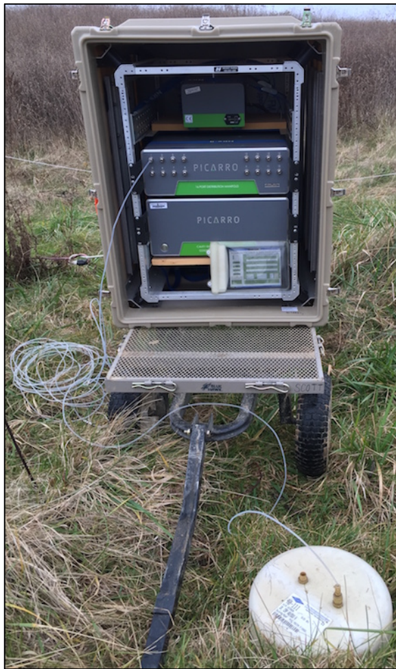
Figure B-1. Image of the Picarro G2508 with cap attachment installed in the transportable box and strapped to a utility cart. Shown with operating tablet in waterproof case.
