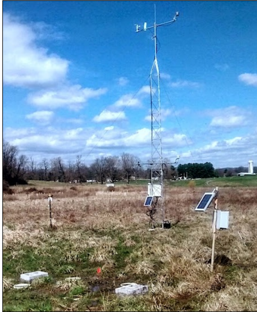
Figure 2-2-3. Image depicting the four collars and solar panel station containing the data logger connected to the Decagon 5TM sensor installed at the Convergence site, and the StREAM Lab meteorological tower with rain gauge. The Decagon 5TM sensor location is marked by an orange field flag.
