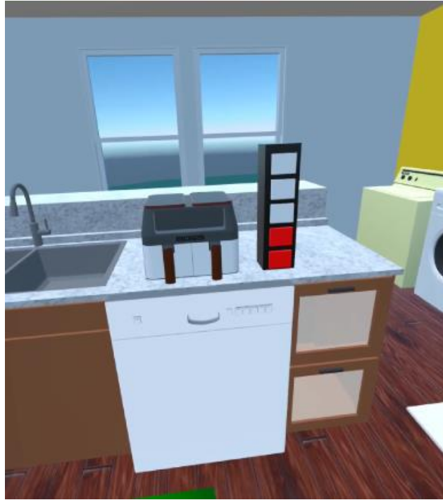
Figure 23: Displays the power meter visual aid, showing five levels of energy consumption indicated by the number of red blocks lit.
