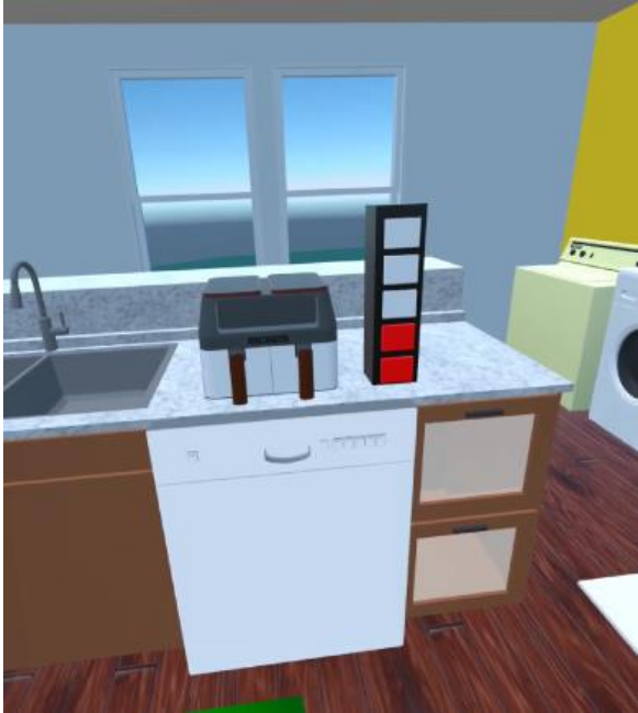
Figure 17: Displays the power meter visual aid, showing five levels of energy consumption indicated by the number of red blocks lit.
