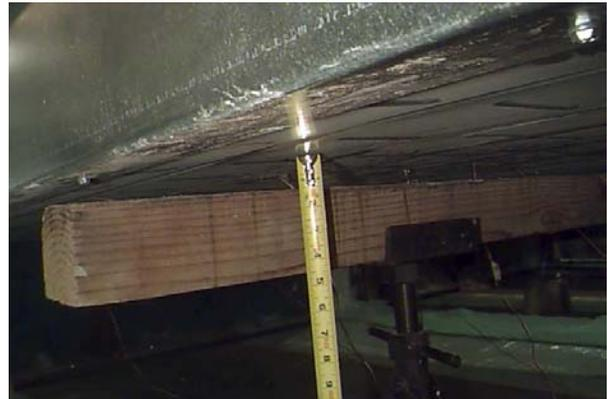
**Figure 5.21 – Typical Close-Up View of Camber of Series III Continuous Specimen**
