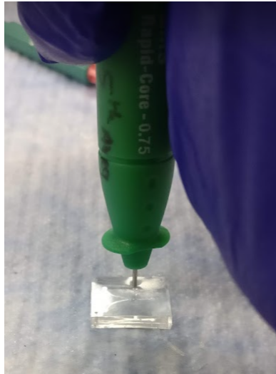
Figure 5.16: Inlet and outlet holes for connecting 30 gauge tubing punched with a 0.75 mm biopsy punch
