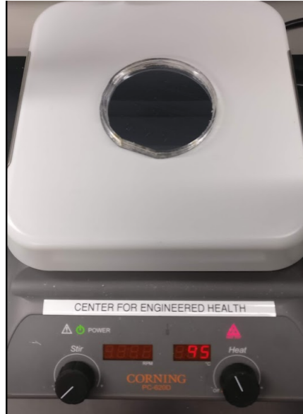
Figure 5.7: Silicon wafer with 10:1 PDMS placed on a hotplate for curing the mixture
