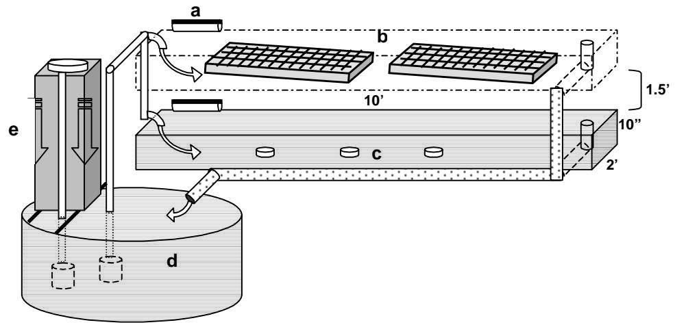
**Figure 3.1.** Larval rearing system: **a**- fry collection lamp, **b**- egg ribbon screens, **c**- internal light niches, **d**- reservoir sump, **e**- packed column trickling filter.
