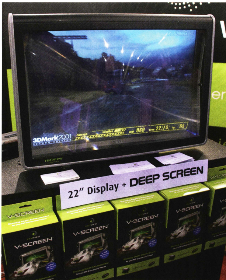
Above: The "Deep Screen" setup put a layer over top of a standard display to add depth to the application that was running. The demoed racing game felt far more immersive.
