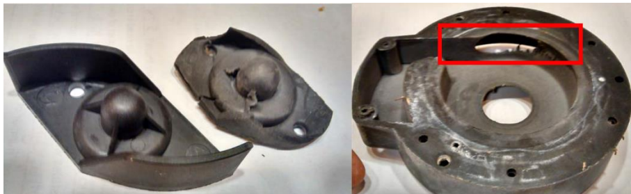
Figure 2-19. (left) new impeller compared to damaged impeller in system with large particles, (right) representative hole in plastic pump housing.
