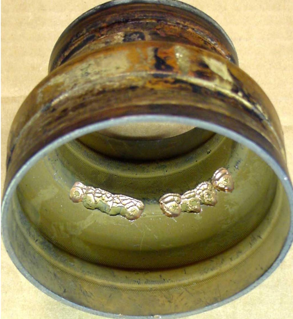
Figure 1-18. Pipe from a Real Premise Plumbing System Exhibiting Possible Cavitation Bubble Implosion Damage
