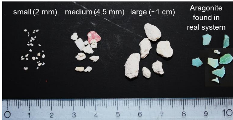
Figure 2-10. Representative aragonite particles used in experiments alongside particles found in Building X's plumbing
