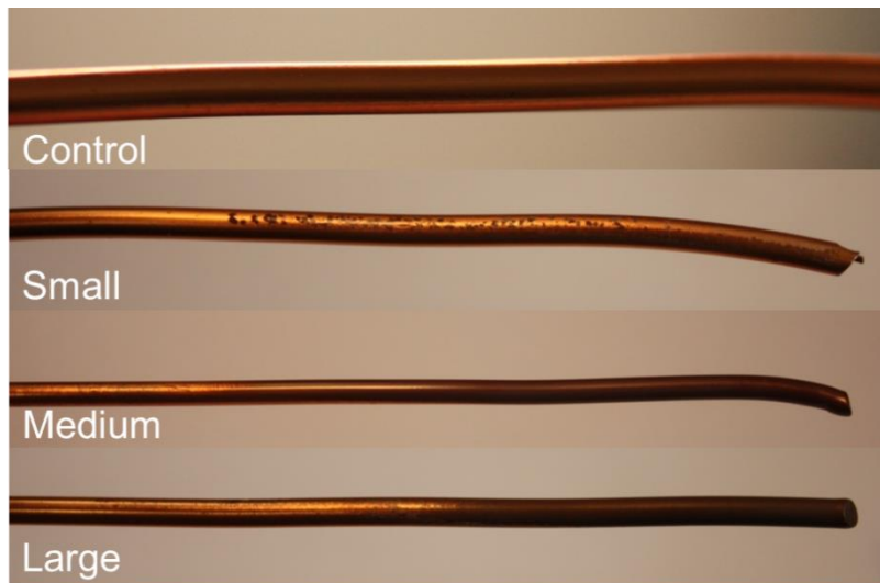
Figure 2-30. Close-up photos of copper wires showing worst erosion corrosion attack w.r.t. increase in particle size
