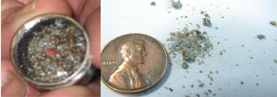
Figure 2-4. Very hard particulates clogged aerators (left) with very abrasive and highly crystalline calcium carbonate particulates (right). Particles on right represent only a portion of those actually present in the aerator.
