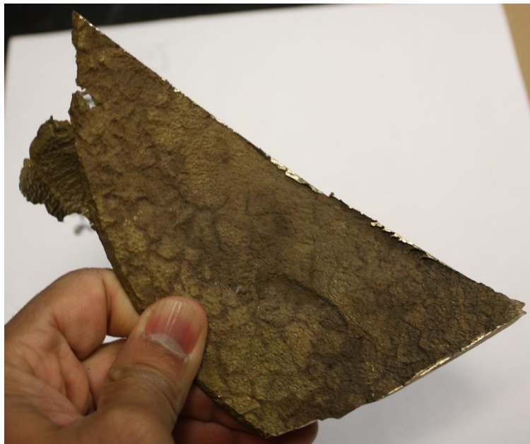
Figure 4-1. Pump impeller section (low-zinc silicon bronze) that witnessed extensive short-term damage while in service
