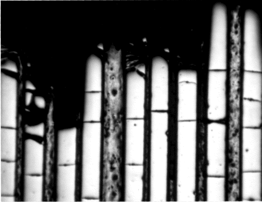
Figure 9a. Cross-section of boron-aluminum composite near fracture showing type I fiber breaks. T6N heat treatment. Magnification 50x.
