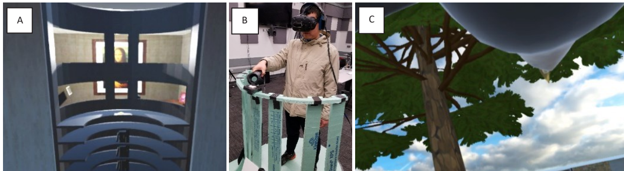
Figure 3-1: The bookshelf and bird techniques. A) The bookshelf uses a virtual rotation to allow the user to proceed to an adjacent room; B) The user standing on the physical prop and touching the button that activates the Bookshelf redirection; C) The bird translates the user to another cell while maintaining the correct relationship between the user, the physical workspace, and the virtual cell.
