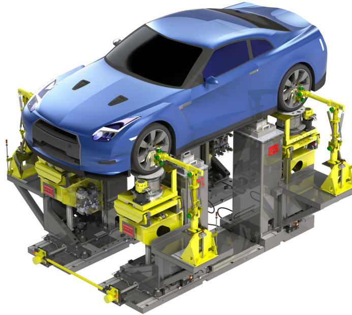
Figure 1.2: MTS Systems' K&C Deflection Measurement System [88]
