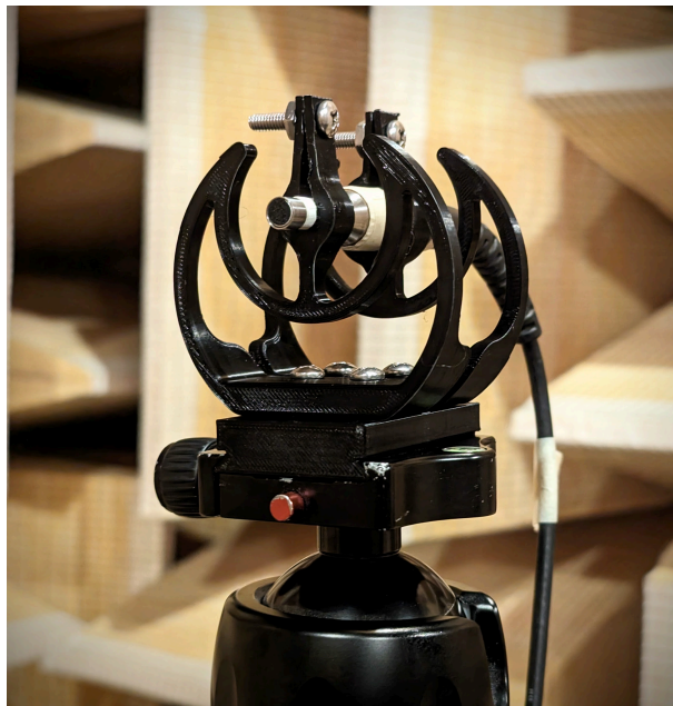
Figure 7.3: PCB Piezotronics Model 130D20 microphone mounted top tripod ball-head
