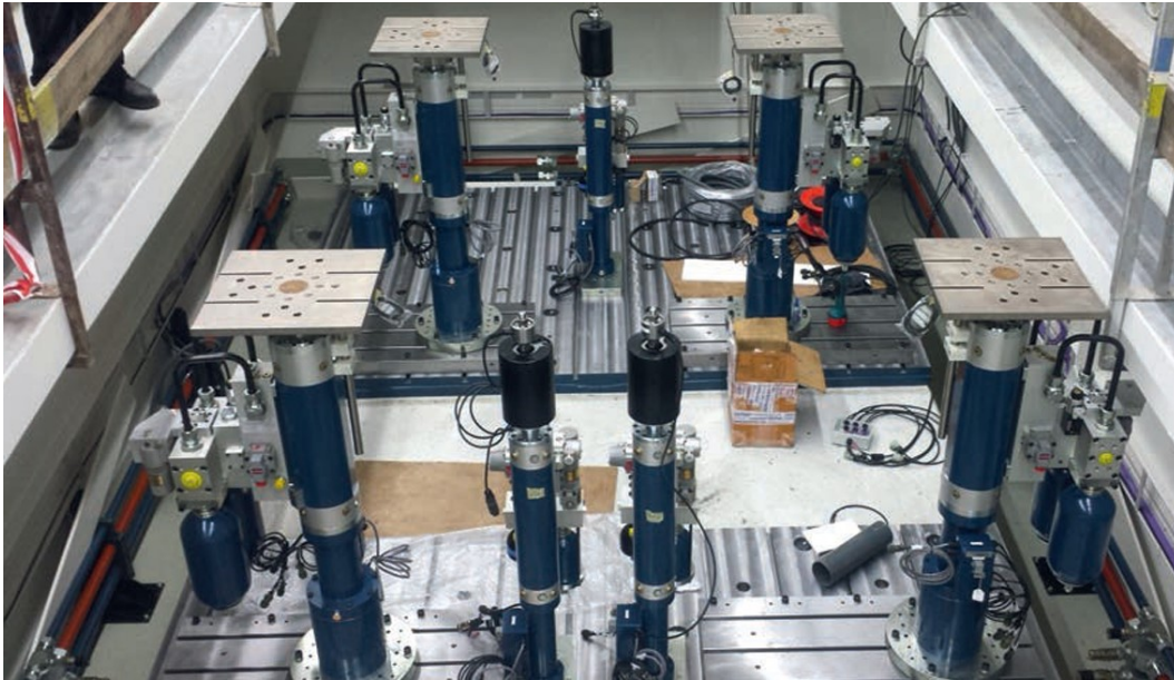
Figure 1.3: The Servotest 7-post Vehicle Ride Simulator used by TRE [40]
