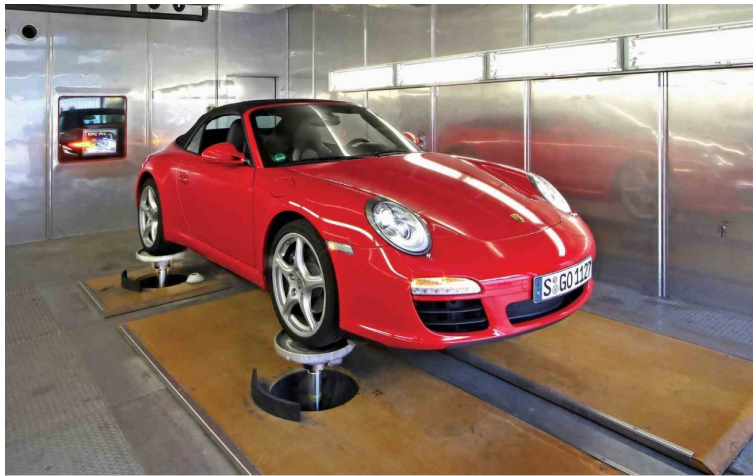
Figure 1.1: MTS Systems' Model 320 Tire-coupled Road Simulator [89]
