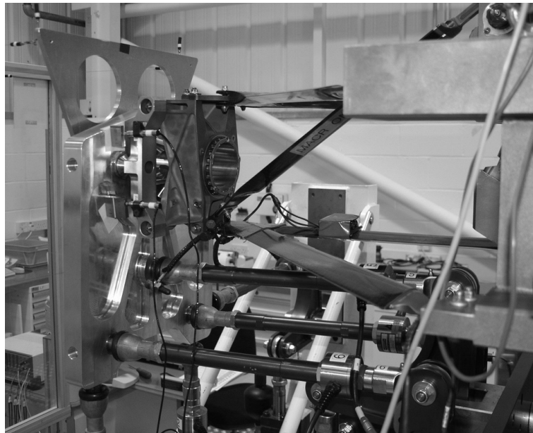
Figure 1.5: Multi-DOF Suspension Test rig used by Formula 1 Teams [73]
