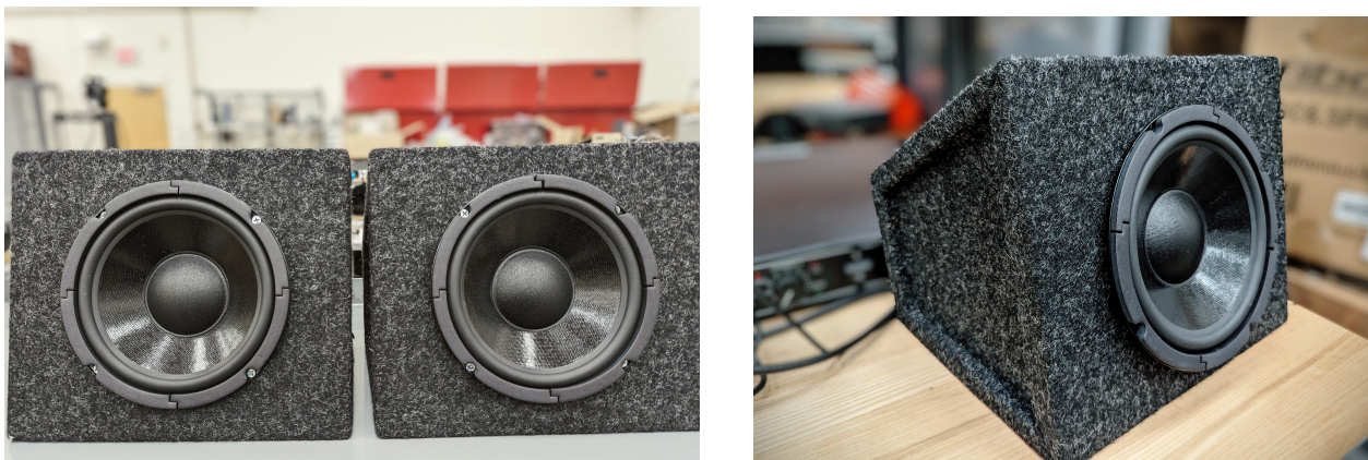
Figure 7.2: Pair of woofer drivers used as speakers secured in their enclosures
