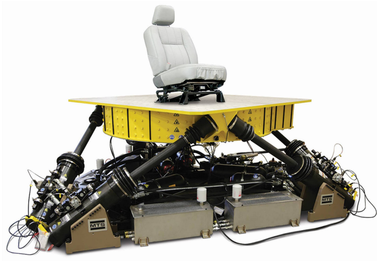
Figure 1.6: MTS Systems' Multi-Axial Simulation Table (MAST) system [90]
