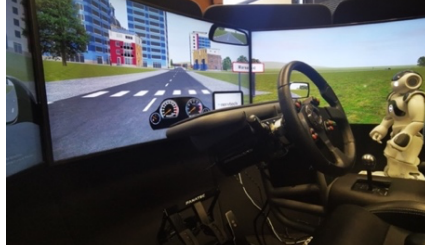
Figure 1. Experimental setup with the NervTech driving simulator and Nao.
